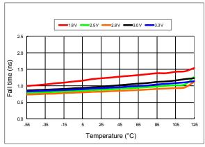
Figure 12. 20%-80% Fall Time vs Temperature
