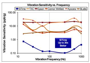
Figure 5. Vibration Robustness<sup>[5]</sup>
