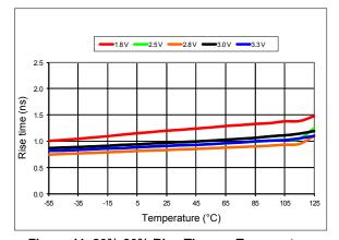
Figure 11. 20%-80% Rise Time vs Temperature
