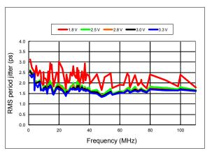
Figure 9. RMS Period Jitter vs Frequency
