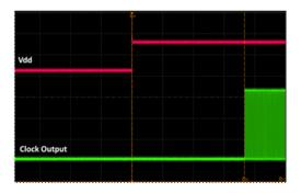
Figure 16. Startup Waveform vs. Vdd
