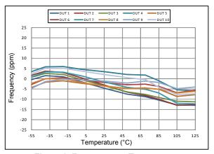
Figure 8. Frequency vs Temperature
