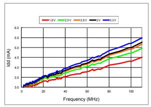
Figure 7. Idd vs Frequency
