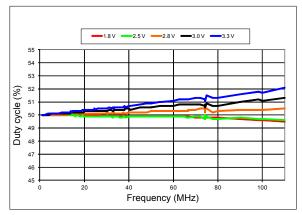
Figure 10. Duty Cycle vs Frequency
