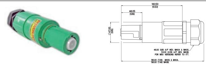
Line Drain is the connector with a female contact which is not normally the live part, however they are fitted with a spring loaded plastic cap that prevents accidental finger touching of the contact, and the connector meets IP2X requirements. Contacts are available to suit cable conductors from 25mm<sup>2</sup> to 300mm<sup>2</sup>.
