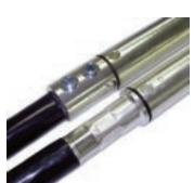
Cable glands meeting IP67 requirements are fitted to the connectors, 4 sizes are available that cover a range of cables with outside diameters from 15mm to 38mm. When selecting the M50 gland, please note that this is supplied with an adaptor (not shown above) that steps the connector up from M40 to M50.
