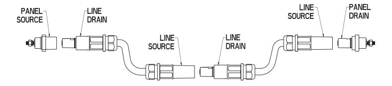
PowerLock connectors feature a bayonet coupling mechanism with a secondary locking pin. When a pair of connectors are mated and fully turned to engage the bayonet, the spring loaded secondary locking pin on the Drain connectors, snaps into a slot on the Source connector; a special release key is then required to uncouple the connectors.
