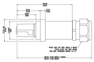
These connectors are supplied with a loose female contact that is fitted to the cable before being assembled into the connector housing.
