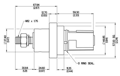
Panel Drain connectors are supplied fully assembled with the female contact having an M12 threaded post, with nut and spring washer for connection to a standard cable lug. These connectors rated either 400 amp (T4) or 660 amp (T6). This connector is fitted with the secondary locking pin for secure connections, see explanation on Line Drain page 13.
