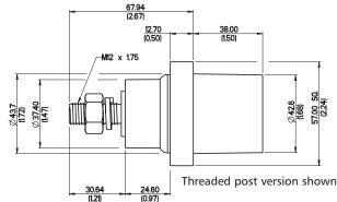
Panel Source connectors are supplied fully assembled with the male contact having an M12 threaded post, with nut and spring washer for connection to a standard cable lug, or M12 threaded hole for fixing with a bolt. These connectors are rated either 400 amp (T4 / H4) or 660 amp (T6 / H6).
