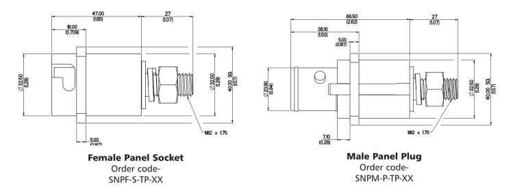
The standard panel connectors are mounted through 4 holes in the flange. The rear of the connector has an M12 threaded post fitted with a nut and lock washer, to take a cable fitted with a standard cable lug. Male and female connectors are available in a range of colors, and all panel connectors are fitted with a gasket.
