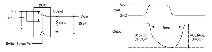
Figure 2. t<sub>BBM</sub> (Time Break-Before-Make)
