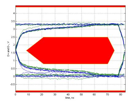
Figure 11. Full Speed Signal Quality Eye Diagram Test (NLAS7222A with  $V_{CC}$  = 3.6 V)
