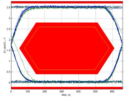
Figure 10. Low Speed Signal Quality Eye Diagram Test (NLAS7222A with V<sub>CC</sub> = 3.6 V)
