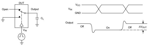
Figure 6. Charge Injection: (Q)
