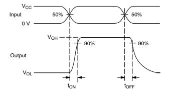
Figure 3. t<sub>ON</sub>/t<sub>OFF</sub>
