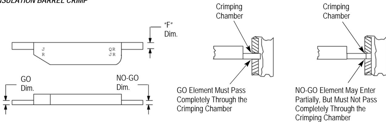
**SUGGESTED PLUG GAGE DESIGN FOR WIRE BARREL CRIMP**
