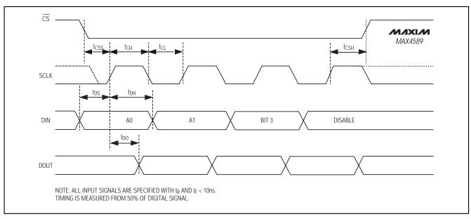
Figure 7. Serial Timing Diagram
