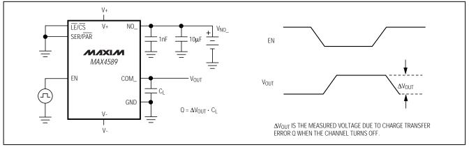
Figure 3. Charge Injection
