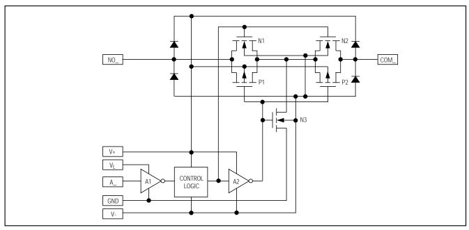
Figure 8. T-Switch Construction
