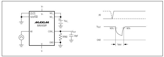
Figure 2. Break-Before-Make Time Delay
