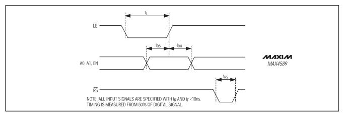
Figure 6. Parallel Timing Diagram
