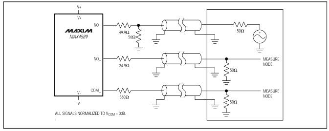
Figure 5. Off-Isolation, Crosstalk, and Bandwidth
