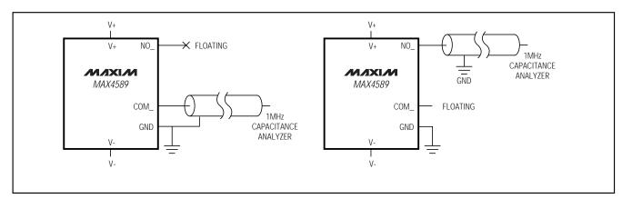
Figure 4. NO\_, COM\_ Capacitance
