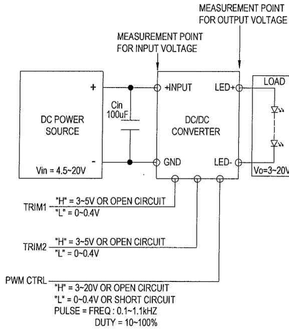
IN APPLICATIONS WHERE POWER IS SUPPLIED OVER LONG LINES AND OUTPUT LOADING IS HIGH, IT IS RECOMMENDED TO USE A GOOD QUALITY LOW EQUIVALENT SERIES RESISTANCE (ESR<1.0Ω AT 100kHz) CAPACITOR WITH 100uF CAPACITANCE FOR THE MODULE.
