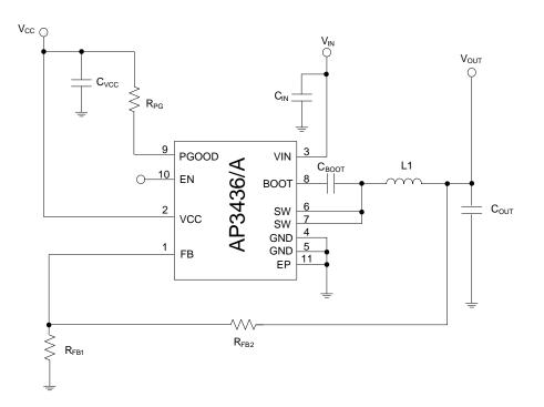
Note 4: When using a single power supply for  $V_{CC}$  and  $V_{IN}$ , a 4.7 $\Omega$  resistor should be placed between them for noise isolation.
