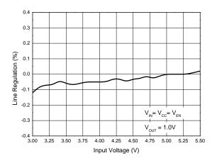
Line Regulation vs. Input Voltage
