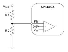
Figure 1. Voltage Divider Circuit
