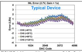
FIGURE 1-66: INL Error vs. DAC Code, and Temperature (Code 100 - 4000) (Single Channel - MCP48FXB21) (12-bit:  $V_{DD} = 2.7V$ , VRxB:VRxA = '01' (Bandgap), Gx = '0' (1x)).
