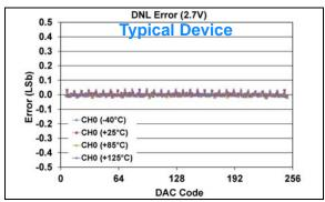
**FIGURE 1-557:** DNL Error vs. DAC Code, and Temperature (Code 6 - 250) (Single Channel - **MCP48FXB01**) (8-bit:  $V_{DD} = 2.7V$ ,  $V_{REF} = 1V$ ,  $V_{RXB}:V_{RXA} = '11'$  ( $V_{REF}$  Buffered),  $G_{X} = '1'$  ( $Z_{X}$ ).
