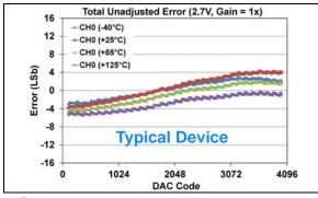
**FIGURE 1-60:** Total Unadjusted Error  $(V_{OUT})$  vs. DAC Code, and Temperature (Single Channel - **MCP48FXB21**)  $(12\text{-bit}: V_{DD} = 2.7V, VRxB:VRxA = '01' (Bandgap), Gx = '0' (1x)).$
