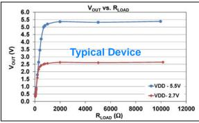
**FIGURE 1-36:** V<sub>OUT</sub> vs. R<sub>LOAD</sub> and Voltage (at +25°C).
