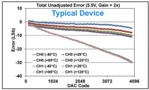
**FIGURE 1-133:** Total Unadjusted Error  $(V_{OUT})$  vs. DAC Code, and Temperature (Dual Channel - **MCP48FXB22**) (12-bit:  $V_{DD} = 5.5V$ ,  $V_{REF} = 2.048V$ ,  $VRxB:VRxA = '10' (V_{REF} Unbuffered)$ , Gx = '1' (2x)).
