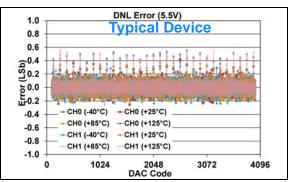
**FIGURE 1-181:** DNL Error vs. DAC Code, and Temperature (Code 100 - 4000) (Dual Channel - **MCP48FXB22**) (**12-bit**:  $V_{DD} = 5.5V$ ,  $V_{REF} = 1V$ , VRxB:VRxA = '11' ( $V_{RFF}$  Buffered), Gx = '0' (1x)).
