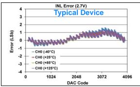
FIGURE 1-155: INL Error vs. DAC Code, and Temperature (Code 100 - 4000) (Single Channel - MCP48FXB21) (12-bit:  $V_{DD} = 2.7V$ ,  $V_{REF} = V_{DD}$ ,  $VRxB:VRxA = '11' (V_{REF} Buffered)$ , Gx = '0' (1x)).
