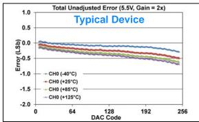
**FIGURE 1-490:** Total Unadjusted Error  $(V_{OUT})$  vs. DAC Code, and Temperature (Single Channel - **MCP48FXB01**) (8-bit:  $V_{DD} = 5.5V$ ,  $V_{REF} = 2.048V$ ,  $VRxB:VRxA = '10' (V_{REF} Unbuffered)$ , Gx = '1' (2x)).
