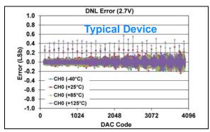
**FIGURE 1-53:** DNL Error vs. DAC Code, and Temperature (Code 100 - 4000) (Single Channel - **MCP48FXB21**) (12-bit:  $V_{DD} = 2.7V$ ,  $VRxB:VRxA = '00' (V_{DD})$ , Gx = '0' (1x)).
