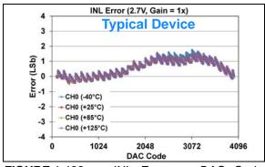
FIGURE 1-138: INL Error vs. DAC Code, and Temperature (Code 100 - 4000) (Single Channel - MCP48FXB21) (12-bit:  $V_{DD} = 2.7V$ ,  $V_{REF} = 2.048V$ ,  $VRxB:VRxA = '10' (V_{REF} Unbuffered)$ , Gx = '0' (1x)).
