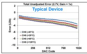
**FIGURE 1-384:** Total Unadjusted Error  $(V_{OUT})$  vs. DAC Code, and Temperature (Single Channel - **MCP48FXB11**)  $(10\text{-bit}: V_{DD} = 2.7V, V_{REF} = 2.048V, VRxB:VRxA = '11' (V_{REF} Buffered), Gx = '0' (1x)).$
