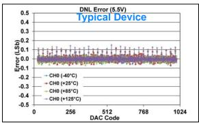
**FIGURE 1-304:** DNL Error vs. DAC Code, and Temperature (Code 25 - 1000) (Single Channel - **MCP48FXB11**) (10-bit:  $V_{DD} = 5.5V$ ,  $V_{REF} = 1V$ ,  $V_{RXB}:V_{RXA} = '10'$  ( $V_{RFF}$  Unbuffered),  $G_{X} = '1'$  ( $Z_{X}$ ).
