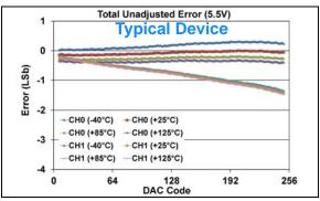
**FIGURE 1-547:** Total Unadjusted Error  $(V_{OUT})$  vs. DAC Code, and Temperature (Dual Channel - **MCP48FXB02**) (8-bit:  $V_{DD} = 5.5V$ ,  $V_{REF} = 1V$ ,  $V_{RXB}:V_{RXA} = '11'$   $(V_{REF} Buffered)$ ,  $G_{X} = '1'$  (2x)).
