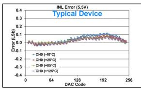
**FIGURE 1-478:** INL Error vs. DAC Code, and Temperature (Code 6 - 250) (Single Channel - **MCP48FXB01**) (8-bit:  $V_{DD} = 5.5V$ ,  $V_{REF} = 1V$ ,  $V_{RXB}:V_{RXA} = '10'$  ( $V_{REF}$  Unbuffered),  $G_{X} = '1'$  (2x)).
