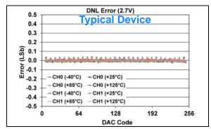
FIGURE 1-560: DNL Error vs. DAC Code, and Temperature (Code 6 - 250) (Dual Channel - MCP48FXB02) (8-bit:  $V_{DD} = 2.7V$ ,  $V_{REF} = 1V$ ,  $V_{RXB}$ :  $V_{RXA} = '11'$  ( $V_{REF}$  Buffered),  $G_{X} = '1'$  ( $V_{REF}$  Buffered).
