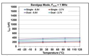
**FIGURE 1-14:** Average Device Supply Current - Active Interface ( $I_{DDA}$ ) ( $F_{SCK} = 1$  MHz) vs. Voltage and Temperature, VRxB:VRxA = '01' (Bandgap mode).
