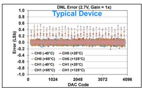
FIGURE 1-147: DNL Error vs. DAC Code, and Temperature (Code 100 - 4000) (Dual Channel - MCP48FXB22) (12-bit:  $V_{DD} = 2.7V$ ,  $V_{REF} = 2.048V$ ,  $VRxB:VRxA = '10' (V_{REF} Unbuffered)$ , Gx = '0' (1x)).
