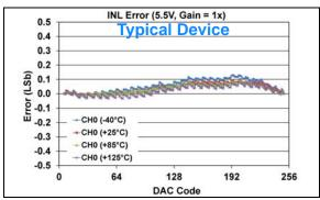
FIGURE 1-425: INL Error vs. DAC Code, and Temperature (Code 6 - 250) (Single Channel - MCP48FXB01) (8-bit:  $V_{DD} = 5.5V$ , VRxB:VRxA = '01' (Bandgap), Gx = '0' (1x)).
