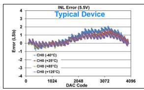
FIGURE 1-118: INL Error vs. DAC Code, and Temperature (Code 100 - 4000) (Single Channel - MCP48FXB21) (12-bit:  $V_{DD} = 5.5V$ ,  $V_{REF} = 1V$ , VRxB:VRxA = '10' ( $V_{RFF}$  Unbuffered), Gx = '1' (2x)).
