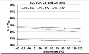
**FIGURE 1-29:** Average  $V_{IL}$  (SDI, SCK,  $\overline{CS}$ , and  $\overline{LAT}$  pins) vs. Voltage and Temperature.
