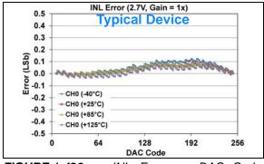
**FIGURE 1-426:** INL Error vs. DAC Code, and Temperature (Code 6 - 250) (Single Channel - **MCP48FXB01**) (8-bit:  $V_{DD} = 2.7V$ , VRxB:VRxA = '01' (Bandgap), Gx = '0' (1x)).
