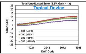
**FIGURE 1-59:** Total Unadjusted Error  $(V_{OUT})$  vs. DAC Code, and Temperature (Single Channel - **MCP48FXB21**) (12-bit:  $V_{DD} = 5.5V$ , VRxB:VRxA = '01' (Bandgap), Gx = '0' (1x)).
