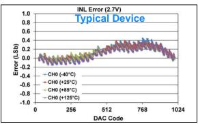
**FIGURE 1-353:** INL Error vs. DAC Code, and Temperature (Code 25 - 1000) (Single Channel - **MCP48FXB11**) (10-bit:  $V_{DD} = 2.7V$ ,  $V_{REF} = 1V$ , VRxB:VRxA = '11' ( $V_{REF}$  Buffered), Gx = '0' (1x)).
