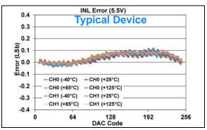
**FIGURE 1-463:** INL Error vs. DAC Code, and Temperature (Code 6 - 250) (Dual Channel - **MCP48FXB02**) (8-bit:  $V_{DD} = 5.5V$ ,  $V_{REF} = 1V$ ,  $V_{RXB}:V_{RXA} = '10'$  ( $V_{RFF}$  Unbuffered),  $G_{X} = '0'$  (1x)).
