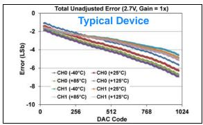
**FIGURE 1-315:** Total Unadjusted Error  $(V_{OUT})$  vs. DAC Code, and Temperature (Dual Channel - **MCP48FXB12**)  $(10\text{-bit}: V_{DD} = 2.7V, V_{REF} = 2.048V, VRxB:VRxA = '10' (V_{REF} Unbuffered), <math>Gx = '0' (1x)$ ).
