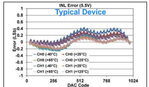
FIGURE 1-265: INL Error vs. DAC Code, and Temperature (Code 25 - 1000) (Dual Channel - MCP48FXB12)
