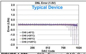
**FIGURE 1-270:** DNL Error vs. DAC Code, and Temperature (Code 25 - 1000) (Single Channel - **MCP48FXB11**) (10-bit:  $V_{DD} = 1.8V$ ,  $V_{REF} = V_{DD}$ ,  $VRxB:VRxA = '10' (V_{REF} Unbuffered)$ , Gx = '0' (1x)),
