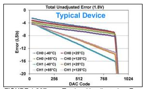
**FIGURE 1-297:** Total Unadjusted Error  $(V_{OUT})$  vs. DAC Code, and Temperature (Dual Channel - **MCP48FXB12**) (10-bit:  $V_{DD} = 1.8V$ ,  $V_{REF} = 1V$ , VRxB:VRxA = '10' ( $V_{REF}$  Unbuffered), Gx = '1' (2x)), (see **Appendix B.3** for additional information).
