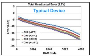
**FIGURE 1-41:** Total Unadjusted Error  $(V_{OUT})$  vs. DAC Code, and Temperature (Single Channel - **MCP48FXB21**) (12-bit:  $V_{DD} = 2.7V$ ,  $VRxB:VRxA = '00' (V_{DD})$ , Gx = '0' (1x)).
