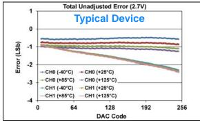
**FIGURE 1-548:** Total Unadjusted Error  $(V_{OUT})$  vs. DAC Code, and Temperature (Dual Channel - **MCP48FXB02**) (8-bit:  $V_{DD} = 2.7V$ ,  $V_{REF} = 1V$ , VRxB:VRxA = '11' ( $V_{REF}$  Buffered), Gx = '1' (2x).
