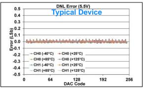
FIGURE 1-487: DNL Error vs. DAC Code, and Temperature (Code 6 - 250) (Dual Channel - MCP48FXB02) (8-bit:  $V_{DD} = 5.5V$ ,  $V_{REF} = 1V$ , VRxB:VRxA = '10' ( $V_{RFF}$  Unbuffered), Gx = '1'(2x)).
