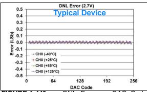
**FIGURE 1-449:** DNL Error vs. DAC Code, and Temperature (Code 6 - 250) (Single Channel - **MCP48FXB01**) (8-bit:  $V_{DD} = 2.7V$ ,  $V_{REF} = V_{DD}$ ,
