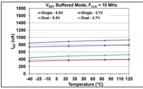
**FIGURE 1-21:** Average Device Supply Current - Active Interface ( $I_{DDA}$ ) ( $F_{SCK} = 10 \text{ MHz}$ ) vs. Voltage and Temperature,  $VRxB:VRxA = '11' (V_{RFF} \text{ Buffered mode})$ .
