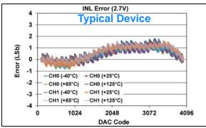
FIGURE 1-122: INL Error vs. DAC Code, and Temperature (Code 100 - 4000) (Dual Channel - MCP48FXB22) (12-bit:  $V_{DD} = 2.7V$ ,  $V_{REF} = 1V$ , VRxB:VRxA = '10' ( $V_{RFF}$  Unbuffered), Gx = '1' (2x).
