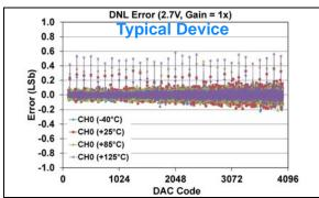
FIGURE 1-72: DNL Error vs. DAC Code, and Temperature (Code 100 - 4000) (Single Channel - MCP48FXB21) (12-bit:  $V_{DD} = 2.7V$ , VRxB:VRxA = '01' (Bandgap), Gx = '0' (1x)).
