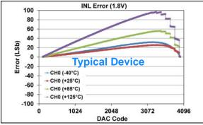
**FIGURE 1-156:** INL Error vs. DAC Code, and Temperature (Code 100 - 4000) (Single Channel - **MCP48FXB21**) (12-bit:  $V_{DD} = 1.8V$ ,  $V_{REF} = V_{DD}$ ,  $VRxB:VRxA = '11' (V_{REF} Buffered)$ , Gx = '0' (1x)), (see **Appendix B.4** for additional information).
