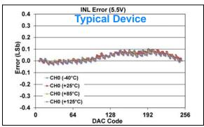
FIGURE 1-532: INL Error vs. DAC Code, and Temperature (Code 6 - 250) (Single Channel - MCP48FXB01) (8-bit:  $V_{DD} = 5.5V$ ,  $V_{REF} = 1V$ , VRxB:VRxA = '11' ( $V_{REF}$  Buffered), Gx = '0' (1x)).
