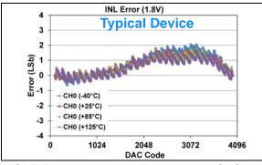
**FIGURE 1-174:** INL Error vs. DAC Code, and Temperature (Code 100 - 4000) (Single Channel - **MCP48FXB21**) (12-bit:  $V_{DD} = 1.8V$ ,  $V_{REF} = 1V$ ,  $V_{RXB}:V_{RXA} = '11'$  ( $V_{REF}$  Buffered),  $G_{X} = '0'$  (1x)).
