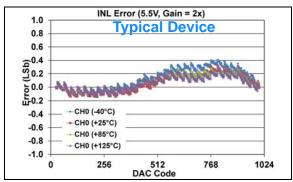
FIGURE 1-244: INL Error vs. DAC Code, and Temperature (Code 25 - 1000) (Single Channel - MCP48FXB11) (10-bit:  $V_{DD} = 5.5V$ , VRxB:VRxA = '01' (Bandgap), Gx = '1' (2x)).
