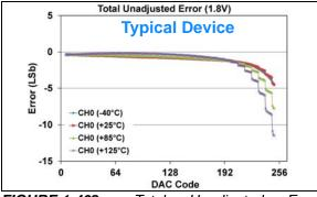
**FIGURE 1-402:** Total Unadjusted Error  $(V_{OUT})$  vs. DAC Code, and Temperature (Single Channel - **MCP48FXB01**)  $(8\text{-bit}: V_{DD} = 1.8V, VRxB:VRxA = '00' (V_{DD}), Gx = '0' (1x)),$  (see **Appendix B.1** for additional information).
