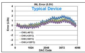
**FIGURE 1-190:** INL Error vs. DAC Code, and Temperature (Code 100 - 4000) (Single Channel - **MCP48FXB21**) (12-bit:  $V_{DD} = 5.5V$ ,  $V_{REF} = 1V$ ,  $V_{RXB}$ : $V_{RXA} = '11'$  ( $V_{RFF}$  Buffered),  $G_{X} = '1'$  ( $Z_{X}$ ).
