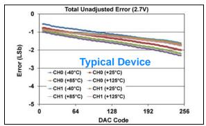
**FIGURE 1-458:** Total Unadjusted Error  $(V_{OUT})$  vs. DAC Code, and Temperature (Dual Channel - **MCP48FXB02**) (8-bit:  $V_{DD} = 2.7V$ ,  $V_{REF} = 1V$ , VRxB:VRxA = '10' ( $V_{RFF}$  Unbuffered), Gx = '0' (1x)).
