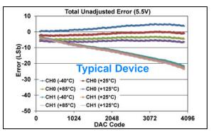
**FIGURE 1-187:** Total Unadjusted Error  $(V_{OUT})$  vs. DAC Code, and Temperature (Dual Channel - **MCP48FXB22**) (12-bit:  $V_{DD} = 5.5V$ ,  $V_{REF} = 1V$ , VRxB:VRxA = '11' ( $V_{REF}$  Buffered), Gx = '1' (2x).
