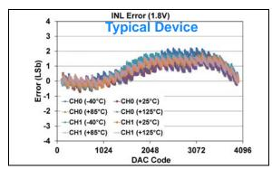
FIGURE 1-105: INL Error vs. DAC Code, and Temperature (Code 100 - 4000) (Dual Channel - MCP48FXB22) (12-bit:  $V_{DD} = 1.8V$ ,  $V_{REF} = 1V$ ,  $V_{RXB}$ :  $V_{RXA} = '10'$  ( $V_{REF}$  Unbuffered),  $G_{X} = '0'$  (1x)).
