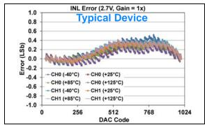
FIGURE 1-249: INL Error vs. DAC Code, and Temperature (Code 25 - 1000) (Dual Channel - MCP48FXB12) (10-bit:  $V_{DD} = 2.7V$ , VRxB:VRxA = '01' (Bandgap), Gx = '0' (1x)).
