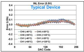
**FIGURE 1-481:** INL Error vs. DAC Code, and Temperature (Code 6 - 250) (Dual Channel - **MCP48FXB02**) (8-bit:  $V_{DD} = 5.5V$ ,  $V_{REF} = 1V$ ,  $V_{RXB}:V_{RXA} = '10'$  ( $V_{RFF}$  Unbuffered),  $G_{X} = '1'$  (2x)).
