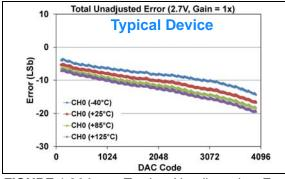
**FIGURE 1-204:** Total Unadjusted Error  $(V_{OUT})$  vs. DAC Code, and Temperature (Single Channel - **MCP48FXB21**) (**12-bit**:  $V_{DD} = 2.7V$ ,  $V_{REF} = 2.048V$ , VRxB:VRxA = '11'  $(V_{REF}$  Buffered), Gx = '0' (1x)).
