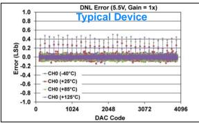
FIGURE 1-143: DNL Error vs. DAC Code, and Temperature (Code 100 - 4000) (Single Channel - MCP48FXB21) (12-bit:  $V_{DD} = 5.5V$ ,  $V_{REF} = 2.048V$ ,  $VRxB:VRxA = '10' (V_{REF} Unbuffered)$ , Gx = '0' (1x)).
