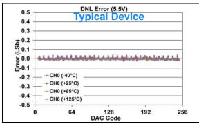
**FIGURE 1-466:** DNL Error vs. DAC Code, and Temperature (Code 6 - 250) (Single Channel - **MCP48FXB01**) (8-bit:  $V_{DD} = 5.5V$ ,  $V_{REF} = 1V$ ,  $V_{RXB}:V_{RXA} = '10'$  ( $V_{RFF}$  Unbuffered),  $G_{X} = '0'$  (1x)).
