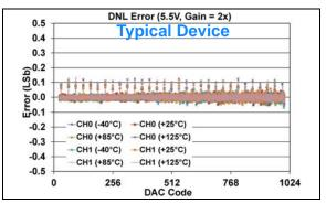
**FIGURE 1-253:** DNL Error vs. DAC Code, and Temperature (Code 25 - 1000) (Dual Channel - **MCP48FXB12**) (10-bit:  $V_{DD} = 5.5V$ , VRxB:VRxA = '01' (Bandgap), Gx = '1' (2x)).
