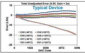
**FIGURE 1-205:** Total Unadjusted Error  $(V_{OUT})$  vs. DAC Code, and Temperature (Dual Channel - **MCP48FXB22**) (12-bit:  $V_{DD} = 5.5V$ ,  $V_{REF} = 2.048V$ ,  $VRxB:VRxA = '11' (V_{RFF} Buffered)$ , Gx = '1' (2x)).
