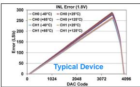
**FIGURE 1-195:** INL Error vs. DAC Code, and Temperature (Code 100 - 4000) (Dual Channel - **MCP48FXB22**) (**12-bit**:  $V_{DD} = 1.8V$ ,  $V_{REF} = 1V$ , VRxB:VRxA = '11' ( $V_{REF}$  Buffered), Gx = '1' (Zx), (see **Appendix B.5** for additional information).
