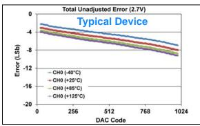
**FIGURE 1-275:** Total Unadjusted Error  $(V_{OUT})$  vs. DAC Code, and Temperature (Single Channel - **MCP48FXB11**)  $(10\text{-bit}: V_{DD} = 2.7V, V_{REF} = 1V, VRxB:VRxA = '10' (V_{RFF} Unbuffered), <math>Gx = '0' (1x)$ ).
