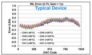
FIGURE 1-321: INL Error vs. DAC Code, and Temperature (Code 25 - 1000) (Dual Channel - MCP48FXB12) (10-bit:  $V_{DD} = 2.7V$ ,  $V_{REF} = 2.048V$ ,  $VRxB:VRxA = '10' (V_{REF} Unbuffered)$ , Gx = '0' (1x)).
