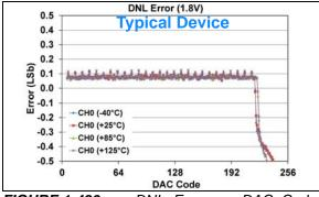
**FIGURE 1-486:** DNL Error vs. DAC Code, and Temperature (Code 6 - 250) (Single Channel - **MCP48FXB01**) (8-bit:  $V_{DD} = 1.8V$ ,  $V_{REF} = 1V$ ,  $V_{RXB}:V_{RXA} = '10'$  ( $V_{REF}$  Unbuffered),  $G_{X} = '1'(2x)$ ), (see **Appendix B.3** for additional information).
