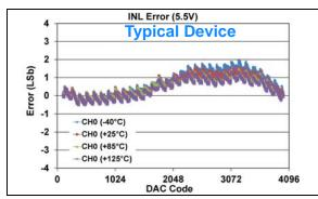
FIGURE 1-100: INL Error vs. DAC Code, and Temperature (Code 100 - 4000) (Single Channel - MCP48FXB21) (12-bit:  $V_{DD} = 5.5V$ ,  $V_{REF} = 1V$ , VRxB:VRxA = '10' ( $V_{RFF}$  Unbuffered), Gx = '0' (1x)).
