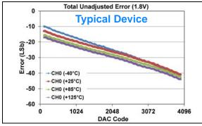
**FIGURE 1-96:** Total Unadjusted Error  $(V_{OUT})$  vs. DAC Code, and Temperature (Single Channel - **MCP48FXB21**) (12-bit:  $V_{DD} = 1.8V$ ,  $V_{REF} = 1V$ ,  $V_{RXB}$ :  $V_{RXA} = '10'$  ( $V_{REF}$  Unbuffered),  $V_{REF} = '10'$  ( $V_{REF} = 1V$ ).
