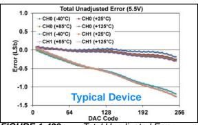
**FIGURE 1-439:** Total Unadjusted Error  $(V_{OUT})$  vs. DAC Code, and Temperature (Dual Channel - **MCP48FXB02**)  $(8\text{-bit}: V_{DD} = 5.5V, V_{REF} = V_{DD}, VRxB:VRxA = '10' (V_{REF} Unbuffered), Gx = '0' (1x)).$
