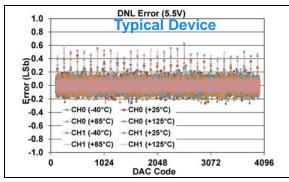
FIGURE 1-106: DNL Error vs. DAC Code, and Temperature (Code 100 - 4000) (Single Channel - MCP48FXB21) (12-bit:  $V_{DD} = 5.5V$ ,  $V_{REF} = 1V$ , VRxB:VRxA = '10' ( $V_{REF}$  Unbuffered), Gx = '0' (1x)).
