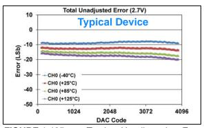
**FIGURE 1-185:** Total Unadjusted Error  $(V_{OUT})$  vs. DAC Code, and Temperature (Single Channel - **MCP48FXB21**) (12-bit:  $V_{DD} = 2.7V$ ,  $V_{REF} = 1V$ , VRxB:VRxA = '11' ( $V_{REF}$  Buffered), Gx = '1' (2x)).
