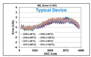
FIGURE 1-177: INL Error vs. DAC Code, and Temperature (Code 100 - 4000) (Dual Channel - MCP48FXB22) (12-bit:  $V_{DD} = 1.8V$ ,  $V_{REF} = 1V$ , VRxB:VRxA = '11' ( $V_{REF}$  Buffered), Gx = '0' (1x)).
