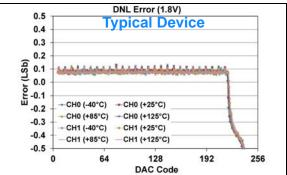
**FIGURE 1-561:** DNL Error vs. DAC Code, and Temperature (Code 6 - 250) (Dual Channel - **MCP48FXB02**) (8-bit:  $V_{DD} = 1.8V$ ,  $V_{REF} = 1V$ , VRxB:VRxA = '11' ( $V_{REF}$  Buffered), Gx = '1' (2x)), (see **Appendix B.5** for additional information).
