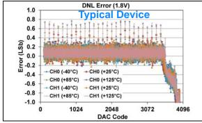
**FIGURE 1-129:** DNL Error vs. DAC Code, and Temperature (Code 100 - 4000) (Dual Channel - **MCP48FXB22**) (12-bit:  $V_{DD} = 1.8V$ ,  $V_{REF} = 1V$ , VRxB:VRxA = '10' ( $V_{REF}$  Unbuffered), Gx = '1' (2x)), (see **Appendix B.3** for additional information).
