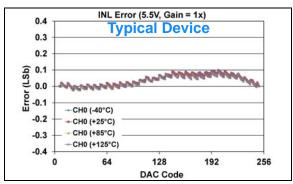
**FIGURE 1-497:** INL Error vs. DAC Code, and Temperature (Code 6 - 250) (Single Channel - **MCP48FXB01**) (8-bit:  $V_{DD} = 5.5V$ ,  $V_{REF} = 2.048V$ ,  $VRxB:VRxA = '10' (V_{REF} Unbuffered)$ , Gx = '0' (1x)).
