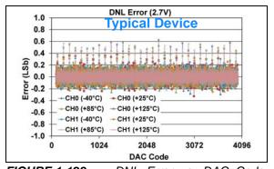
FIGURE 1-128: DNL Error vs. DAC Code, and Temperature (Code 100 - 4000) (Dual Channel - MCP48FXB22) (12-bit:  $V_{DD} = 2.7V$ ,  $V_{REF} = 1V$ , VRxB:VRxA = '10' ( $V_{REF}$  Unbuffered), Gx = '1' (2x).
