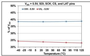
**FIGURE 1-25:** Average  $V_{IH}$  and  $V_{IL}$  (SDI, SCK,  $\overline{CS}$ , and  $\overline{LAT}$  pins) ( $V_{DD} = 5.5V$ ) vs. Temperature.
