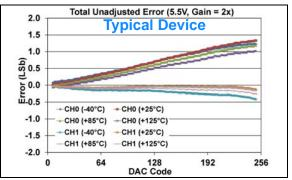
**FIGURE 1-421:** Total Unadjusted Error  $(V_{OUT})$  vs. DAC Code, and Temperature (Dual Channel - **MCP48FXB02**) (8-bit:  $V_{DD} = 5.5V$ , VRxB:VRxA = '01' (Bandgap), Gx = '1' (2x)).
