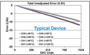
**FIGURE 1-331:** Total Unadjusted Error  $(V_{OUT})$  vs. DAC Code, and Temperature (Dual Channel - **MCP48FXB12**)  $(10\text{-bit}: V_{DD} = 5.5V, V_{REF} = V_{DD}, VRxB:VRxA = '11' (V_{REF} Buffered), Gx = '0' (1x)).$
