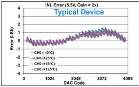
FIGURE 1-136: INL Error vs. DAC Code, and Temperature (Code 100 - 4000) (Single Channel - MCP48FXB21) (12-bit:  $V_{DD} = 5.5V$ ,  $V_{REF} = 2.048V$ ,  $VRxB:VRxA = '10' (V_{REF} Unbuffered)$ , Gx = '1' (2x)).
