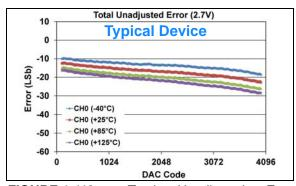
**FIGURE 1-113:** Total Unadjusted Error  $(V_{OUT})$  vs. DAC Code, and Temperature (Single Channel - **MCP48FXB21**) (12-bit:  $V_{DD} = 2.7V$ ,  $V_{REF} = 1V$ , VRxB:VRxA = '10' ( $V_{REF}$  Unbuffered), Gx = '1' (2x)).
