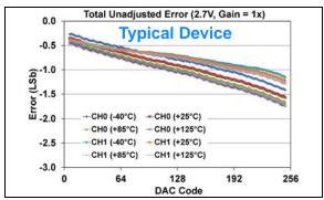
**FIGURE 1-495:** Total Unadjusted Error  $(V_{OUT})$  vs. DAC Code, and Temperature (Dual Channel - **MCP48FXB02**) (8-bit:  $V_{DD} = 2.7V$ ,  $V_{REF} = 2.048V$ ,  $VRxB:VRxA = '10' (V_{REF} Unbuffered)$ , Gx = '0' (1x)).
