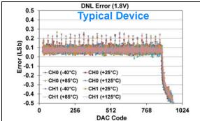
FIGURE 1-381: DNL Error vs. DAC Code, and Temperature (Code 25 - 1000) (Dual Channel - MCP48FXB12) (10-bit:  $V_{DD} = 1.8V$ ,  $V_{REF} = 1V$ , VRxB:VRxA = '11' ( $V_{REF}$  Buffered), Gx = '1' (Zx), (see Appendix B.5 for additional information).
