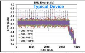
**FIGURE 1-126:** DNL Error vs. DAC Code, and Temperature (Code 100 - 4000) (Single Channel - **MCP48FXB21**) (12-bit:  $V_{DD} = 1.8V$ ,  $V_{REF} = 1V$ ,  $V_{RXB}$ : $V_{RXA} = '10'$  ( $V_{REF}$  Unbuffered),  $G_{X} = '1'$  (2x)), (see **Appendix B.3** for additional information).
