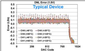
**FIGURE 1-309:** DNL Error vs. DAC Code, and Temperature (Code 25 - 1000) (Dual Channel - **MCP48FXB12**) (10-bit:  $V_{DD} = 1.8V$ ,  $V_{REF} = 1V$ , VRxB:VRxA = '10' ( $V_{REF}$  Unbuffered), Gx = '1' (Zx), (see **Appendix B.3** for additional information).
