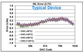
**FIGURE 1-281:** INL Error vs. DAC Code, and Temperature (Code 25 - 1000) (Single Channel - **MCP48FXB11**) (10-bit:  $V_{DD} = 2.7V$ ,  $V_{REF} = 1V$ , VRxB:VRxA = '10' ( $V_{RFF}$  Unbuffered), Gx = '0' (1x)).
