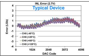
**FIGURE 1-119:** INL Error vs. DAC Code, and Temperature (Code 100 - 4000) (Single Channel - **MCP48FXB21**) (12-bit:  $V_{DD} = 2.7V$ ,  $V_{REF} = 1V$ , VRxB:VRxA = '10' ( $V_{REF}$  Unbuffered), Gx = '1' (2x)).
