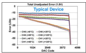
**FIGURE 1-189:** Total Unadjusted Error  $(V_{OUT})$  vs. DAC Code, and Temperature (Dual Channel - **MCP48FXB22**) (12-bit:  $V_{DD} = 1.8V$ ,  $V_{REF} = 1V$ , VRxB:VRxA = '11' ( $V_{REF}$  Buffered), Gx = '1' (2x), (see **Appendix B.5** for additional information).
