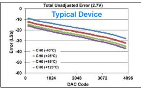
**FIGURE 1-95:** Total Unadjusted Error  $(V_{OUT})$  vs. DAC Code, and Temperature (Single Channel - **MCP48FXB21**) (12-bit:  $V_{DD} = 2.7V$ ,  $V_{REF} = 1V$ ,  $V_{RXB}$ :  $V_{RXA} = '10'$  ( $V_{RFF}$  Unbuffered),  $V_{RFF} = '10'$  ( $V_{RFF} = 10'$ ).
