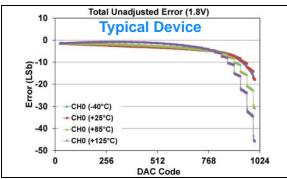
**FIGURE 1-222:** Total Unadjusted Error  $(V_{OUT})$  vs. DAC Code, and Temperature (Single Channel - **MCP48FXB11**)  $(10\text{-bit}: V_{DD} = 1.8V, VRxB:VRxA = '00' (V_{DD}), Gx = '0' (1x)),$  (see **Appendix B.1** for additional information).
