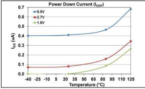
**FIGURE 1-5:** Average Power-Down Current (I<sub>DDP</sub>) vs. Temperature and Voltage.
