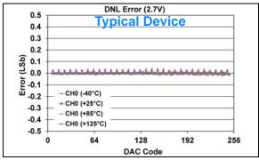
**FIGURE 1-413:** DNL Error vs. DAC Code, and Temperature (Code 6 - 250) (Single Channel - **MCP48FXB01**) (8-bit:  $V_{DD} = 2.7V$ ,  $V_{RXB}:V_{RXA} = '00' (V_{DD})$ ,  $G_{X} = '0' (1x)$ ).
