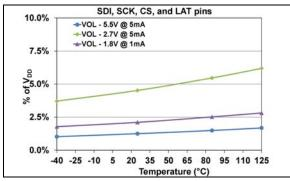
**FIGURE 1-31:** Average  $V_{OL}$  (SDO pin) vs. Voltage and Temperature.
