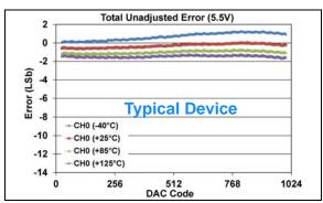
**FIGURE 1-364:** Total Unadjusted Error  $(V_{OUT})$  vs. DAC Code, and Temperature (Single Channel - **MCP48FXB11**)  $(10\text{-bit}: V_{DD} = 5.5\text{V}, V_{REF} = 1\text{V}, VRxB:VRxA = '11' (V_{REF} Buffered), Gx = '1' (2x)).$
