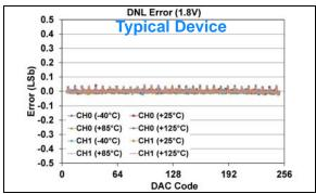
**FIGURE 1-543:** DNL Error vs. DAC Code, and Temperature (Code 6 - 250) (Dual Channel - **MCP48FXB02**) (8-bit:  $V_{DD} = 1.8V$ ,  $V_{REF} = 1V$ ,  $V_{RXB}$ :  $V_{RXA} = '11'$  ( $V_{REF}$  Buffered),  $G_{X} = '0'$  (1x)).
