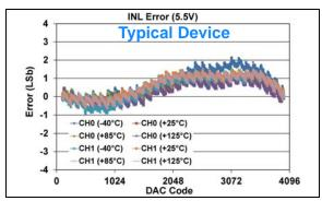
**FIGURE 1-193:** INL Error vs. DAC Code, and Temperature (Code 100 - 4000) (Dual Channel - **MCP48FXB22**) (12-bit:  $V_{DD} = 5.5V$ ,  $V_{REF} = 1V$ , VRxB:VRxA = '11' ( $V_{REF}$  Buffered), Gx = '1' (2x).
