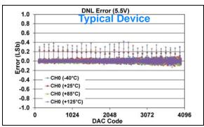
FIGURE 1-160: DNL Error vs. DAC Code, and Temperature (Code 100 - 4000) (Single Channel - MCP48FXB21) (12-bit:  $V_{DD} = 5.5V$ ,  $V_{REF} = V_{DD}$ ,  $VRxB:VRxA = '11' (V_{REF} Buffered)$ , Gx = '0' (1x)).
