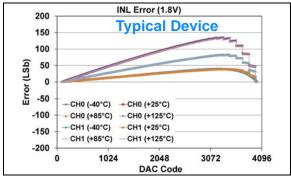
**FIGURE 1-51:** INL Error vs. DAC Code, and Temperature (Code 100 - 4000) (Dual Channel - **MCP48FXB22**) (12-bit:  $V_{DD} = 1.8V$ ,  $VRxB:VRxA = '00' (V_{DD})$ , Gx = '0' (1x)), (see **Appendix B.1** for additional information).
