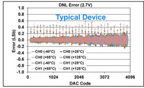
FIGURE 1-56: DNL Error vs. DAC Code, and Temperature (Code 100 - 4000) (Dual Channel - MCP48FXB22) (12-bit:  $V_{DD} = 2.7V$ ,  $VRxB:VRxA = '00' (V_{DD})$ , Gx = '0' (1x)).
