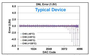
**FIGURE 1-90:** DNL Error vs. DAC Code, and Temperature (Code 100 - 4000) (Single Channel - **MCP48FXB21**) (12-bit:  $V_{DD} = 1.8V$ ,  $V_{REF} = V_{DD}$ , VRXB:VRXA = '10' ( $V_{REF}$  Unbuffered), GX = '0' (1x)), (see **Appendix B.2** for additional information).
