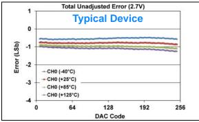
**FIGURE 1-545:** Total Unadjusted Error  $(V_{OUT})$  vs. DAC Code, and Temperature (Single Channel - **MCP48FXB01**) (8-bit:  $V_{DD} = 2.7V$ ,  $V_{REF} = 1V$ ,  $V_{RXB}:V_{RXA} = '11'$  ( $V_{REF}$  Buffered),  $G_{X} = '1'$  ( $Z_{X}$ ).
