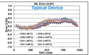
**FIGURE 1-229:** INL Error vs. DAC Code, and Temperature (Code 25 - 1000) (Dual Channel - **MCP48FXB12**) (10-bit:  $V_{DD} = 5.5V$ ,  $VRxB:VRxA = '00' (V_{DD})$ , Gx = '0' (1x)).
