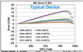
**FIGURE 1-267:** INL Error vs. DAC Code, and Temperature (Code 25 - 1000) (Dual Channel - **MCP48FXB12**) (10-bit:  $V_{DD} = 1.8V$ ,  $V_{REF} = V_{DD}$ ,  $VRxB:VRxA = '10' (V_{REF} Unbuffered)$ , Gx = '0' (1x),
