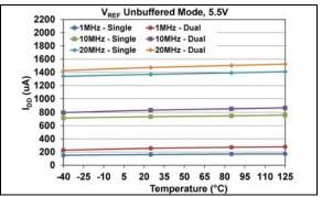
**FIGURE 1-19:** Average Device Supply Current vs. F<sub>SCK</sub> Frequency, Voltage and Temperature,
