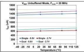
**FIGURE 1-16:** Average Device Supply Current - Active Interface ( $I_{DDA}$ ) ( $F_{SCK} = 20$  MHz) vs. Voltage and Temperature,
