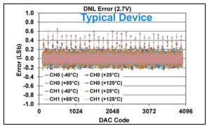
**FIGURE 1-110:** DNL Error vs. DAC Code, and Temperature (Code 100 - 4000) (Dual Channel - **MCP48FXB22**) (12-bit:  $V_{DD} = 2.7V$ ,  $V_{REF} = 1V$ , VRxB:VRxA = '10' ( $V_{RFF}$  Unbuffered), Gx = '0' (1x)).
