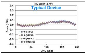
FIGURE 1-551: INL Error vs. DAC Code, and Temperature (Code 6 - 250) (Single Channel - MCP48FXB01) (8-bit:  $V_{DD} = 2.7V$ ,  $V_{REF} = 1V$ , VRxB:VRxA = '11' ( $V_{RFF}$  Buffered), Gx = '1' (2x).
