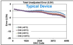
**FIGURE 1-76:** Total Unadjusted Error  $(V_{OUT})$  vs. DAC Code, and Temperature (Single Channel - **MCP48FXB21**)  $(12\text{-bit}: V_{DD} = 5.5V, V_{REF} = V_{DD}, VRxB:VRxA = '10' (V_{REF} Unbuffered), Gx = '0' (1x)).$
