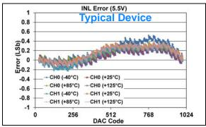
**FIGURE 1-373:** INL Error vs. DAC Code, and Temperature (Code 25 - 1000) (Dual Channel - **MCP48FXB12**) (10-bit:  $V_{DD} = 5.5V$ ,  $V_{REF} = 1V$ ,  $V_{RXB}$ : $V_{RXA} = '11'$  ( $V_{REF}$  Buffered),  $G_{X} = '1'$  ( $Z_{X}$ ).
