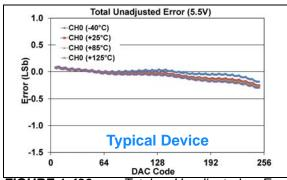
**FIGURE 1-436:** Total Unadjusted Error  $(V_{OUT})$  vs. DAC Code, and Temperature (Single Channel - **MCP48FXB01**)  $(8\text{-bit}: V_{DD} = 5.5V, V_{REF} = V_{DD},$
