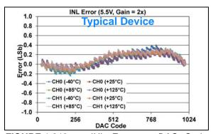
FIGURE 1-319: INL Error vs. DAC Code, and Temperature (Code 25 - 1000) (Dual Channel - MCP48FXB12) (10-bit:  $V_{DD} = 5.5V$ ,  $V_{REF} = 2.048V$ ,  $VRxB:VRxA = '10' (V_{REF} Unbuffered)$ , Gx = '1' (2x)).
