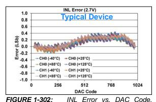
FIGURE 1-302: INL Error vs. DAC Code, and Temperature (Code 25 - 1000) (Dual Channel - MCP48FXB12) (10-bit:  $V_{DD} = 2.7V$ ,  $V_{REF} = 1V$ , VRxB:VRxA = '10' ( $V_{REF}$  Unbuffered), Gx = '1' (Zx).
