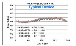
FIGURE 1-500: INL Error vs. DAC Code, and Temperature (Code 6 - 250) (Dual Channel - MCP48FXB02) (8-bit:  $V_{DD} = 5.5V$ ,  $V_{REF} = 2.048V$ ,  $VRxB:VRxA = '10' (V_{RFF} Unbuffered)$ , Gx = '0' (1x)).
