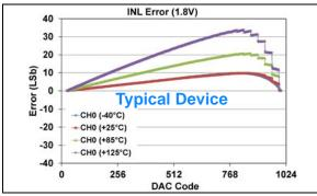
**FIGURE 1-228:** INL Error vs. DAC Code, and Temperature (Code 25 - 1000) (Single Channel - **MCP48FXB11**) (10-bit:  $V_{DD} = 1.8V$ ,  $VRxB:VRxA = '00' (V_{DD})$ , Gx = '0' (1x)), (see **Appendix B.1** for additional information).
