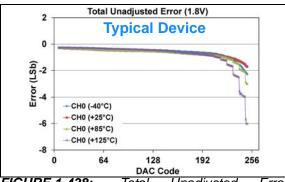
**FIGURE 1-438:** Total Unadjusted Error  $(V_{OUT})$  vs. DAC Code, and Temperature (Single Channel - **MCP48FXB01**)  $(8\text{-bit}: V_{DD} = 1.8V, V_{REF} = V_{DD}, VRxB:VRxA = '10' (V_{REF} Unbuffered), Gx = '0' (1x)), (see$ **Appendix B.2**for additional information).
