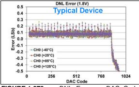
**FIGURE 1-378:** DNL Error vs. DAC Code, and Temperature (Code 25 - 1000) (Single Channel - **MCP48FXB11**) (10-bit:  $V_{DD} = 1.8V$ ,  $V_{REF} = 1V$ , VRxB:VRxA = '11' ( $V_{REF}$  Buffered), Gx = '1' (Zx), (see **Appendix B.5** for additional information).
