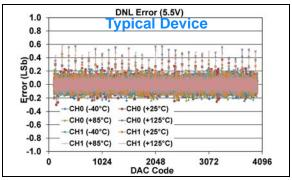
**FIGURE 1-199:** DNL Error vs. DAC Code, and Temperature (Code 100 - 4000) (Dual Channel - **MCP48FXB22**) (**12-bit**:  $V_{DD} = 5.5V$ ,  $V_{REF} = 1V$ , VRxB:VRxA = '11' ( $V_{RFF}$  Buffered), Gx = '1' (2x)).
