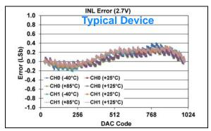
FIGURE 1-338: INL Error vs. DAC Code, and Temperature (Code 25 - 1000) (Dual Channel - MCP48FXB12) (10-bit:  $V_{DD} = 2.7V$ ,  $V_{REF} = V_{DD}$ ,  $VRxB:VRxA = '11' (V_{RFF} Buffered)$ , Gx = '0' (1x)).
