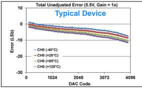
**FIGURE 1-203:** Total Unadjusted Error  $(V_{OUT})$  vs. DAC Code, and Temperature (Single Channel - **MCP48FXB21**) (12-bit:  $V_{DD} = 5.5V$ ,  $V_{REF} = 2.048V$ ,  $VRxB:VRxA = '11' (V_{REF} Buffered)$ , Gx = '0' (1x)).
