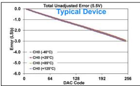
**FIGURE 1-508:** Total Unadjusted Error  $(V_{OUT})$  vs. DAC Code, and Temperature (Single Channel - **MCP48FXB01**) (8-bit:  $V_{DD} = 5.5V$ ,  $V_{REF} = V_{DD}$ ,  $VRxB:VRxA = '11' (V_{REF} Buffered)$ , Gx = '0' (1x)).
