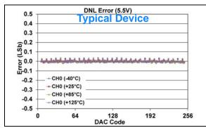
FIGURE 1-538: DNL Error vs. DAC Code, and Temperature (Code 6 - 250) (Single Channel - MCP48FXB01) (8-bit:  $V_{DD} = 5.5V$ ,  $V_{REF} = 1V$ ,  $V_{RXB}:V_{RXA} = '11'$  ( $V_{REF}$  Buffered),  $G_{X} = '0'$  (1x)).
