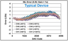
FIGURE 1-68: INL Error vs. DAC Code, and Temperature (Code 100 - 4000) (Dual Channel - MCP48FXB22) (12-bit:  $V_{DD} = 5.5V$ , VRxB:VRxA = '01' (Bandgap), Gx = '0' (1x)).
