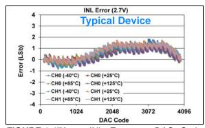
FIGURE 1-176: INL Error vs. DAC Code, and Temperature (Code 100 - 4000) (Dual Channel - MCP48FXB22) (12-bit:  $V_{DD} = 2.7V$ ,  $V_{REF} = 1V$ , VRxB:VRxA = '11' ( $V_{REF}$  Buffered), Gx = '0' (1x)).
