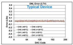
FIGURE 1-542: DNL Error vs. DAC Code, and Temperature (Code 6 - 250) (Dual Channel - MCP48FXB02) (8-bit:  $V_{DD} = 2.7V$ ,  $V_{REF} = 1V$ , VRxB:VRxA = '11' ( $V_{RFF}$  Buffered), Gx = '0' (1x)).
