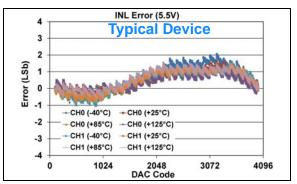
**FIGURE 1-121:** INL Error vs. DAC Code, and Temperature (Code 100 - 4000) (Dual Channel - **MCP48FXB22**) (12-bit:  $V_{DD} = 5.5V$ ,  $V_{REF} = 1V$ , VRxB:VRxA = '10' ( $V_{REF}$  Unbuffered), Gx = '1' (2x)).
