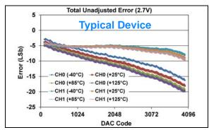
**FIGURE 1-44:** Total Unadjusted Error  $(V_{OUT})$  vs. DAC Code, and Temperature (Dual Channel - **MCP48FXB22**)  $(12\text{-bit}: V_{DD} = 2.7V, VRxB: VRxA = '00' (V_{DD}), Gx = '0' (1x)).$
