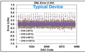
**FIGURE 1-108:** DNL Error vs. DAC Code, and Temperature (Code 100 - 4000) (Single Channel - **MCP48FXB21**) (12-bit:  $V_{DD} = 1.8V$ ,  $V_{REF} = 1V$ ,  $V_{RXB}$ :  $V_{RXA} = '10'$  ( $V_{REF}$  Unbuffered),  $G_{X} = '0'$  (1x)).
