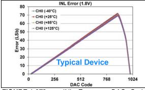
**FIGURE 1-372:** INL Error vs. DAC Code, and Temperature (Code 25 - 1000) (Single Channel - **MCP48FXB11**) (10-bit:  $V_{DD} = 1.8V$ ,  $V_{REF} = 1V$ ,  $V_{RXB}:V_{RXA} = '11'$  ( $V_{REF}$  Buffered),  $G_{X} = '1'$  ( $Z_{X}$ ), (see **Appendix B.5** for additional information).
