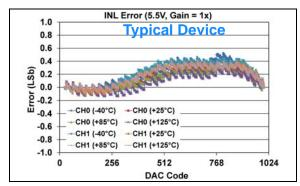
FIGURE 1-248: INL Error vs. DAC Code, and Temperature (Code 25 - 1000) (Dual Channel - MCP48FXB12) (10-bit:  $V_{DD} = 5.5V$ , VRxB:VRxA = '01' (Bandgap), Gx = '0' (1x)).
