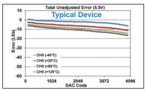
**FIGURE 1-112:** Total Unadjusted Error  $(V_{OUT})$  vs. DAC Code, and Temperature (Single Channel - **MCP48FXB21**) (12-bit:  $V_{DD} = 5.5V$ ,  $V_{REF} = 1V$ , VRxB:VRxA = '10' ( $V_{REF}$  Unbuffered), Gx = '1' (2x)).
