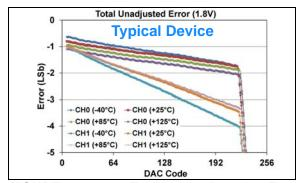
**FIGURE 1-477:** Total Unadjusted Error  $(V_{OUT})$  vs. DAC Code, and Temperature (Dual Channel - **MCP48FXB02**) (8-bit:  $V_{DD} = 1.8V$ ,  $V_{REF} = 1V$ , VRxB:VRxA = '10' ( $V_{REF}$  Unbuffered), Gx = '1' (2x)), (see **Appendix B.3** for additional information).
