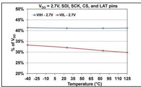
**FIGURE 1-26:** Average  $V_{IH}$  and  $V_{IL}$  (SDI, SCK,  $\overline{CS}$ , and  $\overline{LAT}$  pins) ( $V_{DD}=2.7V$ ) vs. Temperature.
