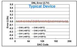
FIGURE 1-488: DNL Error vs. DAC Code, and Temperature (Code 6 - 250) (Dual Channel - MCP48FXB02) (8-bit:  $V_{DD} = 2.7V$ ,  $V_{REF} = 1V$ , VRxB:VRxA = '10' ( $V_{REF}$  Unbuffered), Gx = '1' (2x)).
