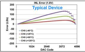
**FIGURE 1-48:** INL Error vs. DAC Code, and Temperature (Code 100 - 4000) (Single Channel - **MCP48FXB21**) (12-bit:  $V_{DD} = 1.8V$ ,  $VRxB:VRxA = '00' (V_{DD})$ , Gx = '0' (1x)), (see **Appendix B.1** for additional information).
