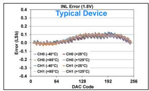
**FIGURE 1-537:** INL Error vs. DAC Code, and Temperature (Code 6 - 250) (Dual Channel - **MCP48FXB02**) (8-bit:  $V_{DD} = 1.8V$ ,  $V_{REF} = 1V$ ,  $V_{RXB}:V_{RXA} = '11'$  ( $V_{REF}$  Buffered),  $G_{X} = '0'$  (1x)).
