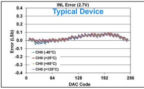
**FIGURE 1-461:** INL Error vs. DAC Code, and Temperature (Code 6 - 250) (Single Channel - **MCP48FXB01**) (8-bit:  $V_{DD} = 2.7V$ ,  $V_{REF} = 1V$ ,  $V_{RXB}:V_{RXA} = '10'$  ( $V_{REF}$  Unbuffered),  $G_{X} = '0'$  (1x)).
