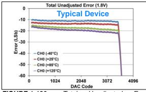
**FIGURE 1-186:** Total Unadjusted Error  $(V_{OUT})$  vs. DAC Code, and Temperature (Single Channel - **MCP48FXB21**) (12-bit:  $V_{DD} = 1.8V$ ,  $V_{REF} = 1V$ , VRxB:VRxA = '11' ( $V_{REF}$  Buffered), Gx = '1' (2x)), (see **Appendix B.5** for additional information).
