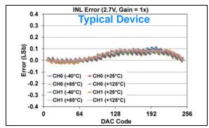
FIGURE 1-573: INL Error vs. DAC Code, and Temperature (Code 6 - 250) (Dual Channel - MCP48FXB02) (8-bit:  $V_{DD} = 2.7V$ ,  $V_{REF} = 2.048V$ ,  $VRxB:VRxA = '11' (V_{REF} Buffered)$ , Gx = '0' (1x)).
