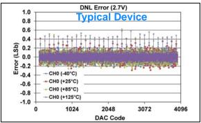
**FIGURE 1-197:** DNL Error vs. DAC Code, and Temperature (Code 100 - 4000) (Single Channel - **MCP48FXB21**) (**12-bit**:  $V_{DD} = 2.7V$ ,  $V_{REF} = 1V$ , VRxB:VRxA = '11' ( $V_{RFF}$  Buffered), Gx = '1' (2x).
