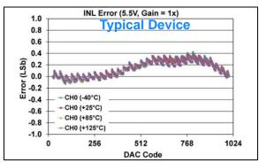
**FIGURE 1-317:** INL Error vs. DAC Code, and Temperature (Code 25 - 1000) (Single Channel - **MCP48FXB11**) (10-bit:  $V_{DD} = 5.5V$ ,  $V_{REF} = 2.048V$ ,  $VRxB:VRxA = '10' (V_{REF} Unbuffered)$ , Gx = '0' (1x)).
