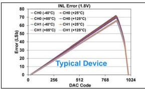
**FIGURE 1-375:** INL Error vs. DAC Code, and Temperature (Code 25 - 1000) (Dual Channel - **MCP48FXB12**) (10-bit:  $V_{DD} = 1.8V$ ,  $V_{REF} = 1V$ , VRxB:VRxA = '11' ( $V_{REF}$  Buffered), Gx = '1' (2x)), (see **Appendix B.5** for additional information).
