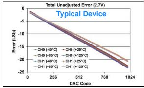
**FIGURE 1-332:** Total Unadjusted Error  $(V_{OUT})$  vs. DAC Code, and Temperature (Dual Channel - **MCP48FXB12**)  $(10\text{-bit}: V_{DD} = 2.7V, V_{REF} = V_{DD}, VRxB:VRxA = '11' (V_{REF} Buffered), Gx = '0' (1x)).$
