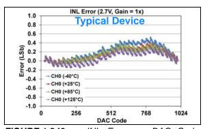
FIGURE 1-246: INL Error vs. DAC Code, and Temperature (Code 25 - 1000) (Single Channel - MCP48FXB11) (10-bit:  $V_{DD} = 2.7V$ , VRxB:VRxA = '01' (Bandgap), Gx = '0' (1x)).
