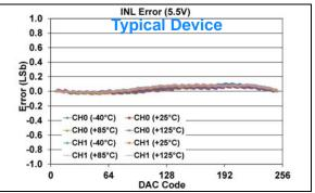
**FIGURE 1-409:** INL Error vs. DAC Code, and Temperature (Code 6 - 250) (Dual Channel - **MCP48FXB02**) (8-bit:  $V_{DD} = 5.5V$ ,  $V_{RXB}:V_{RXA} = '00' (V_{DD})$ ,  $G_{X} = '0' (1x)$ ).
