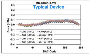
FIGURE 1-536: INL Error vs. DAC Code, and Temperature (Code 6 - 250) (Dual Channel - MCP48FXB02) (8-bit:  $V_{DD} = 2.7V$ ,  $V_{REF} = 1V$ , VRxB:VRxA = '11' ( $V_{REF}$  Buffered), Gx = '0' (1x)).
