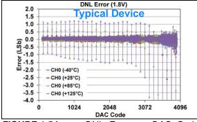
**FIGURE 1-54:** DNL Error vs. DAC Code, and Temperature (Code 100 - 4000) (Single Channel - **MCP48FXB21**) (12-bit:  $V_{DD} = 1.8V$ ,  $VRxB:VRxA = '00' (V_{DD})$ , Gx = '0' (1x)), (see **Appendix B.1** for additional information).
