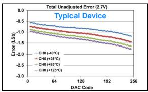
**FIGURE 1-527:** Total Unadjusted Error  $(V_{OUT})$  vs. DAC Code, and Temperature (Single Channel - **MCP48FXB01**) (8-bit:  $V_{DD} = 2.7V$ ,  $V_{REF} = 1V$ , VRxB:VRxA = '11'  $(V_{RFF} Buffered)$ , Gx = '0' (1x)).
