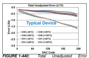
$(V_{OUT})$  vs. DAC Code, and Temperature (Dual Channel - **MCP48FXB02**) (8-bit:  $V_{DD} = 2.7V$ ,  $V_{REF} = V_{DD}$ ,  $VRxB:VRxA = '10' (V_{RFF} Unbuffered)$ , Gx = '0' (1x)).
