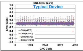
FIGURE 1-89: DNL Error vs. DAC Code, and Temperature (Code 100 - 4000) (Single Channel - MCP48FXB21) (12-bit:  $V_{DD} = 2.7V$ ,  $V_{REF} = V_{DD}$ ,  $VRxB:VRxA = '10' (V_{REF} Unbuffered)$ , Gx = '0' (1x)).
