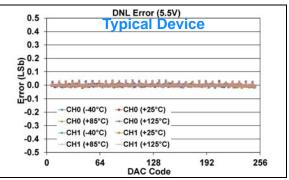
**FIGURE 1-541:** DNL Error vs. DAC Code, and Temperature (Code 6 - 250) (Dual Channel - **MCP48FXB02**) (8-bit:  $V_{DD} = 5.5V$ ,  $V_{REF} = 1V$ ,  $V_{RXB}:V_{RXA} = '11'$  ( $V_{RFF}$  Buffered),  $G_{X} = '0'$  (1x)).
