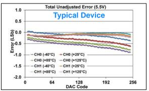
**FIGURE 1-529:** Total Unadjusted Error  $(V_{OUT})$  vs. DAC Code, and Temperature (Dual Channel - **MCP48FXB02**) (8-bit:  $V_{DD} = 5.5V$ ,  $V_{REF} = 1V$ , VRxB:VRxA = '11'  $(V_{RFF}$  Buffered), Gx = '0' (1x)).
