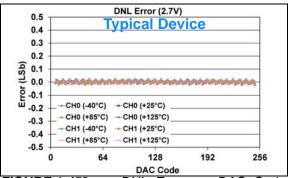
**FIGURE 1-452:** DNL Error vs. DAC Code, and Temperature (Code 6 - 250) (Dual Channel - **MCP48FXB02**) (8-bit:  $V_{DD} = 2.7V$ ,  $V_{REF} = V_{DD}$ ,
