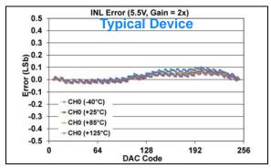
FIGURE 1-424: INL Error vs. DAC Code, and Temperature (Code 6 - 250) (Single Channel - MCP48FXB01) (8-bit:  $V_{DD} = 5.5V$ , VRxB:VRxA = '01' (Bandgap), Gx = '1' (2x)).
