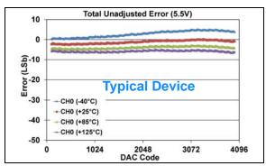
**FIGURE 1-184:** Total Unadjusted Error  $(V_{OUT})$  vs. DAC Code, and Temperature (Single Channel - **MCP48FXB21**)  $(12\text{-bit}: V_{DD} = 5.5V, V_{REF} = 1V, VRxB:VRxA = '11' (V_{REF} Buffered), Gx = '1' (2x)).$
