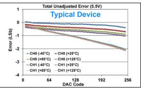
**FIGURE 1-475:** Total Unadjusted Error  $(V_{OUT})$  vs. DAC Code, and Temperature (Dual Channel - **MCP48FXB02**) (8-bit:  $V_{DD} = 5.5V$ ,  $V_{REF} = 1V$ ,  $V_{RXB}:V_{RXA} = '10'$  ( $V_{REF}$  Unbuffered),  $G_{X} = '1'$  ( $Z_{X}$ ).
