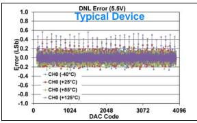
FIGURE 1-124: DNL Error vs. DAC Code, and Temperature (Code 100 - 4000) (Single Channel - MCP48FXB21) (12-bit:  $V_{DD} = 5.5V$ ,  $V_{REF} = 1V$ , VRxB:VRxA = '10' ( $V_{REF}$  Unbuffered), Gx = '1' (Zx).
