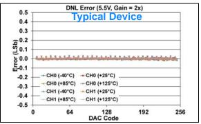
**FIGURE 1-433:** DNL Error vs. DAC Code, and Temperature (Code 6 - 250) (Dual Channel - **MCP48FXB02**) (8-bit:  $V_{DD} = 5.5V$ , VRxB:VRxA = '01' (Bandgap), Gx = '1' (2x)).
