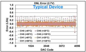
FIGURE 1-92: DNL Error vs. DAC Code, and Temperature (Code 100 - 4000) (Dual Channel - MCP48FXB22) (12-bit:  $V_{DD} = 2.7V$ ,  $V_{REF} = V_{DD}$ ,  $VRxB:VRxA = '10' (V_{RFF} Unbuffered)$ , Gx = '0' (1x)).
