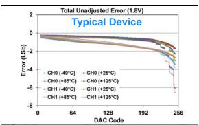
**FIGURE 1-441:** Total Unadjusted Error  $(V_{OUT})$  vs. DAC Code, and Temperature (Dual Channel - **MCP48FXB02**) (8-bit:  $V_{DD} = 1.8V$ ,  $V_{REF} = V_{DD}$ ,  $VRXB:VRXA = '10' (V_{REF} Unbuffered)$ , Gx = '0' (1x), (see **Appendix B.2** for additional information).
