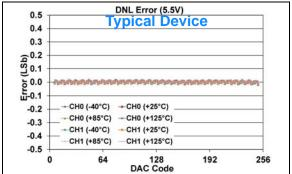
FIGURE 1-451: DNL Error vs. DAC Code, and Temperature (Code 6 - 250) (Dual Channel - MCP48FXB02)
