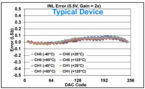
**FIGURE 1-427:** INL Error vs. DAC Code, and Temperature (Code 6 - 250) (Dual Channel - **MCP48FXB02**) (8-bit:  $V_{DD} = 5.5V$ , VRxB:VRxA = '01' (Bandgap), Gx = '1' (2x)).
