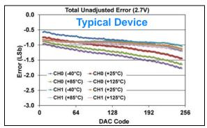
**FIGURE 1-530:** Total Unadjusted Error  $(V_{OUT})$  vs. DAC Code, and Temperature (Dual Channel - **MCP48FXB02**) (8-bit:  $V_{DD} = 2.7V$ ,  $V_{REF} = 1V$ , VRxB:VRxA = '11'  $(V_{REF} Buffered)$ , Gx = '0' (1x)).
