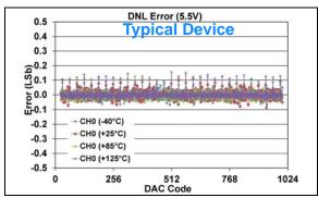
FIGURE 1-376: DNL Error vs. DAC Code, and Temperature (Code 25 - 1000) (Single Channel - MCP48FXB11) (10-bit:  $V_{DD} = 5.5V$ ,  $V_{REF} = 1V$ , VRxB:VRxA = '11' ( $V_{RFF}$  Buffered), Gx = '1' (2x).
