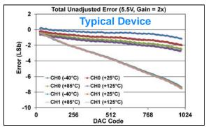
**FIGURE 1-313:** Total Unadjusted Error  $(V_{OUT})$  vs. DAC Code, and Temperature (Dual Channel - **MCP48FXB12**) (10-bit:  $V_{DD} = 5.5V$ ,  $V_{REF} = 2.048V$ ,  $VRxB:VRxA = '10' (V_{REF} Unbuffered)$ , Gx = '1' (2x)).
