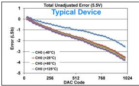
**FIGURE 1-220:** Total Unadjusted Error  $(V_{OUT})$  vs. DAC Code, and Temperature (Single Channel - **MCP48FXB11**)  $(10\text{-bit}: V_{DD} = 5.5V, VRxB: VRxA = '00' (V_{DD}), Gx = '0' (1x)).$
