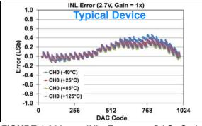
FIGURE 1-390: INL Error vs. DAC Code, and Temperature (Code 25 - 1000) (Single Channel - MCP48FXB11) (10-bit:  $V_{DD} = 2.7V$ ,  $V_{REF} = 2.048V$ ,  $VRxB:VRxA = '11' (V_{REF} Buffered)$ , Gx = '0' (1x)).
