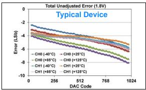
**FIGURE 1-351:** Total Unadjusted Error  $(V_{OUT})$  vs. DAC Code, and Temperature (Dual Channel - **MCP48FXB12**)  $(10\text{-bit: }V_{DD} = 1.8V, V_{REF} = 1V, VRxB:VRxA = '11' (V_{RFF} Buffered), <math>Gx = '0' (1x)$ ).
