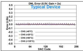
FIGURE 1-574: DNL Error vs. DAC Code, and Temperature (Code 6 - 250) (Single Channel - MCP48FXB01) (8-bit:  $V_{DD} = 5.5V$ ,  $V_{REF} = 2.048V$ ,  $VRxB:VRxA = '11' (V_{REF} Buffered)$ , Gx = '1' (2x)).
