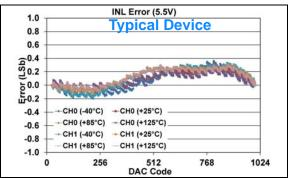
FIGURE 1-337: INL Error vs. DAC Code, and Temperature (Code 25 - 1000) (Dual Channel - MCP48FXB12) (10-bit:  $V_{DD} = 5.5V$ ,  $V_{REF} = V_{DD}$ ,  $VRxB:VRxA = '11' (V_{REF} Buffered)$ , Gx = '0' (1x)).
