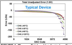
**FIGURE 1-42:** Total Unadjusted Error  $(V_{OUT})$  vs. DAC Code, and Temperature (Single Channel - **MCP48FXB21**)  $(12\text{-bit}: V_{DD} = 1.8V, VRxB:VRxA = '00' (V_{DD}), Gx = '0' (1x)),$  (see **Appendix B.1** for additional information).
