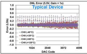
FIGURE 1-71: DNL Error vs. DAC Code, and Temperature (Code 100 - 4000) (Single Channel - MCP48FXB21) (12-bit:  $V_{DD} = 5.5V$ , VRxB:VRxA = '01' (Bandgap), Gx = '0' (1x)).
