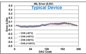
FIGURE 1-514: INL Error vs. DAC Code, and Temperature (Code 6 - 250) (Single Channel - MCP48FXB01) (8-bit:  $V_{DD} = 5.5V$ ,  $V_{REF} = V_{DD}$ ,  $VRxB:VRxA = '11' (V_{REF} Buffered)$ , Gx = '0' (1x)).
