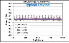
**FIGURE 1-396:** DNL Error vs. DAC Code, and Temperature (Code 25 - 1000) (Single Channel - **MCP48FXB11**) (10-bit:  $V_{DD} = 2.7V$ ,  $V_{REF} = 2.048V$ ,  $VRxB:VRxA = '11' (V_{REF} Buffered)$ , Gx = '0' (1x)).
