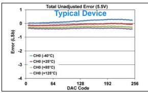
**FIGURE 1-544:** Total Unadjusted Error  $(V_{OUT})$  vs. DAC Code, and Temperature (Single Channel - **MCP48FXB01**) (8-bit:  $V_{DD} = 5.5V$ ,  $V_{REF} = 1V$ ,  $V_{RXB}$ :  $V_{RXA} = '11'$  ( $V_{RFF}$  Buffered),  $G_{X} = '1'$  ( $Z_{X}$ ).
