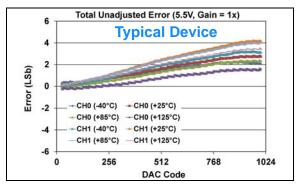
**FIGURE 1-242:** Total Unadjusted Error  $(V_{OUT})$  vs. DAC Code, and Temperature (Dual Channel - **MCP48FXB12**) (10-bit:  $V_{DD} = 5.5V$ , VRxB:VRxA = '01' (Bandgap), Gx = '0' (1x)).
