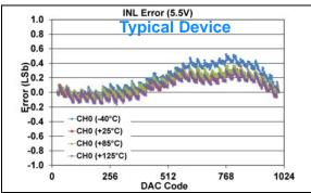
**FIGURE 1-370:** INL Error vs. DAC Code, and Temperature (Code 25 - 1000) (Single Channel - **MCP48FXB11**) (10-bit:  $V_{DD} = 5.5V$ ,  $V_{REF} = 1V$ , VRxB:VRxA = '11' ( $V_{RFF}$  Buffered), Gx = '1' (2x)).
