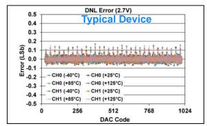
FIGURE 1-308: DNL Error vs. DAC Code, and Temperature (Code 25 - 1000) (Dual Channel - MCP48FXB12) (10-bit:  $V_{DD} = 2.7V$ ,  $V_{REF} = 1V$ , VRxB:VRxA = '10' ( $V_{REF}$  Unbuffered), Gx = '1' (2x).
