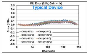
FIGURE 1-428: INL Error vs. DAC Code, and Temperature (Code 6 - 250) (Dual Channel - MCP48FXB02) (8-bit:  $V_{DD} = 5.5V$ , VRxB:VRxA = '01' (Bandgap), Gx = '0' (1x)).
