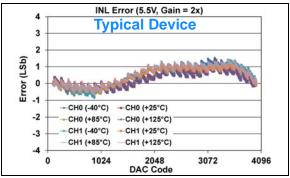
FIGURE 1-211: INL Error vs. DAC Code, and Temperature (Code 100 - 4000) (Dual Channel - MCP48FXB22) (12-bit:  $V_{DD} = 5.5V$ ,  $V_{REF} = 2.048V$ ,  $VRxB:VRxA = '11' (V_{REF} Buffered)$ , Gx = '1' (2x)).
