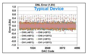
**FIGURE 1-111:** DNL Error vs. DAC Code, and Temperature (Code 100 - 4000) (Dual Channel - **MCP48FXB22**) (12-bit:  $V_{DD} = 1.8V$ ,  $V_{REF} = 1V$ , VRxB:VRxA = '10' ( $V_{REF}$  Unbuffered), Gx = '0' (1x)).
