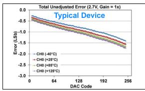
**FIGURE 1-492:** Total Unadjusted Error  $(V_{OUT})$  vs. DAC Code, and Temperature (Single Channel - **MCP48FXB01**) (8-bit:  $V_{DD} = 2.7V$ ,  $V_{REF} = 2.048V$ ,  $VRxB:VRxA = '10' (V_{REF} Unbuffered)$ , Gx = '0' (1x)).
