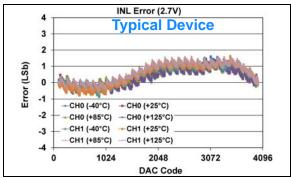
**FIGURE 1-194:** INL Error vs. DAC Code, and Temperature (Code 100 - 4000) (Dual Channel - **MCP48FXB22**) (12-bit:  $V_{DD} = 2.7V$ ,  $V_{REF} = 1V$ , VRxB:VRxA = '11' ( $V_{RFF}$  Buffered), Gx = '1' (2x).
