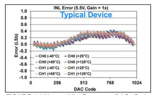
FIGURE 1-392: INL Error vs. DAC Code, and Temperature (Code 25 - 1000) (Dual Channel - MCP48FXB12) (10-bit:  $V_{DD} = 5.5V$ ,  $V_{REF} = 2.048V$ ,  $VRxB:VRxA = '11' (V_{REF} Buffered)$ , Gx = '0' (1x)).
