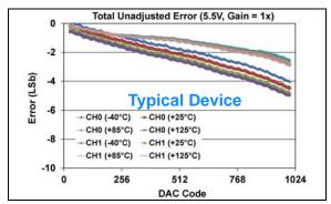
**FIGURE 1-314:** Total Unadjusted Error  $(V_{OUT})$  vs. DAC Code, and Temperature (Dual Channel - **MCP48FXB12**)  $(10\text{-bit}: V_{DD} = 5.5\text{V}, V_{REF} = 2.048\text{V}, VRxB:VRxA = '10' (V_{REF} Unbuffered), Gx = '0' (1x)).$
