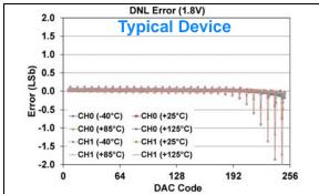
**FIGURE 1-417:** DNL Error vs. DAC Code, and Temperature (Code 6 - 250) (Dual Channel - **MCP48FXB02**) (8-bit:  $V_{DD} = 1.8V$ ,  $VRxB:VRxA = '00' (V_{DD})$ , Gx = '0' (1x)), (see **Appendix B.1** for additional information).
