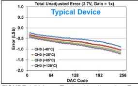
**FIGURE 1-564:** Total Unadjusted Error  $(V_{OUT})$  vs. DAC Code, and Temperature (Single Channel - **MCP48FXB01**)  $(8\text{-bit}: V_{DD} = 2.7V, V_{REF} = 2.048V, VRxB:VRxA = '11' (V_{REF} Buffered), Gx = '0' (1x)).$
