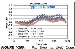
and Temperature (Code 25 - 1000) (Dual Channel - MCP48FXB12) (10-bit:  $V_{DD} = 2.7V$ ,  $V_{REF} = V_{DD}$ ,  $VRXB:VRXA = '10' (V_{REF} Unbuffered)$ , GX = '0' (1x)).
