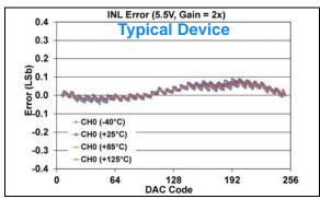
FIGURE 1-568: INL Error vs. DAC Code, and Temperature (Code 6 - 250) (Single Channel - MCP48FXB01) (8-bit:  $V_{DD} = 5.5V$ ,  $V_{REF} = 2.048V$ ,  $VRxB:VRxA = '11' (V_{REF} Buffered)$ , Gx = '1' (2x)).
