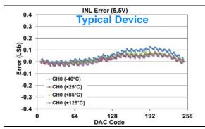
**FIGURE 1-550:** INL Error vs. DAC Code, and Temperature (Code 6 - 250) (Single Channel - **MCP48FXB01**) (8-bit:  $V_{DD} = 5.5V$ ,  $V_{REF} = 1V$ ,  $V_{RXB}:V_{RXA} = '11'$  ( $V_{REF}$  Buffered),  $G_{X} = '1'$  ( $Z_{X}$ ).
