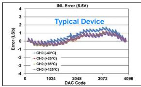
**FIGURE 1-46:** INL Error vs. DAC Code, and Temperature (Code 100 - 4000) (Single Channel - **MCP48FXB21**) (12-bit:  $V_{DD} = 5.5V$ ,  $VRxB:VRxA = '00' (V_{DD})$ , Gx = '0' (1x)).
