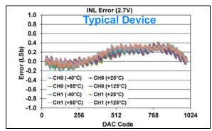
FIGURE 1-284: INL Error vs. DAC Code, and Temperature (Code 25 - 1000) (Dual Channel - MCP48FXB12) (10-bit:  $V_{DD} = 2.7V$ ,  $V_{REF} = 1V$ , VRxB:VRxA = '10' ( $V_{REF}$  Unbuffered), Gx = '0' (1x)).
