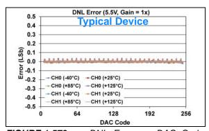
FIGURE 1-578: DNL Error vs. DAC Code, and Temperature (Code 6 - 250) (Dual Channel - MCP48FXB02) (8-bit:  $V_{DD} = 5.5V$ ,  $V_{REF} = 2.048V$ ,  $VRxB:VRxA = '11' (V_{RFF} Buffered)$ , Gx = '0' (1x)).
