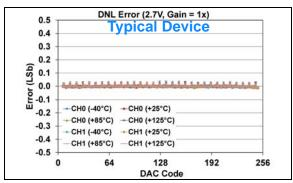
**FIGURE 1-507:** DNL Error vs. DAC Code, and Temperature (Code 6 - 250) (Dual Channel - **MCP48FXB02**) (8-bit:  $V_{DD} = 2.7V$ ,  $V_{REF} = 2.048V$ ,  $VRxB:VRxA = '10' (V_{REF} Unbuffered)$ , Gx = '0' (1x)).
