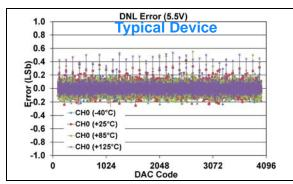
FIGURE 1-178: DNL Error vs. DAC Code, and Temperature (Code 100 - 4000) (Single Channel - MCP48FXB21) (12-bit:  $V_{DD} = 5.5V$ ,  $V_{REF} = 1V$ ,  $V_{RXB}$ :  $V_{RXA} = '11'$  ( $V_{RFF}$  Buffered),  $G_{X} = '0'$  (1x)).
