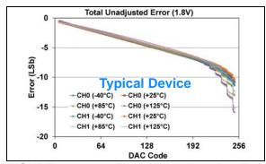
**FIGURE 1-513:** Total Unadjusted Error  $(V_{OUT})$  vs. DAC Code, and Temperature (Dual Channel - **MCP48FXB02**) (8-bit:  $V_{DD} = 1.8$ V,  $V_{REF} = V_{DD}$ ,  $VRXB:VRXA = '11' (V_{REF} Buffered)$ , GX = '0' (1x)), (see **Appendix B.4** for additional information).
