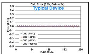
FIGURE 1-430: DNL Error vs. DAC Code, and Temperature (Code 6 - 250) (Single Channel - MCP48FXB01) (8-bit:  $V_{DD} = 5.5V$ , VRxB:VRxA = '01' (Bandgap), Gx = '1' (2x)).
