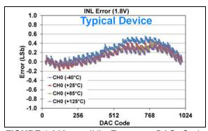
**FIGURE 1-282:** INL Error vs. DAC Code, and Temperature (Code 25 - 1000) (Single Channel - **MCP48FXB11**) (10-bit:  $V_{DD} = 1.8V$ ,  $V_{REF} = 1V$ , VRxB:VRxA = '10' ( $V_{REF}$  Unbuffered), Gx = '0' (1x)).
