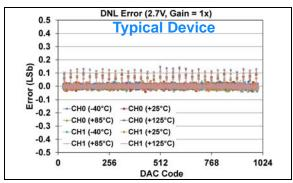
FIGURE 1-327: DNL Error vs. DAC Code, and Temperature (Code 25 - 1000) (Dual Channel - MCP48FXB12) (10-bit:  $V_{DD} = 2.7V$ ,  $V_{REF} = 2.048V$ ,  $VRxB:VRxA = '10' (V_{REF} Unbuffered)$ , Gx = '0' (1x)).
