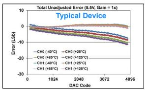
**FIGURE 1-206:** Total Unadjusted Error  $(V_{OUT})$  vs. DAC Code, and Temperature (Dual Channel - **MCP48FXB22**) (12-bit:  $V_{DD} = 5.5V$ ,  $V_{REF} = 2.048V$ ,  $VRxB:VRxA = '11' (V_{REF} Buffered)$ , Gx = '0' (1x)).
