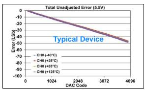
**FIGURE 1-148:** Total Unadjusted Error  $(V_{OUT})$  vs. DAC Code, and Temperature (Single Channel - **MCP48FXB21**) (**12-bit**:  $V_{DD} = 5.5V$ ,  $V_{REF} = V_{DD}$ , VRxB:VRxA = '11'  $(V_{REF}$  Buffered), Gx = '0' (1x)).
