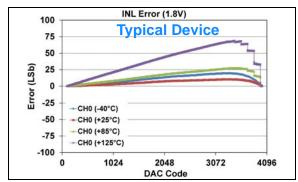
**FIGURE 1-84:** INL Error vs. DAC Code, and Temperature (Code 100 - 4000) (Single Channel - **MCP48FXB21**) (12-bit:  $V_{DD} = 1.8V$ ,  $V_{REF} = V_{DD}$ , VRxB:VRxA = '10' ( $V_{REF}$  Unbuffered), Gx = '0' (1x)), (see **Appendix B.2** for additional information).
