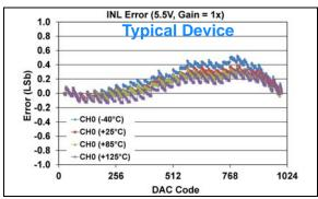
**FIGURE 1-245:** INL Error vs. DAC Code, and Temperature (Code 25 - 1000) (Single Channel - **MCP48FXB11**) (10-bit:  $V_{DD} = 5.5V$ , VRxB:VRxA = '01' (Bandgap), Gx = '0' (1x)).
