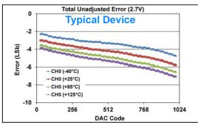
**FIGURE 1-347:** Total Unadjusted Error  $(V_{OUT})$  vs. DAC Code, and Temperature (Single Channel - **MCP48FXB11**)  $(10\text{-bit}: V_{DD} = 2.7V, V_{REF} = 1V, VRxB:VRxA = '11' <math>(V_{REF} \text{ Buffered}), Gx = '0' (1x)).$
