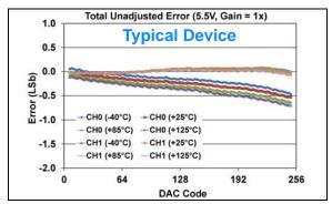
**FIGURE 1-566:** Total Unadjusted Error  $(V_{OUT})$  vs. DAC Code, and Temperature (Dual Channel - **MCP48FXB02**) (8-bit:  $V_{DD} = 5.5V$ ,  $V_{REF} = 2.048V$ ,  $VRxB:VRxA = '11' (V_{REF} Buffered)$ , Gx = '0' (1x)).
