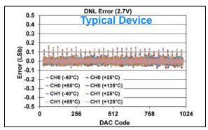
**FIGURE 1-362:** DNL Error vs. DAC Code, and Temperature (Code 25 - 1000) (Dual Channel - **MCP48FXB12**) (10-bit:  $V_{DD} = 2.7V$ ,  $V_{REF} = 1V$ , VRxB:VRxA = '11' ( $V_{RFF}$  Buffered), Gx = '0' (1x)).
