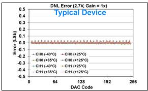
FIGURE 1-435: DNL Error vs. DAC Code, and Temperature (Code 6 - 250) (Dual Channel - MCP48FXB02) (8-bit:  $V_{DD} = 2.7V$ , VRxB:VRxA = '01' (Bandgap), Gx = '0' (1x)).
