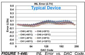
**FIGURE 1-446:** INL Error vs. DAC Code, and Temperature (Code 6 - 250) (Dual Channel - **MCP48FXB02**) (8-bit:  $V_{DD} = 2.7V$ ,  $V_{REF} = V_{DD}$ ,  $VRxB:VRxA = '10' (V_{RFF} Unbuffered)$ , Gx = '0' (1x)).
