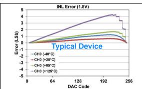
**FIGURE 1-444:** INL Error vs. DAC Code, and Temperature (Code 6 - 250) (Single Channel - **MCP48FXB01**) (8-bit:  $V_{DD} = 1.8V$ ,  $V_{REF} = V_{DD}$ ,  $VRxB:VRxA = '10' (V_{REF} Unbuffered)$ , Gx = '0' (1x)), (see **Appendix B.2** for additional information).
