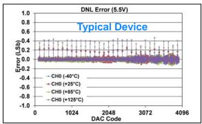
FIGURE 1-52: DNL Error vs. DAC Code, and Temperature (Code 100 - 4000) (Single Channel - MCP48FXB21) (12-bit:  $V_{DD} = 5.5V$ ,  $VRxB:VRxA = '00' (V_{DD})$ , Gx = '0' (1x)).
