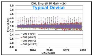
FIGURE 1-70: DNL Error vs. DAC Code, and Temperature (Code 100 - 4000) (Single Channel - MCP48FXB21) (12-bit:  $V_{DD} = 5.5V$ , VRxB:VRxA = '01' (Bandgap), Gx = '1' (2x)).
