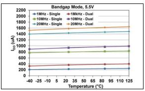
**FIGURE 1-15:** Average Device Supply Current vs.  $F_{SCK}$  Frequency, Voltage and Temperature, VRxB:VRxA = '01', (Bandgap mode).
