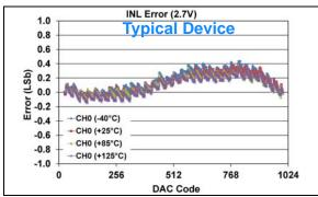
**FIGURE 1-299:** INL Error vs. DAC Code, and Temperature (Code 25 - 1000) (Single Channel - **MCP48FXB11**) (10-bit:  $V_{DD} = 2.7V$ ,  $V_{REF} = 1V$ ,  $V_{RXB}$ : $V_{RXA} = '10'$  ( $V_{REF}$  Unbuffered),  $G_{X} = '1'$  (2x)).
