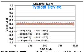
FIGURE 1-272: DNL Error vs. DAC Code, and Temperature (Code 25 - 1000) (Dual Channel - MCP48FXB12) (10-bit:  $V_{DD} = 2.7V$ ,  $V_{REF} = V_{DD}$ ,  $VRxB:VRxA = '10' (V_{RFF} Unbuffered)$ , Gx = '0' (1x)).
