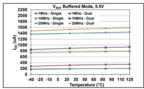
**FIGURE 1-24:** Average Device Supply Current vs.  $F_{SCK}$  Frequency, Voltage and Temperature, VRxB:VRxA = '11' ( $V_{RFF}$  Buffered mode).
