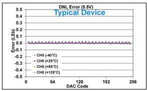
FIGURE 1-520: DNL Error vs. DAC Code, and Temperature (Code 6 - 250) (Single Channel - MCP48FXB01) (8-bit:  $V_{DD} = 5.5V$ ,  $V_{REF} = V_{DD}$ ,  $VRxB:VRxA = '11' (V_{REF} Buffered)$ , Gx = '0' (1x)).
