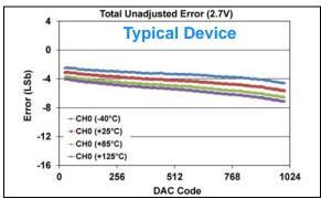
**FIGURE 1-293:** Total Unadjusted Error  $(V_{OUT})$  vs. DAC Code, and Temperature (Single Channel - **MCP48FXB11**) (10-bit:  $V_{DD} = 2.7V$ ,  $V_{REF} = 1V$ ,  $V_{RXB}$ :  $V_{RXA} = '10'$  ( $V_{RFF}$  Unbuffered),  $V_{RFF} = 1V$ ,  $V_{RXB}$ :  $V_{RXA} = '10'$
