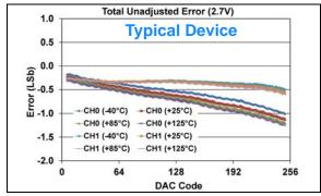
**FIGURE 1-404:** Total Unadjusted Error  $(V_{OUT})$  vs. DAC Code, and Temperature (Dual Channel - **MCP48FXB02**) (8-bit:  $V_{DD} = 2.7V$ ,  $VRxB:VRxA = '00' (V_{DD})$ , Gx = '0' (1x)).
