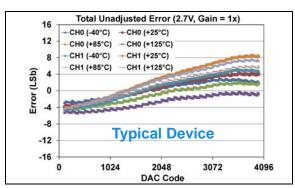
**FIGURE 1-63:** Total Unadjusted Error  $(V_{OUT})$  vs. DAC Code, and Temperature (Dual Channel - **MCP48FXB22**) (12-bit:  $V_{DD} = 2.7V$ , VRxB:VRxA = '01' (Bandgap), Gx = '0' (1x)).
