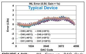
FIGURE 1-212: INL Error vs. DAC Code, and Temperature (Code 100 - 4000) (Dual Channel - MCP48FXB22) (12-bit:  $V_{DD} = 5.5V$ ,  $V_{REF} = 2.048V$ ,  $VRxB:VRxA = '11' (V_{RFF} Buffered)$ , Gx = '0' (1x)).
