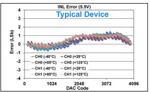
FIGURE 1-157: INL Error vs. DAC Code, and Temperature (Code 100 - 4000) (Dual Channel - MCP48FXB22) (12-bit:  $V_{DD} = 5.5V$ ,  $V_{REF} = V_{DD}$ ,  $VRxB:VRxA = '11' (V_{REF} Buffered)$ , Gx = '0' (1x)).
