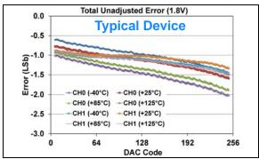
**FIGURE 1-531:** Total Unadjusted Error  $(V_{OUT})$  vs. DAC Code, and Temperature (Dual Channel - **MCP48FXB02**) (8-bit:  $V_{DD} = 1.8V$ ,  $V_{REF} = 1V$ , VRxB:VRxA = '11'  $(V_{REF}$  Buffered), Gx = '0' (1x).
