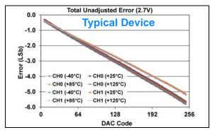
**FIGURE 1-512:** Total Unadjusted Error  $(V_{OUT})$  vs. DAC Code, and Temperature (Dual Channel - **MCP48FXB02**) (8-bit:  $V_{DD} = 2.7V$ ,  $V_{REF} = V_{DD}$ ,  $VRxB:VRxA = '11' (V_{REF} Buffered)$ , Gx = '0' (1x)).
