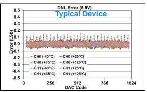
**FIGURE 1-361:** DNL Error vs. DAC Code, and Temperature (Code 25 - 1000) (Dual Channel - **MCP48FXB12**) (10-bit:  $V_{DD} = 5.5V$ ,  $V_{REF} = 1V$ ,  $V_{RXB}$ : $V_{RXA} = '11'$  ( $V_{REF}$  Buffered),  $G_{X} = '0'$  (1x)).
