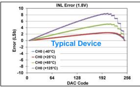
**FIGURE 1-408:** INL Error vs. DAC Code, and Temperature (Code 6 - 250) (Single Channel - **MCP48FXB01**) (8-bit:  $V_{DD} = 1.8V$ ,  $V_{RXB}:V_{RXA} = '00' (V_{DD})$ ,  $G_{X} = '0' (1x)$ ), (see **Appendix B.1** for additional information).
