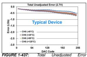
$(V_{OUT})$  vs. DAC Code, and Temperature (Single Channel - **MCP48FXB01**) (8-bit:  $V_{DD} = 2.7V$ ,  $V_{REF} = V_{DD}$ .  $VRxB:VRxA = '10' (V_{REF} Unbuffered)$ , Gx = '0' (1x)).
