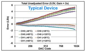
**FIGURE 1-241:** Total Unadjusted Error  $(V_{OUT})$  vs. DAC Code, and Temperature (Dual Channel - **MCP48FXB12**) (10-bit:  $V_{DD} = 5.5V$ , VRxB:VRxA = '01' (Bandgap), Gx = '1' (2x)).
