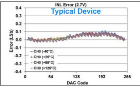
**FIGURE 1-533:** INL Error vs. DAC Code, and Temperature (Code 6 - 250) (Single Channel - **MCP48FXB01**) (8-bit:  $V_{DD} = 2.7V$ ,  $V_{REF} = 1V$ ,  $V_{RXB}:V_{RXA} = '11'$  ( $V_{REF}$  Buffered),  $G_{X} = '0'$  (1x)).
