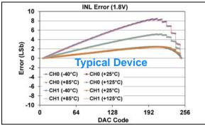
**FIGURE 1-411:** INL Error vs. DAC Code, and Temperature (Code 6 - 250) (Dual Channel - **MCP48FXB02**) (8-bit:  $V_{DD} = 1.8V$ ,  $V_{RXB}:V_{RXA} = '00' (V_{DD})$ ,  $G_{X} = '0' (1x)$ ), (see **Appendix B.1** for additional information).
