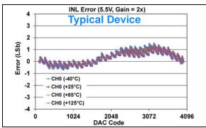
FIGURE 1-208: INL Error vs. DAC Code, and Temperature (Code 100 - 4000) (Single Channel - MCP48FXB21) (12-bit:  $V_{DD} = 5.5V$ ,  $V_{REF} = 2.048V$ ,  $VRxB:VRxA = '11' (V_{REF} Buffered)$ , Gx = '1' (2x)).
