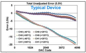
**FIGURE 1-79:** Total Unadjusted Error  $(V_{OUT})$  vs. DAC Code, and Temperature (Dual Channel - **MCP48FXB22**) (12-bit:  $V_{DD} = 5.5V$ ,  $V_{REF} = V_{DD}$ ,  $VRxB:VRxA = '10' (V_{REF} Unbuffered)$ , Gx = '0' (1x)).
