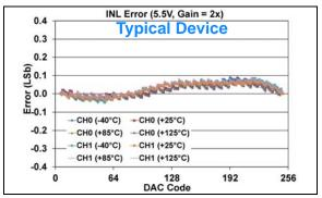
FIGURE 1-571: INL Error vs. DAC Code, and Temperature (Code 6 - 250) (Dual Channel - MCP48FXB02) (8-bit:  $V_{DD} = 5.5V$ ,  $V_{REF} = 2.048V$ ,  $VRxB:VRxA = '11' (V_{REF} Buffered)$ , Gx = '1' (2x)).
