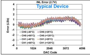
FIGURE 1-104: INL Error vs. DAC Code, and Temperature (Code 100 - 4000) (Dual Channel - MCP48FXB22) (12-bit:  $V_{DD} = 2.7V$ ,  $V_{REF} = 1V$ , VRxB:VRxA = '10' ( $V_{REF}$  Unbuffered), Gx = '0' (1x)).
