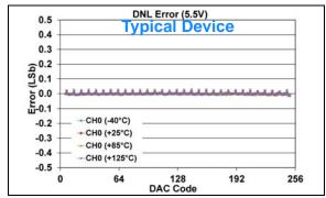
FIGURE 1-412: DNL Error vs. DAC Code, and Temperature (Code 6 - 250) (Single Channel - MCP48FXB01) (8-bit:  $V_{DD} = 5.5V$ ,  $V_{DD} = 5.5V$ ,
