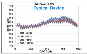
**FIGURE 1-298:** INL Error vs. DAC Code, and Temperature (Code 25 - 1000) (Single Channel - **MCP48FXB11**) (10-bit:  $V_{DD} = 5.5V$ ,  $V_{REF} = 1V$ , VRxB:VRxA = '10' ( $V_{RFF}$  Unbuffered), Gx = '1' (2x)).
