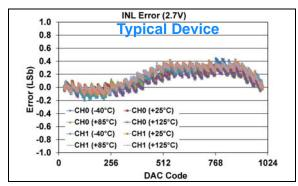
FIGURE 1-356: INL Error vs. DAC Code, and Temperature (Code 25 - 1000) (Dual Channel - MCP48FXB12) (10-bit:  $V_{DD} = 2.7V$ ,  $V_{REF} = 1V$ , VRxB:VRxA = '11' ( $V_{RFF}$  Buffered), Gx = '0' (1x)).
