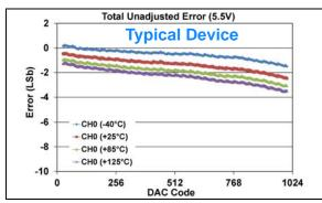
**FIGURE 1-346:** Total Unadjusted Error  $(V_{OUT})$  vs. DAC Code, and Temperature (Single Channel - **MCP48FXB11**)  $(10\text{-bit}: V_{DD} = 5.5V, V_{REF} = 1V, VRxB:VRxA = '11' (V_{RFF} Buffered), <math>Gx = '0' (1x)$ ).
