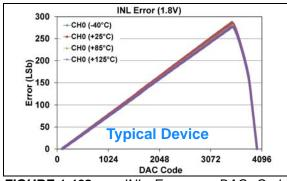
**FIGURE 1-192:** INL Error vs. DAC Code, and Temperature (Code 100 - 4000) (Single Channel - **MCP48FXB21**) (12-bit:  $V_{DD} = 1.8V$ ,  $V_{REF} = 1V$ , VRxB:VRxA = '11' ( $V_{REF}$  Buffered), Gx = '1' (2x)), (see **Appendix B.5** for additional information).
