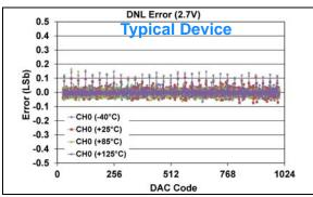
**FIGURE 1-359:** DNL Error vs. DAC Code, and Temperature (Code 25 - 1000) (Single Channel - **MCP48FXB11**) (10-bit:  $V_{DD} = 2.7V$ ,  $V_{REF} = 1V$ ,  $V_{RXB}:V_{RXA} = '11'$  ( $V_{RFF}$  Buffered),  $G_{X} = '0'$  (1x)).
