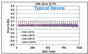
FIGURE 1-341: DNL Error vs. DAC Code, and Temperature (Code 25 - 1000) (Single Channel - MCP48FXB11) (10-bit:  $V_{DD} = 2.7V$ ,  $V_{REF} = V_{DD}$ ,  $VRxB:VRxA = '11' (V_{REF} Buffered)$ , Gx = '0' (1x)).
