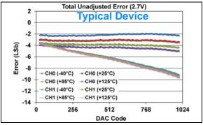
**FIGURE 1-368:** Total Unadjusted Error  $(V_{OUT})$  vs. DAC Code, and Temperature (Dual Channel - **MCP48FXB12**)  $(10\text{-bit}: V_{DD} = 2.7V, V_{REF} = 1V, VRxB:VRxA = '11' <math>(V_{REF} \text{ Buffered}), Gx = '1' (2x)).$
