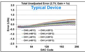
**FIGURE 1-423:** Total Unadjusted Error  $(V_{OUT})$  vs. DAC Code, and Temperature (Dual Channel - **MCP48FXB02**) (8-bit:  $V_{DD} = 2.7V$ , VRxB:VRxA = '01' (Bandgap), Gx = '0' (1x)).
