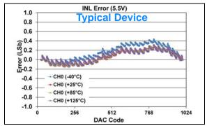
FIGURE 1-226: INL Error vs. DAC Code, and Temperature (Code 25 - 1000) (Single Channel - MCP48FXB11) (10-bit:  $V_{DD} = 5.5V$ ,  $VRxB:VRxA = '00' (V_{DD})$ , Gx = '0' (1x)).
