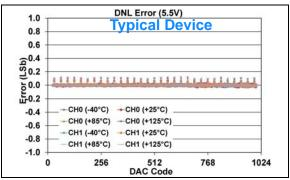
FIGURE 1-235: DNL Error vs. DAC Code, and Temperature (Code 25 - 1000) (Dual Channel - MCP48FXB12) (10-bit:  $V_{DD} = 5.5V$ ,  $VRxB:VRxA = '00' (V_{DD})$ , Gx = '0' (1x)).
