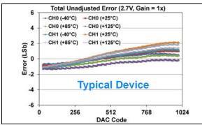
**FIGURE 1-243:** Total Unadjusted Error  $(V_{OUT})$  vs. DAC Code, and Temperature (Dual Channel - **MCP48FXB12**) (10-bit:  $V_{DD} = 2.7V$ , VRxB:VRxA = '01' (Bandgap), Gx = '0' (1x)).
