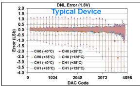
FIGURE 1-57: DNL Error vs. DAC Code, and Temperature (Code 100 - 4000) (Dual Channel - MCP48FXB22) (12-bit:  $V_{DD} = 1.8V$ ,  $VRxB:VRxA = '00' (V_{DD})$ , Gx = '0' (1x)), (see Appendix B.1 for additional information).
