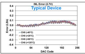
FIGURE 1-479: INL Error vs. DAC Code, and Temperature (Code 6 - 250) (Single Channel - MCP48FXB01) (8-bit:  $V_{DD} = 2.7V$ ,  $V_{REF} = 1V$ , VRxB:VRxA = '10' ( $V_{REF}$  Unbuffered), Gx = '1' (2x).
