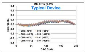
FIGURE 1-554: INL Error vs. DAC Code, and Temperature (Code 6 - 250) (Dual Channel - MCP48FXB02) (8-bit:  $V_{DD} = 2.7V$ ,  $V_{REF} = 1V$ , VRxB:VRxA = '11' ( $V_{RFF}$  Buffered), Gx = '1'(2x)).
