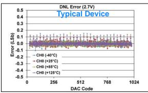
**FIGURE 1-287:** DNL Error vs. DAC Code, and Temperature (Code 25 - 1000) (Single Channel - **MCP48FXB11**) (10-bit:  $V_{DD} = 2.7V$ ,  $V_{REF} = 1V$ , VRxB:VRxA = '10' ( $V_{RFF}$  Unbuffered), Gx = '0' (1x)).
