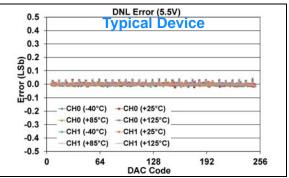
**FIGURE 1-469:** DNL Error vs. DAC Code, and Temperature (Code 6 - 250) (Dual Channel - **MCP48FXB02**) (8-bit:  $V_{DD} = 5.5V$ ,  $V_{REF} = 1V$ ,  $V_{RXB}:V_{RXA} = '10'$  ( $V_{REF}$  Unbuffered),  $G_{X} = '0'$  (1x)).
