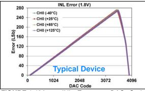
**FIGURE 1-120:** INL Error vs. DAC Code, and Temperature (Code 100 - 4000) (Single Channel - **MCP48FXB21**) (12-bit:  $V_{DD} = 1.8V$ ,  $V_{REF} = 1V$ , VRxB:VRxA = '10' ( $V_{REF}$  Unbuffered), Gx = '1' (2x)), (see **Appendix B.3** for additional information).
