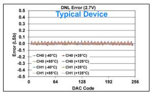
FIGURE 1-470: DNL Error vs. DAC Code, and Temperature (Code 6 - 250) (Dual Channel - MCP48FXB02) (8-bit:  $V_{DD} = 2.7V$ ,  $V_{REF} = 1V$ , VRxB:VRxA = '10' ( $V_{RFF}$  Unbuffered), Gx = '0' (1x)).
