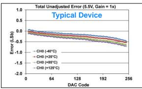
**FIGURE 1-563:** Total Unadjusted Error  $(V_{OUT})$  vs. DAC Code, and Temperature (Single Channel - **MCP48FXB01**) (8-bit:  $V_{DD} = 5.5V$ ,  $V_{REF} = 2.048V$ ,  $VRxB:VRxA = '11' (V_{REF} Buffered)$ , Gx = '0' (1x)).
