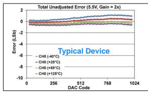
**FIGURE 1-382:** Total Unadjusted Error  $(V_{OUT})$  vs. DAC Code, and Temperature (Single Channel - **MCP48FXB11**)  $(10\text{-bit}: V_{DD} = 5.5V, V_{REF} = 2.048V, VRxB:VRxA = '11' <math>(V_{REF} \text{ Buffered}), Gx = '1' (2x)).$
