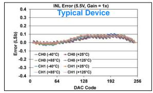
FIGURE 1-572: INL Error vs. DAC Code, and Temperature (Code 6 - 250) (Dual Channel - MCP48FXB02) (8-bit:  $V_{DD} = 5.5V$ ,  $V_{REF} = 2.048V$ ,  $VRxB:VRxA = '11' (V_{RFF} Buffered)$ , Gx = '0' (1x)).
