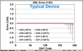
FIGURE 1-453: DNL Error vs. DAC Code, and Temperature (Code 6 - 250) (Dual Channel - MCP48FXB02) (8-bit:  $V_{DD} = 1.8V$ ,  $V_{REF} = V_{DD}$ ,  $VRxB:VRxA = '10' (V_{REF} Unbuffered)$ , Gx = '0' (1x), (see Appendix B.2 for additional information).
