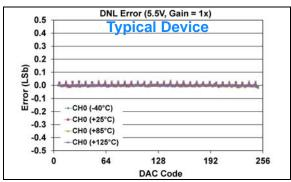
FIGURE 1-575: DNL Error vs. DAC Code, and Temperature (Code 6 - 250) (Single Channel - MCP48FXB01) (8-bit:  $V_{DD} = 5.5V$ ,  $V_{REF} = 2.048V$ ,  $VRxB:VRxA = '11' (V_{REF} Buffered)$ , Gx = '0' (1x)).
