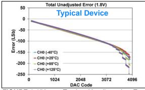
**FIGURE 1-150:** Total Unadjusted Error  $(V_{OUT})$  vs. DAC Code, and Temperature (Single Channel - **MCP48FXB21**)  $(12\text{-bit}: V_{DD} = 1.8V, V_{REF} = V_{DD}, VRXB:VRXA = '11' (V_{REF} Buffered), <math>Gx = '0' (1x)$ ), (see **Appendix B.4** for additional information).
