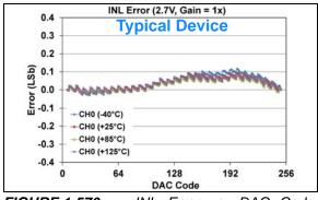
FIGURE 1-570: INL Error vs. DAC Code, and Temperature (Code 6 - 250) (Single Channel - MCP48FXB01) (8-bit:  $V_{DD} = 2.7V$ ,  $V_{REF} = 2.048V$ ,  $VRxB:VRxA = '11' (V_{REF} Buffered)$ , Gx = '0' (1x)).
