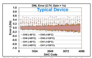
FIGURE 1-75: DNL Error vs. DAC Code, and Temperature (Code 100 - 4000) (Dual Channel - MCP48FXB22) (12-bit:  $V_{DD} = 2.7V$ , VRxB:VRxA = '01' (Bandgap), Gx = '0' (1x)).
