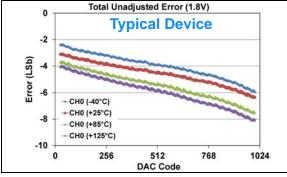
**FIGURE 1-348:** Total Unadjusted Error  $(V_{OUT})$  vs. DAC Code, and Temperature (Single Channel - **MCP48FXB11**) (10-bit:  $V_{DD} = 1.8V$ ,  $V_{REF} = 1V$ ,  $V_{RXB}$ : $V_{RXA} = '11'$  ( $V_{RFF}$  Buffered),  $G_{X} = '0'$  ( $I_{X}$ ).
