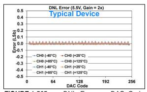
**FIGURE 1-505:** DNL Error vs. DAC Code, and Temperature (Code 6 - 250) (Dual Channel - **MCP48FXB02**) (8-bit:  $V_{DD} = 5.5V$ ,  $V_{REF} = 2.048V$ ,  $VRxB:VRxA = '10' (V_{REF} Unbuffered)$ , Gx = '1' (2x)).
