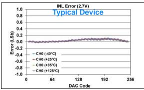
FIGURE 1-407: INL Error vs. DAC Code, and Temperature (Code 6 - 250) (Single Channel - MCP48FXB01) (8-bit:  $V_{DD} = 2.7V$ ,  $VRxB:VRxA = '00' (V_{DD})$ , Gx = '0' (1x)).
