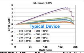
**FIGURE 1-447:** INL Error vs. DAC Code, and Temperature (Code 6 - 250) (Dual Channel - **MCP48FXB02**) (8-bit:  $V_{DD} = 1.8V$ ,  $V_{REF} = V_{DD}$ ,  $VRxB:VRxA = '10' (V_{REF} Unbuffered)$ , Gx = '0' (1x)),
