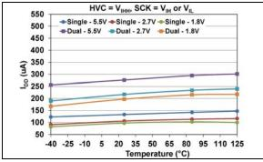
**FIGURE 1-6:** Average Device Current with High Voltage Command Pin (HVC) =  $V_{IHH}$  vs. Temperature and Voltage, SCK =  $V_{IH}$  or  $V_{IL}$ .
