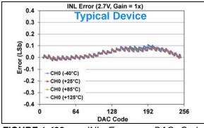
**FIGURE 1-498:** INL Error vs. DAC Code, and Temperature (Code 6 - 250) (Single Channel - **MCP48FXB01**) (8-bit:  $V_{DD} = 2.7V$ ,  $V_{REF} = 2.048V$ ,  $VRxB:VRxA = '10' (V_{REF} Unbuffered)$ , Gx = '0' (1x)).
