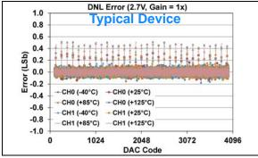
FIGURE 1-219: DNL Error vs. DAC Code, and Temperature (Code 100 - 4000) (Dual Channel - MCP48FXB22) (12-bit:  $V_{DD} = 2.7V$ ,  $V_{REF} = 2.048V$ ,  $VRxB:VRxA = '11' (V_{REF} Buffered)$ , Gx = '0' (1x)).
