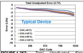
**FIGURE 1-257:** Total Unadjusted Error  $(V_{OUT})$  vs. DAC Code, and Temperature (Single Channel - **MCP48FXB11**)  $(10\text{-bit}: V_{DD} = 2.7V, V_{REF} = V_{DD}, VRxB:VRxA = '10' (V_{REF} Unbuffered), Gx = '0' (1x)).$
