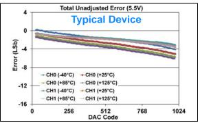
**FIGURE 1-277:** Total Unadjusted Error  $(V_{OUT})$  vs. DAC Code, and Temperature (Dual Channel - **MCP48FXB12**) (10-bit:  $V_{DD} = 5.5V$ ,  $V_{REF} = 1V$ , VRxB:VRxA = '10' ( $V_{RFF}$  Unbuffered), Gx = '0' (1x).
