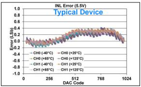
**FIGURE 1-355:** INL Error vs. DAC Code, and Temperature (Code 25 - 1000) (Dual Channel - **MCP48FXB12**) (10-bit:  $V_{DD} = 5.5V$ ,  $V_{REF} = 1V$ , VRXB:VRXA = '11' ( $V_{RFF}$  Buffered), GX = '0' (1x)).
