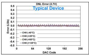
FIGURE 1-467: DNL Error vs. DAC Code, and Temperature (Code 6 - 250) (Single Channel - MCP48FXB01) (8-bit:  $V_{DD} = 2.7V$ ,  $V_{REF} = 1V$ , VRxB:VRxA = '10' ( $V_{REF}$  Unbuffered), Gx = '0' (1x)).
