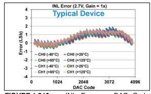
FIGURE 1-213: INL Error vs. DAC Code, and Temperature (Code 100 - 4000) (Dual Channel - MCP48FXB22) (12-bit:  $V_{DD} = 2.7V$ ,  $V_{REF} = 2.048V$ ,  $VRxB:VRxA = '11' (V_{REF} Buffered)$ , Gx = '0' (1x)).
