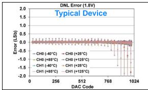
**FIGURE 1-345:** DNL Error vs. DAC Code, and Temperature (Code 25 - 1000) (Dual Channel - **MCP48FXB12**) (10-bit:  $V_{DD} = 1.8V$ ,  $V_{REF} = V_{DD}$ , VRXB:VRXA = '11' ( $V_{REF}$  Buffered), GX = '0' (1x)), (see **Appendix B.4** for additional information).
