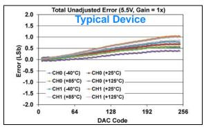
**FIGURE 1-422:** Total Unadjusted Error  $(V_{OUT})$  vs. DAC Code, and Temperature (Dual Channel - **MCP48FXB02**) (8-bit:  $V_{DD} = 5.5V$ , VRxB:VRxA = '01' (Bandgap), Gx = '0' (1x)).
