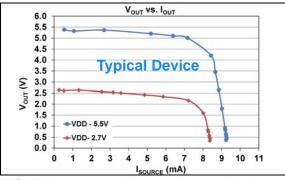
**FIGURE 1-35:**  $V_{OUT}$  vs.  $I_{OUT}$  and Voltage (at +25°C).
