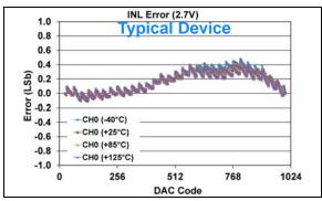
**FIGURE 1-227:** INL Error vs. DAC Code, and Temperature (Code 25 - 1000) (Single Channel - **MCP48FXB11**) (10-bit:  $V_{DD} = 2.7V$ ,  $VRxB:VRxA = '00' (V_{DD})$ , Gx = '0' (1x)).
