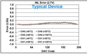
FIGURE 1-410: INL Error vs. DAC Code, and Temperature (Code 6 - 250) (Dual Channel - MCP48FXB02) (8-bit:  $V_{DD} = 2.7V$ ,  $VRxB:VRxA = '00' (V_{DD})$ , Gx = '0' (1x)).
