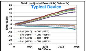
**FIGURE 1-61:** Total Unadjusted Error  $(V_{OUT})$  vs. DAC Code, and Temperature (Dual Channel - **MCP48FXB22**) (12-bit:  $V_{DD} = 5.5V$ , VRxB:VRxA = '01' (Bandgap), Gx = '1' (2x)).
