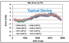
FIGURE 1-50: INL Error vs. DAC Code, and Temperature (Code 100 - 4000) (Dual Channel - MCP48FXB22) (12-bit:  $V_{DD} = 2.7V$ ,  $VRxB:VRxA = '00' (V_{DD})$ , Gx = '0' (1x)).
