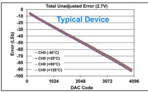
**FIGURE 1-149:** Total Unadjusted Error  $(V_{OUT})$  vs. DAC Code, and Temperature (Single Channel - **MCP48FXB21**) (12-bit:  $V_{DD} = 2.7V$ ,  $V_{REF} = V_{DD}$ ,  $VRXB:VRXA = '11' (V_{REF} Buffered)$ , GX = '0' (1x)).
