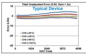
**FIGURE 1-202:** Total Unadjusted Error  $(V_{OUT})$  vs. DAC Code, and Temperature (Single Channel - **MCP48FXB21**) (**12-bit**:  $V_{DD} = 5.5V$ ,  $V_{REF} = 2.048V$ , VRxB:VRxA = '11'  $(V_{REF}$  Buffered), Gx = '1' (2x)).
