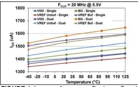
**FIGURE 1-1:** Average Device Supply Active Current  $(I_{DDA})$  (at 5.5V and  $F_{SCK} = 20 \text{ MHz})$  vs. Temperature and DAC Reference Voltage Mode.
