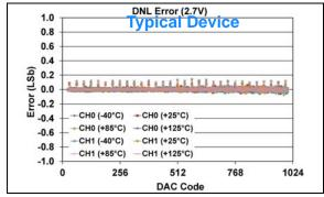
FIGURE 1-236: DNL Error vs. DAC Code, and Temperature (Code 25 - 1000) (Dual Channel - MCP48FXB12) (10-bit:  $V_{DD} = 2.7V$ ,  $VRxB:VRxA = '00' (V_{DD})$ , Gx = '0' (1x)).
