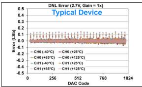
**FIGURE 1-255:** DNL Error vs. DAC Code, and Temperature (Code 25 - 1000) (Dual Channel - **MCP48FXB12**) (10-bit:  $V_{DD} = 2.7V$ , VRxB:VRxA = '01' (Bandgap), Gx = '0' (1x)).
