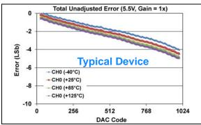
**FIGURE 1-311:** Total Unadjusted Error  $(V_{OUT})$  vs. DAC Code, and Temperature (Single Channel - **MCP48FXB11**)  $(10\text{-bit}: V_{DD} = 5.5V, V_{REF} = 2.048V, VRxB:VRxA = '10' (V_{RFF} Unbuffered), <math>Gx = '0' (1x)$ ).
