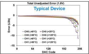
**FIGURE 1-405:** Total Unadjusted Error  $(V_{OUT})$  vs. DAC Code, and Temperature (Dual Channel - **MCP48FXB02**) (8-bit:  $V_{DD} = 1.8V$ ,  $VRxB:VRxA = '00' (V_{DD})$ , Gx = '0' (1x)), (see **Appendix B.1** for additional information).
