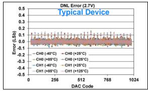
**FIGURE 1-380:** DNL Error vs. DAC Code, and Temperature (Code 25 - 1000) (Dual Channel - **MCP48FXB12**) (10-bit:  $V_{DD} = 2.7V$ ,  $V_{REF} = 1V$ , VRxB:VRxA = '11' ( $V_{RFF}$  Buffered), Gx = '1' (2x).
