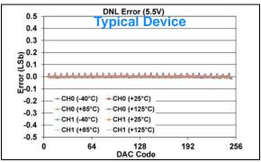
**FIGURE 1-415:** DNL Error vs. DAC Code, and Temperature (Code 6 - 250) (Dual Channel - **MCP48FXB02**) (8-bit:  $V_{DD} = 5.5V$ ,  $V_{RXB}:V_{RXA} = '00' (V_{DD})$ ,  $G_{X} = '0' (1x)$ ).
