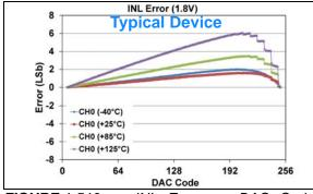
**FIGURE 1-516:** INL Error vs. DAC Code, and Temperature (Code 6 - 250) (Single Channel - **MCP48FXB01**) (8-bit:  $V_{DD} = 1.8V$ ,  $V_{REF} = V_{DD}$ ,  $VRxB:VRxA = '11' (V_{REF} Buffered)$ , Gx = '0' (1x)), (see **Appendix B.4** for additional information).
