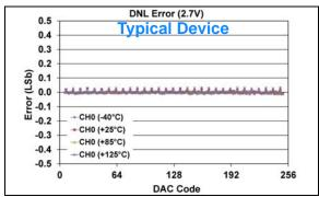
FIGURE 1-521: DNL Error vs. DAC Code, and Temperature (Code 6 - 250) (Single Channel - MCP48FXB01) (8-bit:  $V_{DD} = 2.7V$ ,  $V_{REF} = V_{DD}$ ,  $VRxB:VRxA = '11' (V_{RFF} Buffered)$ , Gx = '0' (1x)).
