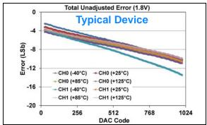
**FIGURE 1-279:** Total Unadjusted Error  $(V_{OUT})$  vs. DAC Code, and Temperature (Dual Channel - **MCP48FXB12**)  $(10\text{-bit: }V_{DD} = 1.8V, V_{REF} = 1V, VRxB:VRxA = '10' (V_{RFF} Unbuffered), <math>Gx = '0' (1x)$ ).
