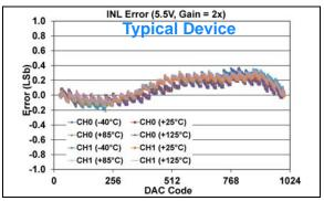
FIGURE 1-391: INL Error vs. DAC Code, and Temperature (Code 25 - 1000) (Dual Channel - MCP48FXB12) (10-bit:  $V_{DD} = 5.5V$ ,  $V_{REF} = 2.048V$ ,  $VRxB:VRxA = '11' (V_{REF} Buffered)$ , Gx = '1' (2x)).
