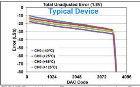
**FIGURE 1-114:** Total Unadjusted Error  $(V_{OUT})$  vs. DAC Code, and Temperature (Single Channel - **MCP48FXB21**) (12-bit:  $V_{DD} = 1.8V$ ,  $V_{REF} = 1V$ , VRxB:VRxA = '10' ( $V_{REF}$  Unbuffered), Gx = '1' (2x)), (see **Appendix B.3** for additional information).
