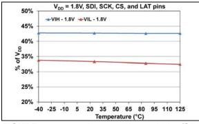
FIGURE 1-27: Average  $V_{IH}$  and  $V_{IL}$  (SDI, SCK,  $\overline{CS}$ , and  $\overline{LAT}$  pins) ( $V_{DD} = 1.8V$ ) vs. Temperature.
