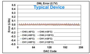
FIGURE 1-524: DNL Error vs. DAC Code, and Temperature (Code 6 - 250) (Dual Channel - MCP48FXB02) (8-bit:  $V_{DD} = 2.7V$ ,  $V_{REF} = V_{DD}$ ,  $VRxB:VRxA = '11' (V_{RFF} Buffered)$ , Gx = '0' (1x)).
