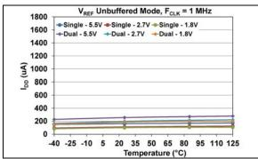
**FIGURE 1-18:** Average Device Supply Current - Active Interface ( $I_{DDA}$ ) ( $F_{SCK} = 1$  MHz) vs. Voltage and Temperature, VRxB:VRxA = '10' ( $V_{RFF}$  Unbuffered mode).
