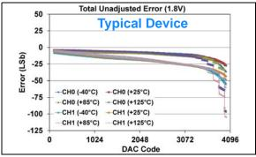
**FIGURE 1-81:** Total Unadjusted Error  $(V_{OUT})$  vs. DAC Code, and Temperature (Dual Channel - **MCP48FXB22**) (12-bit:  $V_{DD} = 1.8V$ ,  $V_{REF} = V_{DD}$ ,  $VRXB:VRXA = '10' (V_{REF} Unbuffered)$ , GX = '0' (1x)), (see **Appendix B.2** for additional information).
