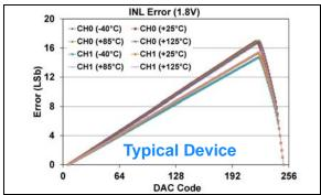
**FIGURE 1-483:** INL Error vs. DAC Code, and Temperature (Code 6 - 250) (Dual Channel - **MCP48FXB02**) (8-bit:  $V_{DD} = 1.8V$ ,  $V_{REF} = 1V$ ,  $V_{RXB}:V_{RXA} = '10'$  ( $V_{REF}$  Unbuffered),  $G_{X} = '1'(2x)$ ), (see **Appendix B.3** for additional information).
