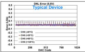
FIGURE 1-340: DNL Error vs. DAC Code, and Temperature (Code 25 - 1000) (Single Channel - MCP48FXB11) (10-bit:  $V_{DD} = 5.5V$ ,  $V_{REF} = V_{DD}$ ,  $VRxB:VRxA = '11' (V_{REF} Buffered)$ , Gx = '0' (1x)).
