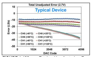
**FIGURE 1-188:** Total Unadjusted Error  $(V_{OUT})$  vs. DAC Code, and Temperature (Dual Channel - **MCP48FXB22**) (12-bit:  $V_{DD} = 2.7V$ ,  $V_{REF} = 1V$ , VRxB:VRxA = '11' ( $V_{REF}$  Buffered), Gx = '1' (2x)).
