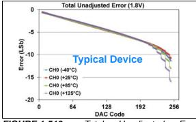
**FIGURE 1-510:** Total Unadjusted Error  $(V_{OUT})$  vs. DAC Code, and Temperature (Single Channel - **MCP48FXB01**) (8-bit:  $V_{DD} = 1.8V$ ,  $V_{REF} = V_{DD}$ ,  $VRxB:VRxA = '11' (V_{REF} Buffered)$ , Gx = '0' (1x)), (see **Appendix B.4** for additional information).
