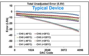
**FIGURE 1-115:** Total Unadjusted Error  $(V_{OUT})$  vs. DAC Code, and Temperature (Dual Channel - **MCP48FXB22**) (12-bit:  $V_{DD} = 5.5V$ ,  $V_{REF} = 1V$ , VRxB:VRxA = '10'  $(V_{RFF} \ Unbuffered)$ ,  $Gx = '1' \ (2x)$ ).
