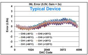
**FIGURE 1-67:** INL Error vs. DAC Code, and Temperature (Code 100 - 4000) (Dual Channel - **MCP48FXB22**) (12-bit:  $V_{DD} = 5.5V$ , VRxB:VRxA = '01' (Bandgap), Gx = '1' (2x)).
