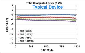
**FIGURE 1-365:** Total Unadjusted Error  $(V_{OUT})$  vs. DAC Code, and Temperature (Single Channel - **MCP48FXB11**)  $(10\text{-bit}: V_{DD} = 2.7V, V_{REF} = 1V, VRxB:VRxA = '11' <math>(V_{RFF} \text{ Buffered}), Gx = '1' (2x)).$
