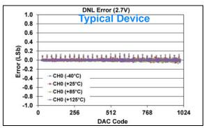
**FIGURE 1-233:** DNL Error vs. DAC Code, and Temperature (Code 25 - 1000) (Single Channel - **MCP48FXB11**) (10-bit:  $V_{DD} = 2.7V$ ,  $VRxB:VRxA = '00' (V_{DD})$ , Gx = '0' (1x)).
