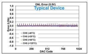
FIGURE 1-232: DNL Error vs. DAC Code, and Temperature (Code 25 - 1000) (Single Channel - MCP48FXB11) (10-bit:  $V_{DD} = 5.5V$ ,  $VRxB:VRxA = '00' (V_{DD})$ , Gx = '0' (1x)).
