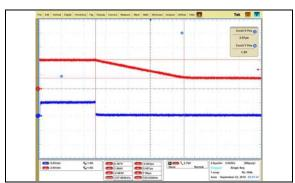
FIGURE 1-39: Half-Scale Settling Time – C00h to 400h (MCP48FXB2X).
