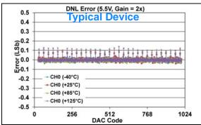
FIGURE 1-322: DNL Error vs. DAC Code, and Temperature (Code 25 - 1000) (Single Channel - MCP48FXB11) (10-bit:  $V_{DD} = 5.5V$ ,  $V_{REF} = 2.048V$ ,  $VRxB:VRxA = '10' (V_{REF} Unbuffered)$ , Gx = '1' (2x)).
