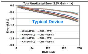
**FIGURE 1-494:** Total Unadjusted Error  $(V_{OUT})$  vs. DAC Code, and Temperature (Dual Channel - **MCP48FXB02**) (8-bit:  $V_{DD} = 5.5V$ ,  $V_{REF} = 2.048V$ ,  $VRxB:VRxA = '10' (V_{REF} Unbuffered)$ , Gx = '0' (1x)).
