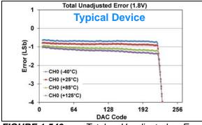
**FIGURE 1-546:** Total Unadjusted Error  $(V_{OUT})$  vs. DAC Code, and Temperature (Single Channel - **MCP48FXB01**) (8-bit:  $V_{DD} = 1.8V$ ,  $V_{REF} = 1V$ ,  $V_{RXB}$ :  $V_{RXA} = '11'$  ( $V_{REF}$  Buffered),  $G_{X} = '1'$  ( $V_{X} = V_{X} = V$
