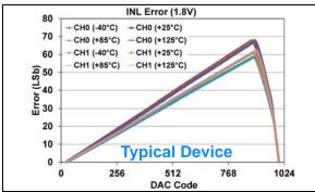
**FIGURE 1-303:** INL Error vs. DAC Code, and Temperature (Code 25 - 1000) (Dual Channel - **MCP48FXB12**) (10-bit:  $V_{DD} = 1.8V$ ,  $V_{REF} = 1V$ ,  $V_{RXB}$ :  $V_{RXA} = '10'$  ( $V_{REF}$  Unbuffered),  $V_{REF} = 1V$ ,  $V_{RXB}$ :  $V_{RXA} = V_{RXA} = V_{REF}$  (see **Appendix B.3** for additional information).
