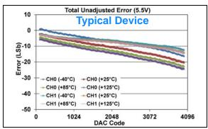
**FIGURE 1-97:** Total Unadjusted Error  $(V_{OUT})$  vs. DAC Code, and Temperature (Dual Channel - **MCP48FXB22**) (12-bit:  $V_{DD} = 5.5V$ ,  $V_{REF} = 1V$ , VRxB:VRxA = '10' ( $V_{REF}$  Unbuffered), Gx = '0' (1x).
