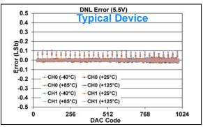
**FIGURE 1-343:** DNL Error vs. DAC Code, and Temperature (Code 25 - 1000) (Dual Channel - **MCP48FXB12**) (10-bit:  $V_{DD} = 5.5V$ ,  $V_{REF} = V_{DD}$ ,  $VRxB:VRxA = '11' (V_{REF} Buffered)$ , Gx = '0' (1x)).
