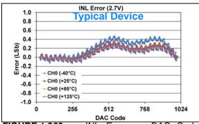
FIGURE 1-263: INL Error vs. DAC Code, and Temperature (Code 25 - 1000) (Single Channel - MCP48FXB11) (10-bit:  $V_{DD} = 2.7V$ ,  $V_{REF} = V_{DD}$ ,  $VRxB:VRxA = '10' (V_{REF} Unbuffered)$ , Gx = '0' (1x)).
