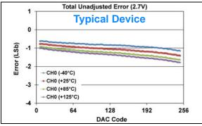
**FIGURE 1-473:** Total Unadjusted Error  $(V_{OUT})$  vs. DAC Code, and Temperature (Single Channel - **MCP48FXB01**) (8-bit:  $V_{DD} = 2.7V$ ,  $V_{REF} = 1V$ , VRxB:VRxA = '10' ( $V_{REF}$  Unbuffered), Gx = '1'(2x)).
