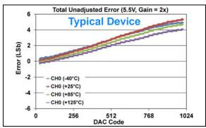
**FIGURE 1-238:** Total Unadjusted Error  $(V_{OUT})$  vs. DAC Code, and Temperature (Single Channel - **MCP48FXB11**)  $(10\text{-bit}: V_{DD} = 5.5V, VRxB:VRxA = '01' (Bandgap), Gx = '1' (2x)).$
