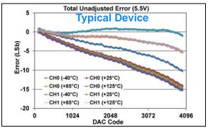
**FIGURE 1-43:** Total Unadjusted Error  $(V_{OUT})$  vs. DAC Code, and Temperature (Dual Channel - **MCP48FXB22**) (12-bit:  $V_{DD} = 5.5V$ ,  $VRxB:VRxA = '00' (V_{DD})$ , Gx = '0' (1x)).
