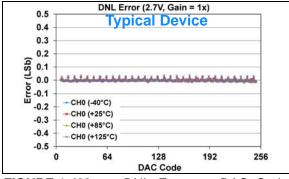
**FIGURE 1-432:** DNL Error vs. DAC Code, and Temperature (Code 6 - 250) (Single Channel - **MCP48FXB01**) (8-bit:  $V_{DD} = 2.7V$ , VRxB:VRxA = '01' (Bandgap), Gx = '0' (1x)).
