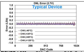
**FIGURE 1-269:** DNL Error vs. DAC Code, and Temperature (Code 25 - 1000) (Single Channel - **MCP48FXB11**) (10-bit:  $V_{DD} = 2.7V$ ,  $V_{REF} = V_{DD}$ ,  $VRxB:VRxA = '10' (V_{RFF} Unbuffered)$ , Gx = '0' (1x)).
