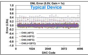
FIGURE 1-215: DNL Error vs. DAC Code, and Temperature (Code 100 - 4000) (Single Channel - MCP48FXB21) (12-bit:  $V_{DD} = 5.5V$ ,  $V_{REF} = 2.048V$ ,  $VRxB:VRxA = '11' (V_{REF} Buffered)$ , Gx = '0' (1x)).
