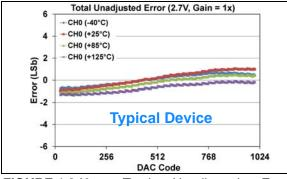
**FIGURE 1-240:** Total Unadjusted Error  $(V_{OUT})$  vs. DAC Code, and Temperature (Single Channel - **MCP48FXB11**)  $(10\text{-bit}: V_{DD} = 2.7V, VRxB:VRxA = '01' (Bandgap), Gx = '0' (1x)).$
