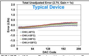
**FIGURE 1-420:** Total Unadjusted Error  $(V_{OUT})$  vs. DAC Code, and Temperature (Single Channel - **MCP48FXB01**) (8-bit:  $V_{DD} = 2.7V$ , VRxB:VRxA = '01' (Bandgap), Gx = '0' (1x)).
