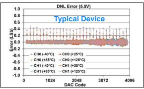
**FIGURE 1-55:** DNL Error vs. DAC Code, and Temperature (Code 100 - 4000) (Dual Channel - **MCP48FXB22**) (**12-bit**:  $V_{DD} = 5.5V$ ,  $VRxB:VRxA = '00' (V_{DD})$ , Gx = '0' (1x)).
