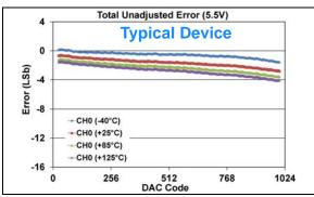
**FIGURE 1-292:** Total Unadjusted Error  $(V_{OUT})$  vs. DAC Code, and Temperature (Single Channel - **MCP48FXB11**)  $(10\text{-bit}: V_{DD} = 5.5 \text{V}, V_{REF} = 1 \text{V}, VRxB:VRxA = '10' (V_{REF} Unbuffered), Gx = '1' (2x)).$
