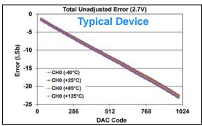
**FIGURE 1-329:** Total Unadjusted Error  $(V_{OUT})$  vs. DAC Code, and Temperature (Single Channel - **MCP48FXB11**)  $(10\text{-bit}: V_{DD} = 2.7\text{V}, V_{REF} = V_{DD}, VRxB:VRxA = '11' (V_{REF} \text{ Buffered}), Gx = '0' (1x)).$
