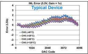
**FIGURE 1-65:** INL Error vs. DAC Code, and Temperature (Code 100 - 4000) (Single Channel - **MCP48FXB21**) (**12-bit**:  $V_{DD} = 5.5V$ , VRxB:VRxA = '01' (Bandgap), Gx = '0' (1x)).
