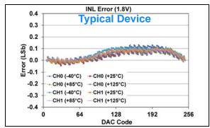
**FIGURE 1-465:** INL Error vs. DAC Code, and Temperature (Code 6 - 250) (Dual Channel - **MCP48FXB02**) (8-bit:  $V_{DD} = 1.8V$ ,  $V_{REF} = 1V$ ,  $V_{RXB}$ :  $V_{RXA} = '10'$  ( $V_{REF}$  Unbuffered),  $G_{X} = '0'$  (1x)).
