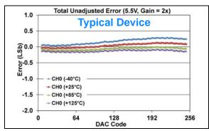
**FIGURE 1-562:** Total Unadjusted Error  $(V_{OUT})$  vs. DAC Code, and Temperature (Single Channel - **MCP48FXB01**) (8-bit:  $V_{DD} = 5.5V$ ,  $V_{REF} = 2.048V$ ,  $VRxB:VRxA = '11' (V_{REF} Buffered)$ , Gx = '1' (2x)).
