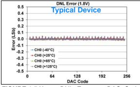
FIGURE 1-540: DNL Error vs. DAC Code, and Temperature (Code 6 - 250) (Single Channel - MCP48FXB01) (8-bit:  $V_{DD} = 1.8V$ ,  $V_{REF} = 1V$ ,  $V_{RXB}$ :  $V_{RXA} = '11'$  ( $V_{REF}$  Buffered),  $G_{X} = '0'$  (1x)).
