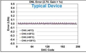
**FIGURE 1-576:** DNL Error vs. DAC Code, and Temperature (Code 6 - 250) (Single Channel - **MCP48FXB01**) (8-bit:  $V_{DD} = 2.7V$ ,  $V_{REF} = 2.048V$ ,  $VRxB:VRxA = '11' (V_{REF} Buffered)$ , Gx = '0' (1x)).
