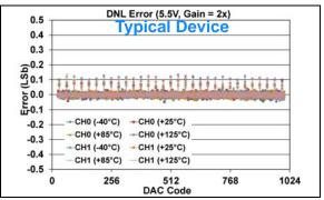
**FIGURE 1-397:** DNL Error vs. DAC Code, and Temperature (Code 25 - 1000) (Dual Channel - **MCP48FXB12**) (10-bit:  $V_{DD} = 5.5V$ ,  $V_{REF} = 2.048V$ ,  $VRxB:VRxA = '11' (V_{REF} Buffered)$ , Gx = '1' (2x)).
