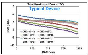
**FIGURE 1-350:** Total Unadjusted Error  $(V_{OUT})$  vs. DAC Code, and Temperature (Dual Channel - **MCP48FXB12**) (10-bit:  $V_{DD} = 2.7V$ ,  $V_{REF} = 1V$ , VRxB:VRxA = '11' ( $V_{REF}$  Buffered), Gx = '0' (1x)).
