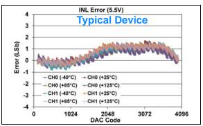
**FIGURE 1-175:** INL Error vs. DAC Code, and Temperature (Code 100 - 4000) (Dual Channel - **MCP48FXB22**) (**12-bit**:  $V_{DD} = 5.5V$ ,  $V_{REF} = 1V$ , VRxB:VRxA = '11' ( $V_{RFF}$  Buffered), Gx = '0' (1x)).
