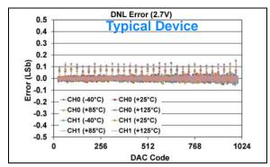
FIGURE 1-344: DNL Error vs. DAC Code, and Temperature (Code 25 - 1000) (Dual Channel - MCP48FXB12) (10-bit:  $V_{DD} = 2.7V$ ,  $V_{REF} = V_{DD}$ ,  $VRxB:VRxA = '11' (V_{RFF} Buffered)$ , Gx = '0' (1x)).
