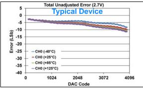
**FIGURE 1-77:** Total Unadjusted Error  $(V_{OUT})$  vs. DAC Code, and Temperature (Single Channel - **MCP48FXB21**) (**12-bit**:  $V_{DD} = 2.7V$ ,  $V_{REF} = V_{DD}$ , VRxB:VRxA = '10'  $(V_{REF}$  Unbuffered), Gx = '0' (1x)).
