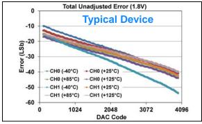
**FIGURE 1-99:** Total Unadjusted Error  $(V_{OUT})$  vs. DAC Code, and Temperature (Dual Channel - **MCP48FXB22**) (12-bit:  $V_{DD} = 1.8V$ ,  $V_{REF} = 1V$ , VRxB:VRxA = '10' ( $V_{REF}$  Unbuffered), Gx = '0' (1x)).
