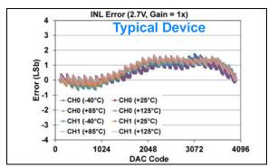
FIGURE 1-141: INL Error vs. DAC Code, and Temperature (Code 100 - 4000) (Dual Channel - MCP48FXB22) (12-bit:  $V_{DD} = 2.7V$ ,  $V_{REF} = 2.048V$ ,  $VRxB:VRxA = '10' (V_{REF} Unbuffered)$ , Gx = '0' (1x)).
