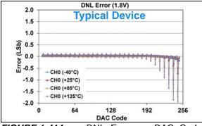
**FIGURE 1-414:** DNL Error vs. DAC Code, and Temperature (Code 6 - 250) (Single Channel - **MCP48FXB01**) (8-bit:  $V_{DD} = 1.8V$ ,  $V_{RXB}:V_{RXA} = '00' (V_{DD})$ ,  $G_{X} = '0' (1x)$ ), (see **Appendix B.1** for additional information).
