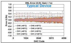
FIGURE 1-74: DNL Error vs. DAC Code, and Temperature (Code 100 - 4000) (Dual Channel - MCP48FXB22) (12-bit:  $V_{DD} = 5.5V$ , VRxB:VRxA = '01' (Bandgap), Gx = '0' (1x)).
