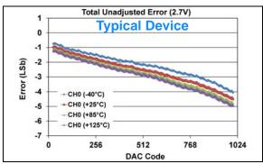
**FIGURE 1-221:** Total Unadjusted Error  $(V_{OUT})$  vs. DAC Code, and Temperature (Single Channel - **MCP48FXB11**)  $(10\text{-bit}: V_{DD} = 2.7V, VRxB: VRxA = '00' (V_{DD}), Gx = '0' (1x)).$
