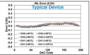
**FIGURE 1-517:** INL Error vs. DAC Code, and Temperature (Code 6 - 250) (Dual Channel - **MCP48FXB02**) (8-bit:  $V_{DD} = 5.5V$ ,  $V_{REF} = V_{DD}$ ,  $VRxB:VRxA = '11' (V_{REF} Buffered)$ , Gx = '0' (1x)).
