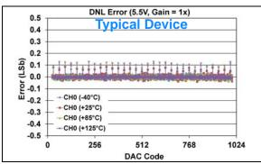
**FIGURE 1-395:** DNL Error vs. DAC Code, and Temperature (Code 25 - 1000) (Single Channel - **MCP48FXB11**) (10-bit:  $V_{DD} = 5.5V$ ,  $V_{REF} = 2.048V$ ,  $VRxB:VRxA = '11' (V_{REF} Buffered)$ , Gx = '0' (1x)).
