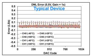
FIGURE 1-398: DNL Error vs. DAC Code, and Temperature (Code 25 - 1000) (Dual Channel - MCP48FXB12) (10-bit:  $V_{DD} = 5.5V$ ,  $V_{REF} = 2.048V$ ,  $VRxB:VRxA = '11' (V_{RFF} Buffered)$ , Gx = '0' (1x)).
