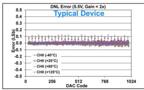
FIGURE 1-250: DNL Error vs. DAC Code, and Temperature (Code 25 - 1000) (Single Channel - MCP48FXB11) (10-bit:  $V_{DD} = 5.5V$ , VRxB:VRxA = '01' (Bandgap), Gx = '1' (2x)).
