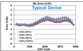
**FIGURE 1-82:** INL Error vs. DAC Code, and Temperature (Code 100 - 4000) (Single Channel - **MCP48FXB21**) (12-bit:  $V_{DD} = 5.5V$ ,  $V_{REF} = V_{DD}$ ,  $VRxB:VRxA = '10' (V_{RFF} Unbuffered)$ , Gx = '0' (1x)).
