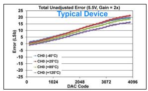
**FIGURE 1-58:** Total Unadjusted Error  $(V_{OUT})$  vs. DAC Code, and Temperature (Single Channel - **MCP48FXB21**) (12-bit:  $V_{DD} = 5.5V$ , VRxB:VRxA = '01' (Bandgap), Gx = '1' (2x)).
