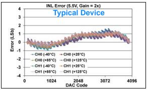
FIGURE 1-139: INL Error vs. DAC Code, and Temperature (Code 100 - 4000) (Dual Channel - MCP48FXB22) (12-bit:  $V_{DD} = 5.5V$ ,  $V_{REF} = 2.048V$ ,  $VRxB:VRxA = '10' (V_{REF} Unbuffered)$ , Gx = '1' (2x)).
