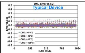
FIGURE 1-358: DNL Error vs. DAC Code, and Temperature (Code 25 - 1000) (Single Channel - **MCP48FXB11**) (10-bit:  $V_{DD} = 5.5V$ ,  $V_{REF} = 1V$ ,  $V_{RXB}:V_{RXA} = '11'$  ( $V_{RFF}$  Buffered),  $G_{X} = '0'$  (1x)).
