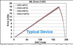
**FIGURE 1-552:** INL Error vs. DAC Code, and Temperature (Code 6 - 250) (Single Channel - **MCP48FXB01**) (8-bit:  $V_{DD} = 1.8V$ ,  $V_{REF} = 1V$ ,  $V_{RXB}:V_{RXA} = '11'$  ( $V_{REF}$  Buffered),  $G_{X} = '1'$  (2x)), (see **Appendix B.5** for additional information).
