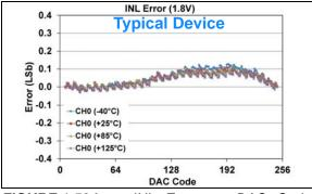
**FIGURE 1-534:** INL Error vs. DAC Code, and Temperature (Code 6 - 250) (Single Channel - **MCP48FXB01**) (8-bit:  $V_{DD} = 1.8V$ ,  $V_{REF} = 1V$ ,  $V_{RXB}:V_{RXA} = '11'$  ( $V_{REF}$  Buffered),  $G_{X} = '0'$  (1x)).
