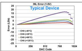
FIGURE 1-264: INL Error vs. DAC Code, and Temperature (Code 25 - 1000) (Single Channel - MCP48FXB11) (10-bit:  $V_{DD} = 1.8V$ ,  $V_{REF} = V_{DD}$ ,  $VRxB:VRxA = '10' (V_{REF} Unbuffered)$ , Gx = '0' (1x)),
