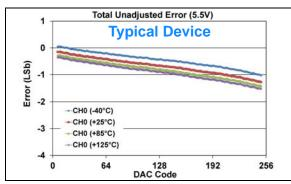
**FIGURE 1-454:** Total Unadjusted Error  $(V_{OUT})$  vs. DAC Code, and Temperature (Single Channel - **MCP48FXB01**) (8-bit:  $V_{DD} = 5.5V$ ,  $V_{REF} = 1V$ ,  $V_{RXB}:V_{RXA} = '10'$  ( $V_{RFF}$  Unbuffered),  $G_{X} = '0'$  (1x)).
