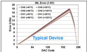
**FIGURE 1-555:** INL Error vs. DAC Code, and Temperature (Code 6 - 250) (Dual Channel - **MCP48FXB02**) (8-bit:  $V_{DD} = 1.8V$ ,  $V_{REF} = 1V$ ,  $V_{RXB}$ :  $V_{RXA} = '11'$  ( $V_{REF}$  Buffered),  $G_{X} = '1'$  ( $Z_{X}$ ), (see **Appendix B.5** for additional information).
