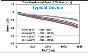
**FIGURE 1-134:** Total Unadjusted Error  $(V_{OUT})$  vs. DAC Code, and Temperature (Dual Channel - **MCP48FXB22**) (12-bit:  $V_{DD} = 5.5V$ ,  $V_{REF} = 2.048V$ ,  $VRxB:VRxA = '10' (V_{RFF} Unbuffered)$ , Gx = '0' (1x)).
