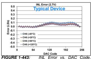
and Temperature (Code 6 - 250) (Single Channel - MCP48FXB01) (8-bit:  $V_{DD} = 2.7V$ ,  $V_{REF} = V_{DD}$ ,  $VRxB:VRxA = '10' (V_{RFF} Unbuffered)$ , Gx = '0' (1x)).
