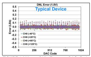
FIGURE 1-288: DNL Error vs. DAC Code, and Temperature (Code 25 - 1000) (Single Channel - MCP48FXB11) (10-bit:  $V_{DD} = 1.8V$ ,  $V_{REF} = 1V$ ,  $V_{RXB}$ : $V_{RXA} = '10'$  ( $V_{REF}$  Unbuffered),  $G_{X} = '0'$  (1x)).
