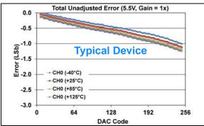
**FIGURE 1-491:** Total Unadjusted Error  $(V_{OUT})$  vs. DAC Code, and Temperature (Single Channel - **MCP48FXB01**) (8-bit:  $V_{DD} = 5.5V$ ,  $V_{REF} = 2.048V$ ,  $VRxB:VRxA = '10' (V_{REF} Unbuffered)$ , Gx = '0' (1x)).
