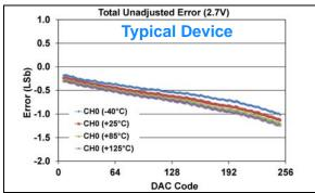
**FIGURE 1-401:** Total Unadjusted Error  $(V_{OUT})$  vs. DAC Code, and Temperature (Single Channel - **MCP48FXB01**)  $(8\text{-bit}: V_{DD} = 2.7V, VRxB: VRxA = '00' (V_{DD}), Gx = '0' (1x)).$
