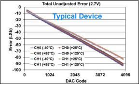
**FIGURE 1-152:** Total Unadjusted Error  $(V_{OUT})$  vs. DAC Code, and Temperature (Dual Channel - **MCP48FXB22**)  $(12\text{-bit}: V_{DD} = 2.7V, V_{REF} = V_{DD}, VRxB:VRxA = '11' (V_{REF} Buffered), Gx = '0' (1x)).$
