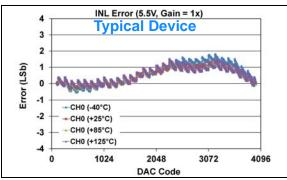
FIGURE 1-209: INL Error vs. DAC Code, and Temperature (Code 100 - 4000) (Single Channel - MCP48FXB21) (12-bit:  $V_{DD} = 5.5V$ ,  $V_{REF} = 2.048V$ ,  $VRxB:VRxA = '11' (V_{REF} Buffered)$ , Gx = '0' (1x)).
