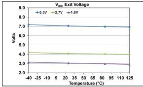
**FIGURE 1-33:** Average HVC pin High Voltage Exit Voltage ( $V_{IHHEXIT}$ ) vs.  $V_{DD}$  Voltage and Temperature.
