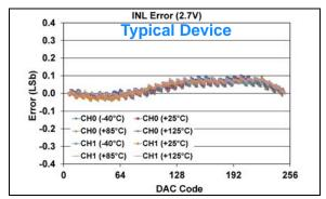
FIGURE 1-482: INL Error vs. DAC Code, and Temperature (Code 6 - 250) (Dual Channel - MCP48FXB02) (8-bit:  $V_{DD} = 2.7V$ ,  $V_{REF} = 1V$ , VRxB:VRxA = '10' ( $V_{RFF}$  Unbuffered), Gx = '1'(2x)).
