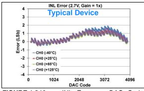
**FIGURE 1-210:** INL Error vs. DAC Code, and Temperature (Code 100 - 4000) (Single Channel - **MCP48FXB21**) (12-bit:  $V_{DD} = 2.7V$ ,  $V_{REF} = 2.048V$ ,  $VRxB:VRxA = '11' (V_{REF} Buffered)$ , Gx = '0' (1x)).
