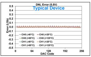
FIGURE 1-523: DNL Error vs. DAC Code, and Temperature (Code 6 - 250) (Dual Channel - MCP48FXB02) (8-bit:  $V_{DD} = 5.5V$ ,  $V_{REF} = V_{DD}$ ,  $VRxB:VRxA = '11' (V_{REF} Buffered)$ , Gx = '0' (1x)).
