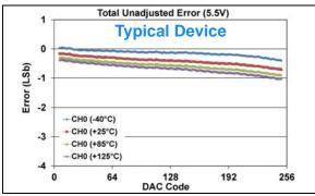
**FIGURE 1-472:** Total Unadjusted Error  $(V_{OUT})$  vs. DAC Code, and Temperature (Single Channel - **MCP48FXB01**) (8-bit:  $V_{DD} = 5.5V$ ,  $V_{REF} = 1V$ ,  $V_{RXB}:V_{RXA} = '10'$  ( $V_{REF}$  Unbuffered),  $G_{X} = '1'$  ( $Z_{X}$ ).
