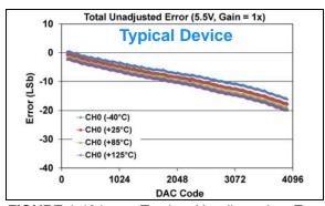
**FIGURE 1-131:** Total Unadjusted Error  $(V_{OUT})$  vs. DAC Code, and Temperature (Single Channel - **MCP48FXB21**) (12-bit:  $V_{DD} = 5.5V$ ,  $V_{REF} = 2.048V$ ,  $VRXB:VRXA = '10' (V_{REF} Unbuffered)$ , GX = '0' (1x)).
