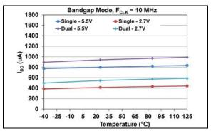
**FIGURE 1-13:** Average Device Supply Current - Active Interface ( $I_{DDA}$ ) ( $F_{SCK} = 10$  MHz) vs. Voltage and Temperature, VRxB:VRxA = '01' (Bandgap mode).
