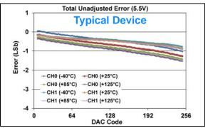
**FIGURE 1-457:** Total Unadjusted Error  $(V_{OUT})$  vs. DAC Code, and Temperature (Dual Channel - **MCP48FXB02**) (8-bit:  $V_{DD} = 5.5V$ ,  $V_{REF} = 1V$ ,  $V_{RXB}$ :  $V_{RXA} = '10'$  ( $V_{RFF}$  Unbuffered),  $G_{X} = '0'$  (1x)).
