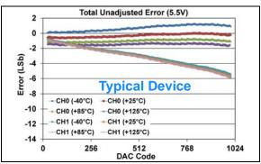
**FIGURE 1-367:** Total Unadjusted Error  $(V_{OUT})$  vs. DAC Code, and Temperature (Dual Channel - **MCP48FXB12**)  $(10\text{-bit}: V_{DD} = 5.5V, V_{REF} = 1V, VRxB:VRxA = '11' <math>(V_{RFF} \text{ Buffered}), Gx = '1' (2x)).$
