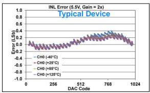
FIGURE 1-316: INL Error vs. DAC Code, and Temperature (Code 25 - 1000) (Single Channel - MCP48FXB11) (10-bit:  $V_{DD} = 5.5V$ ,  $V_{REF} = 2.048V$ ,  $VRxB:VRxA = '10' (V_{REF} Unbuffered)$ , Gx = '1' (2x)).
