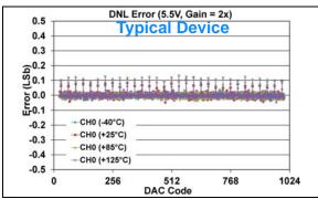
FIGURE 1-394: DNL Error vs. DAC Code, and Temperature (Code 25 - 1000) (Single Channel - MCP48FXB11) (10-bit:  $V_{DD} = 5.5V$ ,  $V_{REF} = 2.048V$ ,  $VRxB:VRxA = '11' (V_{REF} Buffered)$ , Gx = '1' (2x)).
