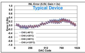
FIGURE 1-388: INL Error vs. DAC Code, and Temperature (Code 25 - 1000) (Single Channel - MCP48FXB11) (10-bit:  $V_{DD} = 5.5V$ ,  $V_{REF} = 2.048V$ ,  $VRxB:VRxA = '11' (V_{REF} Buffered)$ , Gx = '1' (2x)).
