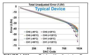
**FIGURE 1-333:** Total Unadjusted Error  $(V_{OUT})$  vs. DAC Code, and Temperature (Dual Channel - **MCP48FXB12**)  $(10\text{-bit}: V_{DD} = 1.8V, V_{REF} = V_{DD}, VRxB:VRxA = '11' (V_{REF} Buffered), Gx = '0' (1x)), (see$ **Appendix B.4**for additional information).
