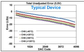
**FIGURE 1-94:** Total Unadjusted Error  $(V_{OUT})$  vs. DAC Code, and Temperature (Single Channel - **MCP48FXB21**) (12-bit:  $V_{DD} = 5.5V$ ,  $V_{REF} = 1V$ ,  $V_{RXB}$ : $V_{RXA} = '10'$  ( $V_{REF}$  Unbuffered),  $G_{X} = '0'$  ( $I_{X}$ ).
