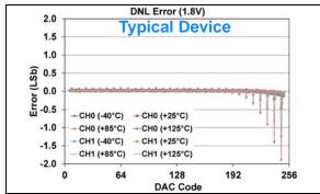
**FIGURE 1-525:** DNL Error vs. DAC Code, and Temperature (Code 6 - 250) (Dual Channel - **MCP48FXB02**) (8-bit:  $V_{DD} = 1.8V$ ,  $V_{REF} = V_{DD}$ , VRxB:VRxA = '11' ( $V_{REF}$  Buffered), Gx = '0' (1x)), (see **Appendix B.4** for additional information).
