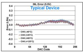
FIGURE 1-460: INL Error vs. DAC Code, and Temperature (Code 6 - 250) (Single Channel - MCP48FXB01) (8-bit:  $V_{DD} = 5.5V$ ,  $V_{REF} = 1V$ , VRxB:VRxA = '10' ( $V_{RFF}$  Unbuffered), Gx = '0' (1x)).
