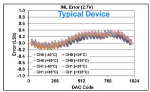
FIGURE 1-374: INL Error vs. DAC Code, and Temperature (Code 25 - 1000) (Dual Channel - MCP48FXB12) (10-bit:  $V_{DD} = 2.7V$ ,  $V_{REF} = 1V$ , VRxB:VRxA = '11' ( $V_{RFF}$  Buffered), Gx = '1' (2x).
