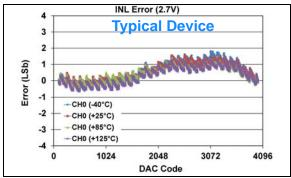
**FIGURE 1-173:** INL Error vs. DAC Code, and Temperature (Code 100 - 4000) (Single Channel - **MCP48FXB21**) (12-bit:  $V_{DD} = 2.7V$ ,  $V_{REF} = 1V$ , VRXB:VRXA = '11' ( $V_{REF}$  Buffered), GX = '0' (1x)).
