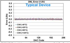
FIGURE 1-468: DNL Error vs. DAC Code, and Temperature (Code 6 - 250) (Single Channel - MCP48FXB01) (8-bit:  $V_{DD} = 1.8V$ ,  $V_{REF} = 1V$ ,  $V_{RXB}$ :  $V_{RXA} = '10'$  ( $V_{REF}$  Unbuffered),  $G_{X} = '0'$  (1x)).
