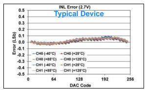
FIGURE 1-518: INL Error vs. DAC Code, and Temperature (Code 6 - 250) (Dual Channel - MCP48FXB02) (8-bit:  $V_{DD} = 2.7V$ ,  $V_{REF} = V_{DD}$ ,  $VRXB:VRXA = '11' (V_{REF} Buffered)$ , GX = '0' (1x)).
