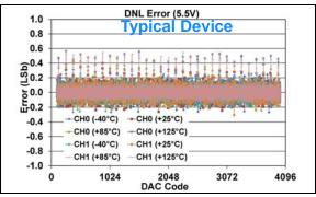
FIGURE 1-127: DNL Error vs. DAC Code, and Temperature (Code 100 - 4000) (Dual Channel - MCP48FXB22) (12-bit:  $V_{DD} = 5.5V$ ,  $V_{REF} = 1V$ , VRxB:VRxA = '10' ( $V_{REF}$  Unbuffered), Gx = '1' (2x)).
