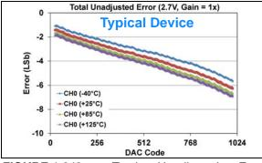
**FIGURE 1-312:** Total Unadjusted Error  $(V_{OUT})$  vs. DAC Code, and Temperature (Single Channel - **MCP48FXB11**)  $(10\text{-bit}: V_{DD} = 2.7V, V_{REF} = 2.048V, VRxB:VRxA = '10' (V_{REF} Unbuffered), Gx = '0' (1x)).$
