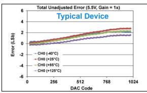
**FIGURE 1-239:** Total Unadjusted Error  $(V_{OUT})$  vs. DAC Code, and Temperature (Single Channel - **MCP48FXB11**)  $(10\text{-bit}: V_{DD} = 5.5V, VRxB:VRxA = '01' (Bandgap), <math>Gx = '0' (1x)$ ).
