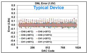
**FIGURE 1-363:** DNL Error vs. DAC Code, and Temperature (Code 25 - 1000) (Dual Channel - **MCP48FXB12**) (10-bit:  $V_{DD} = 1.8V$ ,  $V_{REF} = 1V$ , VRxB:VRxA = '11' ( $V_{REF}$  Buffered), Gx = '0' (1x)).
