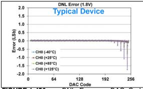
**FIGURE 1-450:** DNL Error vs. DAC Code, and Temperature (Code 6 - 250) (Single Channel - **MCP48FXB01**) (8-bit:  $V_{DD} = 1.8V$ ,  $V_{REF} = V_{DD}$ ,  $VRxB:VRxA = '10' (V_{REF} Unbuffered)$ , Gx = '0' (1x)),
