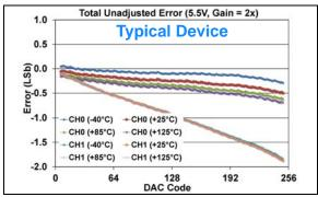
**FIGURE 1-493:** Total Unadjusted Error  $(V_{OUT})$  vs. DAC Code, and Temperature (Dual Channel - **MCP48FXB02**) (8-bit:  $V_{DD} = 5.5V$ ,  $V_{REF} = 2.048V$ ,  $VRxB:VRxA = '10' (V_{REF} Unbuffered)$ , Gx = '1' (2x)).
