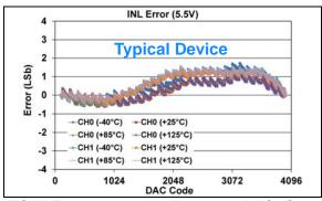
**FIGURE 1-49:** INL Error vs. DAC Code, and Temperature (Code 100 - 4000) (Dual Channel - **MCP48FXB22**) (12-bit:  $V_{DD} = 5.5V$ ,  $VRxB:VRxA = '00' (V_{DD})$ , Gx = '0' (1x)).
