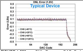
**FIGURE 1-558:** DNL Error vs. DAC Code, and Temperature (Code 6 - 250) (Single Channel - **MCP48FXB01**) (8-bit:  $V_{DD} = 1.8V$ ,  $V_{REF} = 1V$ ,  $V_{RXB}:V_{RXA} = '11'$  ( $V_{REF}$  Buffered),  $G_{X} = '1'$  (2x)), (see **Appendix B.5** for additional information).
