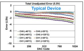
**FIGURE 1-349:** Total Unadjusted Error  $(V_{OUT})$  vs. DAC Code, and Temperature (Dual Channel - **MCP48FXB12**) (10-bit:  $V_{DD} = 5.5V$ ,  $V_{REF} = 1V$ , VRxB:VRxA = '11' ( $V_{RFF}$  Buffered), Gx = '0' (1x)).
