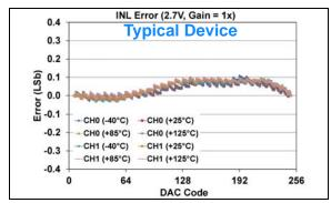
FIGURE 1-501: INL Error vs. DAC Code, and Temperature (Code 6 - 250) (Dual Channel - MCP48FXB02) (8-bit:  $V_{DD} = 2.7V$ ,  $V_{REF} = 2.048V$ ,  $VRxB:VRxA = '10' (V_{REF} Unbuffered)$ , Gx = '0' (1x)).
