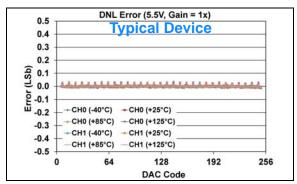
FIGURE 1-506: DNL Error vs. DAC Code, and Temperature (Code 6 - 250) (Dual Channel - MCP48FXB02) (8-bit:  $V_{DD} = 5.5V$ ,  $V_{REF} = 2.048V$ ,  $VRxB:VRxA = '10' (V_{RFF} Unbuffered)$ , Gx = '0' (1x)).
