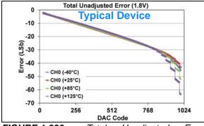
**FIGURE 1-330:** Total Unadjusted Error  $(V_{OUT})$  vs. DAC Code, and Temperature (Single Channel - **MCP48FXB11**)  $(10\text{-bit}: V_{DD} = 1.8V, V_{REF} = V_{DD}, VRXB:VRXA = '11' (V_{REF} Buffered), GX = '0' (1x)), (see$ **Appendix B.4**for additional information).
