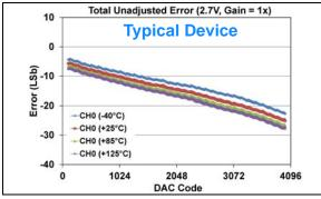
**FIGURE 1-132:** Total Unadjusted Error  $(V_{OUT})$  vs. DAC Code, and Temperature (Single Channel - **MCP48FXB21**) (12-bit:  $V_{DD} = 2.7V$ ,  $V_{REF} = 2.048V$ ,  $VRxB:VRxA = '10' (V_{REF} Unbuffered)$ , Gx = '0' (1x)).
