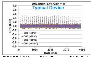
FIGURE 1-216: DNL Error vs. DAC Code, and Temperature (Code 100 - 4000) (Single Channel - MCP48FXB21) (12-bit:  $V_{DD} = 2.7V$ ,  $V_{REF} = 2.048V$ ,  $VRxB:VRxA = '11' (V_{REF} Buffered)$ , Gx = '0' (1x)).
