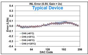
FIGURE 1-496: INL Error vs. DAC Code, and Temperature (Code 6 - 250) (Single Channel - MCP48FXB01) (8-bit:  $V_{DD} = 5.5V$ ,  $V_{REF} = 2.048V$ ,  $VRxB:VRxA = '10' (V_{REF} Unbuffered)$ , Gx = '1' (2x)).
