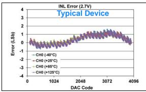
**FIGURE 1-191:** INL Error vs. DAC Code, and Temperature (Code 100 - 4000) (Single Channel - **MCP48FXB21**) (12-bit:  $V_{DD} = 2.7V$ ,  $V_{REF} = 1V$ ,  $V_{RXB}$ : $V_{RXA} = '11'$  ( $V_{RFF}$  Buffered),  $G_{X} = '1'$  ( $V_{X} = V_{X} = V_{X$
