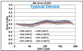
FIGURE 1-445: INL Error vs. DAC Code, and Temperature (Code 6 - 250) (Dual Channel - MCP48FXB02)
