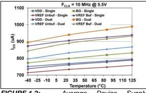
**FIGURE 1-2:** Average Device Supply Active Current  $(I_{DDA})$  (at 5.5V and  $F_{SCK} = 10 \text{ MHz})$  vs. Temperature and DAC Reference Voltage Mode.
