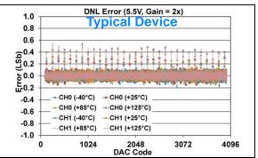
FIGURE 1-217: DNL Error vs. DAC Code, and Temperature (Code 100 - 4000) (Dual Channel - MCP48FXB22) (12-bit:  $V_{DD} = 5.5V$ ,  $V_{REF} = 2.048V$ ,  $VRxB:VRxA = '11' (V_{REF} Buffered)$ , Gx = '1' (2x)).
