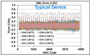
**FIGURE 1-183:** DNL Error vs. DAC Code, and Temperature (Code 100 - 4000) (Dual Channel - **MCP48FXB22**) (12-bit:  $V_{DD} = 1.8V$ ,  $V_{REF} = 1V$ , VRxB:VRxA = '11' ( $V_{REF}$  Buffered), Gx = '0' (1x)).
