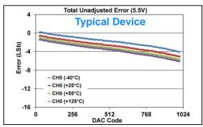
**FIGURE 1-274:** Total Unadjusted Error  $(V_{OUT})$  vs. DAC Code, and Temperature (Single Channel - **MCP48FXB11**) (10-bit:  $V_{DD} = 5.5V$ ,  $V_{REF} = 1V$ , VRxB:VRxA = '10' ( $V_{RFF}$  Unbuffered), Gx = '0' (1x).
