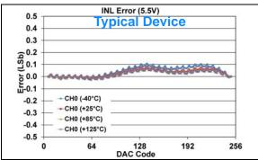
FIGURE 1-442: INL Error vs. DAC Code, and Temperature (Code 6 - 250) (Single Channel - MCP48FXB01)
