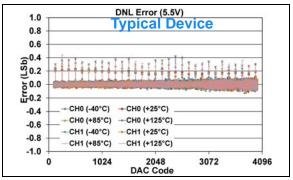
FIGURE 1-163: DNL Error vs. DAC Code, and Temperature (Code 100 - 4000) (Dual Channel - MCP48FXB22) (12-bit:  $V_{DD} = 5.5V$ ,  $V_{REF} = V_{DD}$ ,  $VRxB:VRxA = '11' (V_{REF} Buffered)$ , Gx = '0' (1x)).
