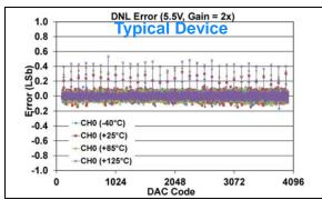
FIGURE 1-214: DNL Error vs. DAC Code, and Temperature (Code 100 - 4000) (Single Channel - MCP48FXB21) (12-bit:  $V_{DD} = 5.5V$ ,  $V_{REF} = 2.048V$ ,  $VRxB:VRxA = '11' (V_{REF} Buffered)$ , Gx = '1' (2x)).
