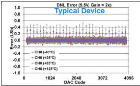
FIGURE 1-142: DNL Error vs. DAC Code, and Temperature (Code 100 - 4000) (Single Channel - MCP48FXB21) (12-bit:  $V_{DD} = 5.5V$ ,  $V_{REF} = 2.048V$ ,  $VRxB:VRxA = '10' (V_{REF} Unbuffered)$ , Gx = '1' (2x)).
