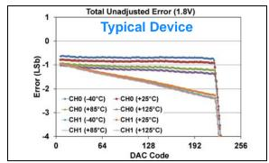
**FIGURE 1-549:** Total Unadjusted Error  $(V_{OUT})$  vs. DAC Code, and Temperature (Dual Channel - **MCP48FXB02**) (8-bit:  $V_{DD} = 1.8V$ ,  $V_{REF} = 1V$ , VRxB:VRxA = '11' ( $V_{REF}$  Buffered), Gx = '1'(2x)), (see **Appendix B.5** for additional information).
