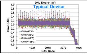
**FIGURE 1-198:** DNL Error vs. DAC Code, and Temperature (Code 100 - 4000) (Single Channel - **MCP48FXB21**) (12-bit:  $V_{DD} = 1.8V$ ,  $V_{REF} = 1V$ , VRxB:VRxA = '11' ( $V_{REF}$  Buffered), Gx = '1' (2x)), (see **Appendix B.5** for additional information).
