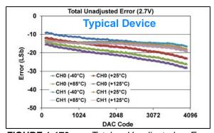
**FIGURE 1-170:** Total Unadjusted Error  $(V_{OUT})$  vs. DAC Code, and Temperature (Dual Channel - **MCP48FXB22**) (12-bit:  $V_{DD} = 2.7V$ ,  $V_{REF} = 1V$ , VRxB:VRxA = '11' ( $V_{REF}$  Buffered), Gx = '0' (1x)).
