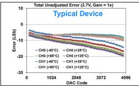
**FIGURE 1-207:** Total Unadjusted Error  $(V_{OUT})$  vs. DAC Code, and Temperature (Dual Channel - **MCP48FXB22**)  $(12\text{-bit}: V_{DD} = 2.7V, V_{REF} = 2.048V, VRxB:VRxA = '11' <math>(V_{REF}$  Buffered), Gx = '0' (1x)).
