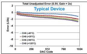
**FIGURE 1-310:** Total Unadjusted Error  $(V_{OUT})$  vs. DAC Code, and Temperature (Single Channel - **MCP48FXB11**)  $(10\text{-bit}: V_{DD} = 5.5\text{V}, V_{REF} = 2.048\text{V}, VRxB:VRxA = '10' (V_{REF} Unbuffered), Gx = '1' (2x)).$
