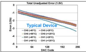
**FIGURE 1-459:** Total Unadjusted Error  $(V_{OUT})$  vs. DAC Code, and Temperature (Dual Channel - **MCP48FXB02**) (8-bit:  $V_{DD} = 1.8V$ ,  $V_{REF} = 1V$ , VRxB:VRxA = '10'  $(V_{REF}$  Unbuffered), Gx = '0' (1x)).
