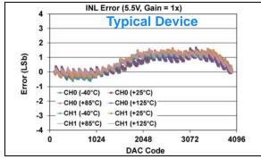
FIGURE 1-140: INL Error vs. DAC Code, and Temperature (Code 100 - 4000) (Dual Channel - MCP48FXB22) (12-bit:  $V_{DD} = 5.5V$ ,  $V_{REF} = 2.048V$ ,  $VRxB:VRxA = '10' (V_{REF} Unbuffered)$ , Gx = '0' (1x)).
