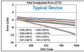
**FIGURE 1-296:** Total Unadjusted Error  $(V_{OUT})$  vs. DAC Code, and Temperature (Dual Channel - **MCP48FXB12**)  $(10\text{-bit: }V_{DD} = 2.7V, V_{REF} = 1V, VRxB:VRxA = '10' (V_{RFF} Unbuffered), Gx = '1' (2x)).$
