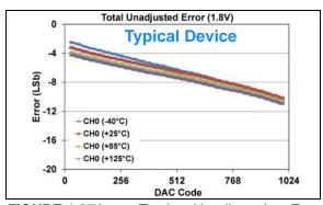
**FIGURE 1-276:** Total Unadjusted Error  $(V_{OUT})$  vs. DAC Code, and Temperature (Single Channel - **MCP48FXB11**)  $(10\text{-bit}: V_{DD} = 1.8V, V_{REF} = 1V, VRxB:VRxA = '10' <math>(V_{REF} \text{ Unbuffered}), Gx = '0' (1x)).$
