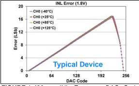
**FIGURE 1-480:** INL Error vs. DAC Code, and Temperature (Code 6 - 250) (Single Channel - **MCP48FXB01**) (8-bit:  $V_{DD} = 1.8V$ ,  $V_{REF} = 1V$ ,  $V_{RXB}:V_{RXA} = '10'$  ( $V_{REF}$  Unbuffered),  $G_{X} = '1'$  (2x)), (see **Appendix B.3** for additional information).
