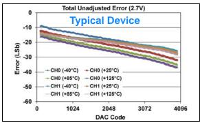
**FIGURE 1-98:** Total Unadjusted Error  $(V_{OUT})$  vs. DAC Code, and Temperature (Dual Channel - **MCP48FXB22**) (12-bit:  $V_{DD} = 2.7V$ ,  $V_{REF} = 1V$ , VRxB:VRxA = '10' ( $V_{RFF}$  Unbuffered), Gx = '0' (1x)).
