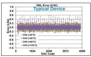
FIGURE 1-196: DNL Error vs. DAC Code, and Temperature (Code 100 - 4000) (Single Channel - MCP48FXB21) (12-bit:  $V_{DD} = 5.5V$ ,  $V_{REF} = 1V$ , VRxB:VRxA = '11' ( $V_{RFF}$  Buffered), Gx = '1' (2x).
