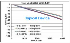
**FIGURE 1-151:** Total Unadjusted Error  $(V_{OUT})$  vs. DAC Code, and Temperature (Dual Channel - **MCP48FXB22**) (12-bit:  $V_{DD} = 5.5V$ ,  $V_{REF} = V_{DD}$ ,  $VRxB:VRxA = '11' (V_{REF} Buffered)$ , Gx = '0' (1x)).
