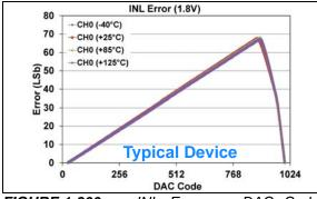
**FIGURE 1-300:** INL Error vs. DAC Code, and Temperature (Code 25 - 1000) (Single Channel - **MCP48FXB11**) (10-bit:  $V_{DD} = 1.8V$ ,  $V_{REF} = 1V$ , VRxB:VRxA = '10' ( $V_{REF}$  Unbuffered), Gx = '1' (2x)), (see **Appendix B.3** for additional information).
