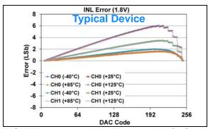
**FIGURE 1-519:** INL Error vs. DAC Code, and Temperature (Code 6 - 250) (Dual Channel - **MCP48FXB02**) (8-bit:  $V_{DD} = 1.8V$ ,  $V_{REF} = V_{DD}$ ,  $VRxB:VRxA = '11' (V_{REF} Buffered)$ , Gx = '0' (1x)), (see **Appendix B.4** for additional information).
