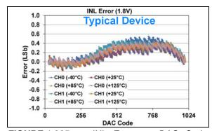
FIGURE 1-285: INL Error vs. DAC Code, and Temperature (Code 25 - 1000) (Dual Channel - MCP48FXB12) (10-bit:  $V_{DD} = 1.8V$ ,  $V_{REF} = 1V$ , VRxB:VRxA = '10' ( $V_{REF}$  Unbuffered), Gx = '0' (1x)).
