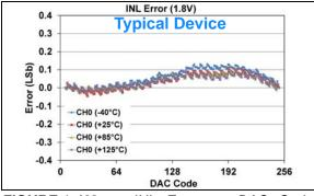
FIGURE 1-462: INL Error vs. DAC Code, and Temperature (Code 6 - 250) (Single Channel - MCP48FXB01) (8-bit:  $V_{DD} = 1.8V$ ,  $V_{REF} = 1V$ ,  $V_{RXB}:V_{RXA} = '10'$  ( $V_{REF}$  Unbuffered),  $G_{X} = '0'$  (1x)).
