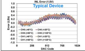
FIGURE 1-357: INL Error vs. DAC Code, and Temperature (Code 25 - 1000) (Dual Channel - MCP48FXB12) (10-bit:  $V_{DD} = 1.8V$ ,  $V_{REF} = 1V$ , VRxB:VRxA = '11' ( $V_{REF}$  Buffered), Gx = '0' (1x)).
