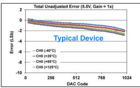
**FIGURE 1-383:** Total Unadjusted Error  $(V_{OUT})$  vs. DAC Code, and Temperature (Single Channel - **MCP48FXB11**)  $(10\text{-bit}: V_{DD} = 5.5V, V_{REF} = 2.048V, VRxB:VRxA = '11' <math>(V_{REF} \text{ Buffered}), Gx = '0' (1x)).$
