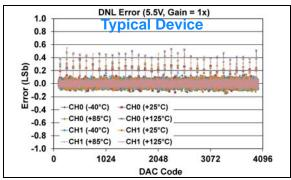
FIGURE 1-218: DNL Error vs. DAC Code, and Temperature (Code 100 - 4000) (Dual Channel - MCP48FXB22) (12-bit:  $V_{DD} = 5.5V$ ,  $V_{REF} = 2.048V$ ,  $VRxB:VRxA = '11' (V_{RFF} Buffered)$ , Gx = '0' (1x)).
