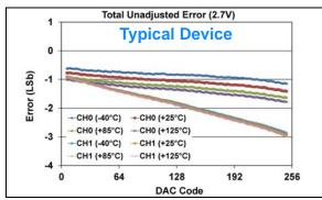
**FIGURE 1-476:** Total Unadjusted Error  $(V_{OUT})$  vs. DAC Code, and Temperature (Dual Channel - **MCP48FXB02**) (8-bit:  $V_{DD} = 2.7V$ ,  $V_{REF} = 1V$ , VRxB:VRxA = '10'  $(V_{REF}$  Unbuffered), Gx = '1' (2x)).
