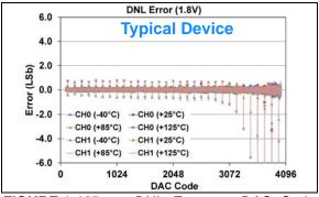
**FIGURE 1-165:** DNL Error vs. DAC Code, and Temperature (Code 100 - 4000) (Dual Channel - **MCP48FXB22**) (12-bit:  $V_{DD} = 1.8V$ ,  $V_{REF} = V_{DD}$ ,  $VRxB:VRxA = '11' (V_{REF} Buffered)$ , Gx = '0' (1x)), (see **Appendix B.4** for additional information).
