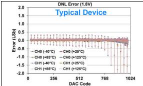
FIGURE 1-237: DNL Error vs. DAC Code, and Temperature (Code 25 - 1000) (Dual Channel - MCP48FXB12) (10-bit:  $V_{DD} = 1.8V$ ,  $VRxB:VRxA = '00' (V_{DD})$ , Gx = '0' (1x)), (see Appendix B.1 for additional information).
