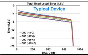
**FIGURE 1-294:** Total Unadjusted Error  $(V_{OUT})$  vs. DAC Code, and Temperature (Single Channel - **MCP48FXB11**)  $(10\text{-bit}: V_{DD} = 1.8V, V_{REF} = 1V, VRxB:VRxA = '10' (V_{REF} Unbuffered), Gx = '1' (2x)),$  (see **Appendix B.3** for additional information).
