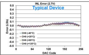
**FIGURE 1-515:** INL Error vs. DAC Code, and Temperature (Code 6 - 250) (Single Channel - **MCP48FXB01**) (8-bit:  $V_{DD} = 2.7V$ ,  $V_{REF} = V_{DD}$ ,  $VRxB:VRxA = '11' (V_{REF} Buffered)$ , Gx = '0' (1x)).
