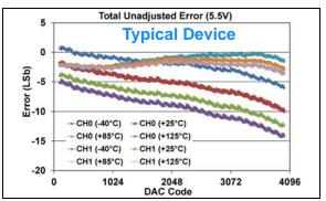
**FIGURE 1-169:** Total Unadjusted Error  $(V_{OUT})$  vs. DAC Code, and Temperature (Dual Channel - **MCP48FXB22**) (12-bit:  $V_{DD} = 5.5V$ ,  $V_{REF} = 1V$ , VRxB:VRxA = '11' ( $V_{REF}$  Buffered), Gx = '0' (1x)).
