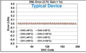
FIGURE 1-579: DNL Error vs. DAC Code, and Temperature (Code 6 - 250) (Dual Channel - MCP48FXB02) (8-bit:  $V_{DD} = 2.7V$ ,  $V_{REF} = 2.048V$ ,  $VRxB:VRxA = '11' (V_{REF} Buffered)$ , Gx = '0' (1x)).
