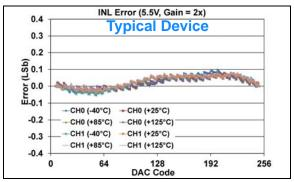
FIGURE 1-499: INL Error vs. DAC Code, and Temperature (Code 6 - 250) (Dual Channel - MCP48FXB02) (8-bit:  $V_{DD} = 5.5V$ ,  $V_{REF} = 2.048V$ ,  $VRxB:VRxA = '10' (V_{REF} Unbuffered)$ , Gx = '1' (2x)).
