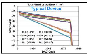
**FIGURE 1-117:** Total Unadjusted Error  $(V_{OUT})$  vs. DAC Code, and Temperature (Dual Channel - **MCP48FXB22**)  $(12\text{-bit}: V_{DD} = 1.8V, V_{REF} = 1V, VRxB:VRxA = '10' (V_{REF} Unbuffered), <math>Gx = '1' (2x)$ ), (see **Appendix B.3** for additional information).
