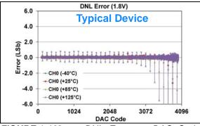
FIGURE 1-162: DNL Error vs. DAC Code, and Temperature (Code 100 - 4000) (Single Channel - MCP48FXB21) (12-bit:  $V_{DD} = 1.8V$ ,  $V_{REF} = V_{DD}$ ,  $VRxB:VRxA = '11' (V_{REF} Buffered)$ , Gx = '0' (1x), (see Appendix B.4 for additional information).
