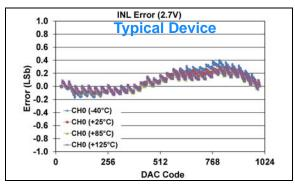
**FIGURE 1-335:** INL Error vs. DAC Code, and Temperature (Code 25 - 1000) (Single Channel - **MCP48FXB11**) (10-bit:  $V_{DD} = 2.7V$ ,  $V_{REF} = V_{DD}$ ,  $VRxB:VRxA = '11' (V_{REF} Buffered)$ , Gx = '0' (1x)).
