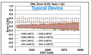
FIGURE 1-73: DNL Error vs. DAC Code, and Temperature (Code 100 - 4000) (Dual Channel - MCP48FXB22) (12-bit:  $V_{DD} = 5.5V$ , VRxB:VRxA = '01' (Bandgap), Gx = '1' (2x)).
