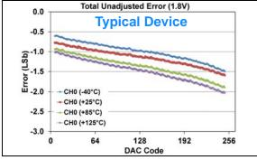
**FIGURE 1-528:** Total Unadjusted Error  $(V_{OUT})$  vs. DAC Code, and Temperature (Single Channel - **MCP48FXB01**) (8-bit:  $V_{DD} = 1.8V$ ,  $V_{REF} = 1V$ , VRxB:VRxA = '11'  $(V_{RFF} Buffered)$ , Gx = '0' (1x)).
