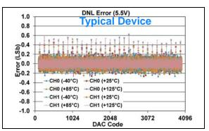
**FIGURE 1-109:** DNL Error vs. DAC Code, and Temperature (Code 100 - 4000) (Dual Channel - **MCP48FXB22**) (12-bit:  $V_{DD} = 5.5V$ ,  $V_{REF} = 1V$ , VRxB:VRxA = '10' ( $V_{REF}$  Unbuffered), Gx = '0' (1x)).
