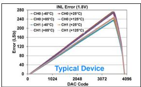
**FIGURE 1-123:** INL Error vs. DAC Code, and Temperature (Code 100 - 4000) (Dual Channel - **MCP48FXB22**) (**12-bit**:  $V_{DD} = 1.8V$ ,  $V_{REF} = 1V$ , VRxB:VRxA = '10' ( $V_{REF}$  Unbuffered), Gx = '1' (2x)), (see **Appendix B.3** for additional information).
