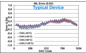
FIGURE 1-334: INL Error vs. DAC Code, and Temperature (Code 25 - 1000) (Single Channel - MCP48FXB11) (10-bit:  $V_{DD} = 5.5V$ ,  $V_{REF} = V_{DD}$ ,  $VRxB:VRxA = '11' (V_{REF} Buffered)$ , Gx = '0' (1x)).
