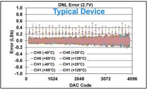
FIGURE 1-164: DNL Error vs. DAC Code, and Temperature (Code 100 - 4000) (Dual Channel - MCP48FXB22) (12-bit:  $V_{DD} = 2.7V$ ,  $V_{REF} = V_{DD}$ ,  $VRxB:VRxA = '11' (V_{RFF} Buffered)$ , Gx = '0' (1x)).
