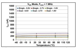
**FIGURE 1-9:** Average Device Supply Current - Active Interface ( $I_{DDA}$ ) ( $F_{SCK} = 1$  MHz) vs. Voltage and Temperature, VRxB:VRxA = '00' ( $V_{DD}$  mode).
