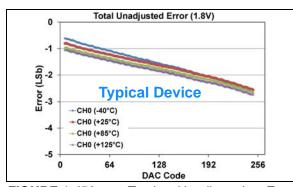
**FIGURE 1-456:** Total Unadjusted Error  $(V_{OUT})$  vs. DAC Code, and Temperature (Single Channel - **MCP48FXB01**) (8-bit:  $V_{DD} = 1.8V$ ,  $V_{REF} = 1V$ ,  $V_{RXB}$ : $V_{RXA} = '10'$  ( $V_{REF}$  Unbuffered),  $G_{X} = '0'$  (1x)).
