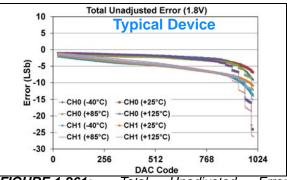
**FIGURE 1-261:** Total Unadjusted Error  $(V_{OUT})$  vs. DAC Code, and Temperature (Dual Channel - **MCP48FXB12**)  $(10\text{-bit}: V_{DD} = 1.8V, V_{REF} = V_{DD}, VRxB:VRxA = '10' (V_{REF} Unbuffered), Gx = '0' (1x)), (see$ **Appendix B.2**for additional information).
