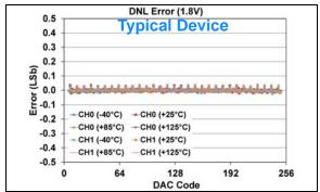
FIGURE 1-471: DNL Error vs. DAC Code, and Temperature (Code 6 - 250) (Dual Channel - MCP48FXB02) (8-bit:  $V_{DD} = 1.8V$ ,  $V_{REF} = 1V$ , VRxB:VRxA = '10' ( $V_{RFF}$  Unbuffered), Gx = '0' (1x)).
