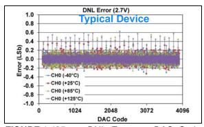
**FIGURE 1-125:** DNL Error vs. DAC Code, and Temperature (Code 100 - 4000) (Single Channel - **MCP48FXB21**) (12-bit:  $V_{DD} = 2.7V$ ,  $V_{REF} = 1V$ ,  $V_{RXB}:V_{RXA} = '10'$  ( $V_{REF}$  Unbuffered),  $G_{X} = '1'$  (2x)).
