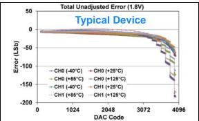
**FIGURE 1-45:** Total Unadjusted Error  $(V_{OUT})$  vs. DAC Code, and Temperature (Dual Channel - **MCP48FXB22**) (12-bit:  $V_{DD} = 1.8V$ ,  $VRxB:VRxA = '00' (V_{DD})$ , Gx = '0' (1x)), (see **Appendix B.1** for additional information).
