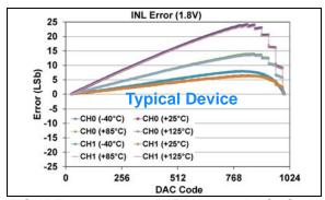
**FIGURE 1-339:** INL Error vs. DAC Code, and Temperature (Code 25 - 1000) (Dual Channel - **MCP48FXB12**) (10-bit:  $V_{DD} = 1.8V$ ,  $V_{REF} = V_{DD}$ ,  $VRxB:VRxA = '11' (V_{REF} Buffered)$ , Gx = '0' (1x)), (see **Appendix B.4** for additional information).
