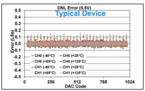
FIGURE 1-307: DNL Error vs. DAC Code, and Temperature (Code 25 - 1000) (Dual Channel - MCP48FXB12) (10-bit:  $V_{DD} = 5.5V$ ,  $V_{REF} = 1V$ , VRxB:VRxA = '10' ( $V_{REF}$  Unbuffered), Gx = '1' (2x).
