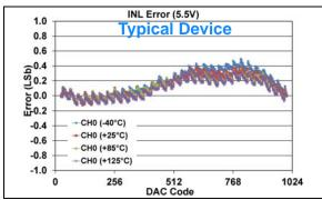
**FIGURE 1-280:** INL Error vs. DAC Code, and Temperature (Code 25 - 1000) (Single Channel - **MCP48FXB11**) (10-bit:  $V_{DD} = 5.5V$ ,  $V_{REF} = 1V$ , VRxB:VRxA = '10' ( $V_{RFF}$  Unbuffered), Gx = '0' (1x)).
