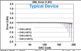
**FIGURE 1-522:** DNL Error vs. DAC Code, and Temperature (Code 6 - 250) (Single Channel - **MCP48FXB01**) (8-bit:  $V_{DD} = 1.8V$ ,  $V_{REF} = V_{DD}$ , VRxB:VRxA = '11' ( $V_{REF}$  Buffered), Gx = '0' (1x)), (see **Appendix B.4** for additional information).
