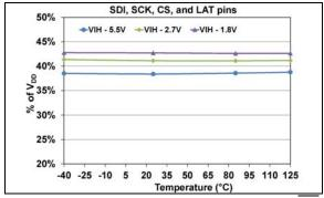
**FIGURE 1-28:** Average  $V_{IH}$  (SDI, SCK,  $\overline{CS}$ , and  $\overline{LAT}$  pins) vs. Voltage and Temperature.
