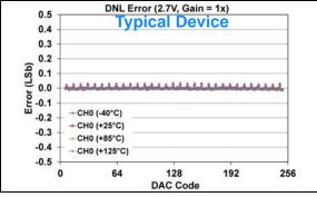
FIGURE 1-504: DNL Error vs. DAC Code, and Temperature (Code 6 - 250) (Single Channel - MCP48FXB01) (8-bit:  $V_{DD} = 2.7V$ ,  $V_{REF} = 2.048V$ ,  $VRxB:VRxA = '10' (V_{REF} Unbuffered)$ , Gx = '0' (1x)).
