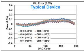
**FIGURE 1-553:** INL Error vs. DAC Code, and Temperature (Code 6 - 250) (Dual Channel - **MCP48FXB02**) (8-bit:  $V_{DD} = 5.5V$ ,  $V_{REF} = 1V$ ,  $V_{RXB}:V_{RXA} = '11'$  ( $V_{REF}$  Buffered),  $G_{X} = '1'$  ( $Z_{X}$ ).
