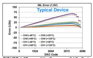
**FIGURE 1-87:** INL Error vs. DAC Code, and Temperature (Code 100 - 4000) (Dual Channel - **MCP48FXB22**) (**12-bit**:  $V_{DD} = 1.8V$ ,  $V_{REF} = V_{DD}$ , VRxB:VRxA = '10' ( $V_{REF}$  Unbuffered), Gx = '0' (1x)), (see **Appendix B.2** for additional information).
