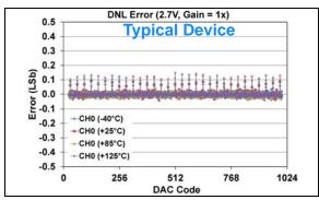
FIGURE 1-324: DNL Error vs. DAC Code, and Temperature (Code 25 - 1000) (Single Channel - MCP48FXB11) (10-bit:  $V_{DD} = 2.7V$ ,  $V_{REF} = 2.048V$ ,  $VRxB:VRxA = '10' (V_{REF} Unbuffered)$ , Gx = '0' (1x)).
