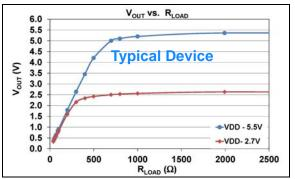
**FIGURE 1-37:**  $V_{OUT}$  vs.  $R_{LOAD}$  and Voltage (at +25°C) ( $R_{LOAD}$  0 $\Omega$  - 2500 $\Omega$ ).
