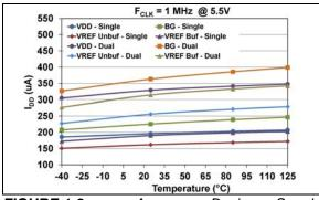
**FIGURE 1-3:** Average Device Supply Active Current  $(I_{DDA})$  (at 5.5V and  $F_{SCK} = 1$  MHz) vs. Temperature and DAC Reference Voltage Mode.
