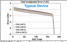
**FIGURE 1-474:** Total Unadjusted Error  $(V_{OUT})$  vs. DAC Code, and Temperature (Single Channel - **MCP48FXB01**) (8-bit:  $V_{DD} = 1.8V$ ,  $V_{REF} = 1V$ ,  $V_{RXB}:V_{RXA} = '10'$  ( $V_{REF}$  Unbuffered),  $G_{X} = '1'$  (2x)), (see **Appendix B.3** for additional information).
