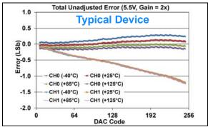
**FIGURE 1-565:** Total Unadjusted Error  $(V_{OUT})$  vs. DAC Code, and Temperature (Dual Channel - **MCP48FXB02**) (8-bit:  $V_{DD} = 5.5V$ ,  $V_{REF} = 2.048V$ ,  $VRxB:VRxA = '11' (V_{REF} Buffered)$ , Gx = '1' (2x)).
