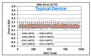
FIGURE 1-290: DNL Error vs. DAC Code, and Temperature (Code 25 - 1000) (Dual Channel - MCP48FXB12) (10-bit:  $V_{DD} = 2.7V$ ,  $V_{REF} = 1V$ , VRxB:VRxA = '10' ( $V_{RFF}$  Unbuffered), Gx = '0' (1x)).
