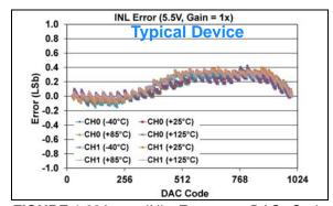
FIGURE 1-320: INL Error vs. DAC Code, and Temperature (Code 25 - 1000) (Dual Channel - MCP48FXB12) (10-bit:  $V_{DD} = 5.5V$ ,  $V_{REF} = 2.048V$ ,  $VRxB:VRxA = '10' (V_{RFF} Unbuffered)$ , Gx = '0' (1x)).
