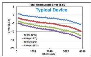
**FIGURE 1-166:** Total Unadjusted Error  $(V_{OUT})$  vs. DAC Code, and Temperature (Single Channel - **MCP48FXB21**) (12-bit:  $V_{DD} = 5.5V$ ,  $V_{REF} = 1V$ , VRxB:VRxA = '11' ( $V_{REF}$  Buffered), Gx = '0' (1x)).
