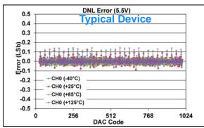
**FIGURE 1-286:** DNL Error vs. DAC Code, and Temperature (Code 25 - 1000) (Single Channel - **MCP48FXB11**) (10-bit:  $V_{DD} = 5.5V$ ,  $V_{REF} = 1V$ ,  $V_{RXB}:V_{RXA} = '10'$  ( $V_{RFF}$  Unbuffered),  $G_{X} = '0'$  (1x)).
