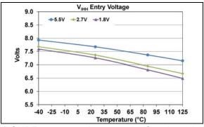
**FIGURE 1-32:** Average HVC pin High Voltage Entry Voltage  $(V_{IHHENTRY})$  vs.  $V_{DD}$  Voltage and Temperature.
