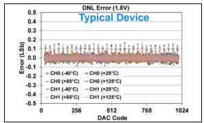
**FIGURE 1-291:** DNL Error vs. DAC Code, and Temperature (Code 25 - 1000) (Dual Channel - **MCP48FXB12**) (10-bit:  $V_{DD} = 1.8V$ ,  $V_{REF} = 1V$ , VRxB:VRxA = '10' ( $V_{REF}$  Unbuffered), Gx = '0' (1x)).
