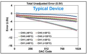
**FIGURE 1-295:** Total Unadjusted Error  $(V_{OUT})$  vs. DAC Code, and Temperature (Dual Channel - **MCP48FXB12**)  $(10\text{-bit}: V_{DD} = 5.5V, V_{REF} = 1V, VRxB:VRxA = '10' (V_{RFF} Unbuffered), <math>Gx = '1' (2x)$ ).
