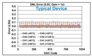
FIGURE 1-326: DNL Error vs. DAC Code, and Temperature (Code 25 - 1000) (Dual Channel - MCP48FXB12) (10-bit:  $V_{DD} = 5.5V$ ,  $V_{REF} = 2.048V$ ,  $VRxB:VRxA = '10' (V_{RFF} Unbuffered)$ , Gx = '0' (1x)).
