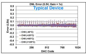
FIGURE 1-251: DNL Error vs. DAC Code, and Temperature (Code 25 - 1000) (Single Channel - MCP48FXB11) (10-bit:  $V_{DD} = 5.5V$ , VRxB:VRxA = '01' (Bandgap), Gx = '0' (1x)).
