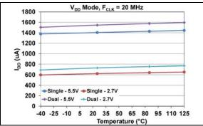
**FIGURE 1-7:** Average Device Supply Current - Active Interface ( $I_{DDA}$ ) ( $F_{SCK} = 20$  MHz) vs. Voltage and Temperature, VRxB:VRxA = `00" ( $V_{DD}$  mode).
