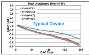
**FIGURE 1-400:** Total Unadjusted Error  $(V_{OUT})$  vs. DAC Code, and Temperature (Single Channel - **MCP48FXB01**)  $(8\text{-bit}: V_{DD} = 5.5V, VRxB: VRxA = '00' (V_{DD}), Gx = '0' (1x)).$
