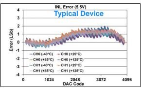
**FIGURE 1-103:** INL Error vs. DAC Code, and Temperature (Code 100 - 4000) (Dual Channel - **MCP48FXB22**) (**12-bit**:  $V_{DD} = 5.5V$ ,  $V_{REF} = 1V$ , VRxB:VRxA = '10' ( $V_{REF}$  Unbuffered), Gx = '0' (1x)).
