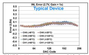
**FIGURE 1-429:** INL Error vs. DAC Code, and Temperature (Code 6 - 250) (Dual Channel - **MCP48FXB02**) (8-bit:  $V_{DD} = 2.7V$ , VRxB:VRxA = '01' (Bandgap), Gx = '0' (1x)).
