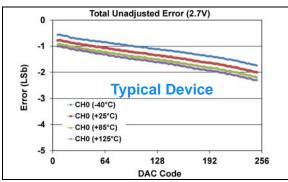
**FIGURE 1-455:** Total Unadjusted Error  $(V_{OUT})$  vs. DAC Code, and Temperature (Single Channel - **MCP48FXB01**) (8-bit:  $V_{DD} = 2.7V$ ,  $V_{REF} = 1V$ ,  $V_{RXB}:V_{RXA} = '10'$  ( $V_{REF}$  Unbuffered),  $G_{X} = '0' (1x)$ ).
