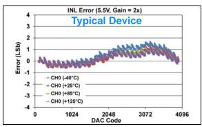
FIGURE 1-64: INL Error vs. DAC Code, and Temperature (Code 100 - 4000) (Single Channel - MCP48FXB21) (12-bit:  $V_{DD} = 5.5V$ , VRxB:VRxA = '01' (Bandgap), Gx = '1' (2x)).
