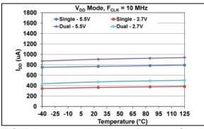
**FIGURE 1-8:** Average Device Supply Current - Active Interface ( $I_{DDA}$ ) ( $F_{SCK} = 10$  MHz) vs. Voltage and Temperature,  $VRxB:VRxA = `00" (V_{DD} mode)$ .
