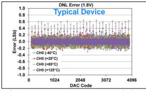
**FIGURE 1-180:** DNL Error vs. DAC Code, and Temperature (Code 100 - 4000) (Single Channel - **MCP48FXB21**) (12-bit:  $V_{DD} = 1.8V$ ,  $V_{REF} = 1V$ ,  $V_{RXB}:V_{RXA} = '11'$  ( $V_{REF}$  Buffered),  $G_{X} = '0'$  (1x)).
