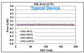
**FIGURE 1-485:** DNL Error vs. DAC Code, and Temperature (Code 6 - 250) (Single Channel - **MCP48FXB01**) (8-bit:  $V_{DD} = 2.7V$ ,  $V_{REF} = 1V$ ,  $V_{RXB}:V_{RXA} = '10'$  ( $V_{REF}$  Unbuffered),  $G_{X} = '1'$  ( $Z_{X}$ ).
