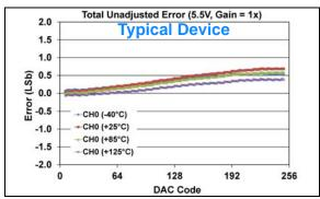
**FIGURE 1-419:** Total Unadjusted Error  $(V_{OUT})$  vs. DAC Code, and Temperature (Single Channel - **MCP48FXB01**) (8-bit:  $V_{DD} = 5.5V$ , VRxB:VRxA = '01' (Bandgap), Gx = '0' (1x)).
