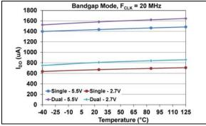
**FIGURE 1-12:** Average Device Supply Current - Active Interface ( $I_{DDA}$ ) ( $F_{SCK} = 20$  MHz) vs. Voltage and Temperature,  $VRxB:VRxA = {}^{\circ}01$ ' (Bandgap mode).
