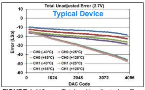
**FIGURE 1-116:** Total Unadjusted Error  $(V_{OUT})$  vs. DAC Code, and Temperature (Dual Channel - **MCP48FXB22**) (12-bit:  $V_{DD} = 2.7V$ ,  $V_{REF} = 1V$ , VRxB:VRxA = '10' ( $V_{REF}$  Unbuffered), Gx = '1' (2x).
