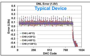
**FIGURE 1-306:** DNL Error vs. DAC Code, and Temperature (Code 25 - 1000) (Single Channel - **MCP48FXB11**) (10-bit:  $V_{DD} = 1.8V$ ,  $V_{REF} = 1V$ , VRxB:VRxA = '10' ( $V_{REF}$  Unbuffered), Gx = '1' (2x)), (see **Appendix B.3** for additional information).
