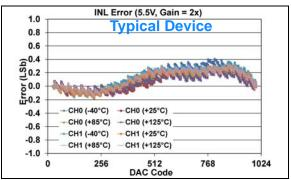
**FIGURE 1-247:** INL Error vs. DAC Code, and Temperature (Code 25 - 1000) (Dual Channel - **MCP48FXB12**) (10-bit:  $V_{DD} = 5.5V$ , VRxB:VRxA = '01' (Bandgap), Gx = '1' (2x)).
