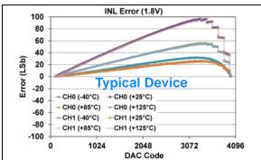
**FIGURE 1-159:** INL Error vs. DAC Code, and Temperature (Code 100 - 4000) (Dual Channel - **MCP48FXB22**) (12-bit:  $V_{DD} = 1.8V$ ,  $V_{REF} = V_{DD}$ , VRXB:VRXA = '11' ( $V_{REF}$  Buffered), GX = '0' (1x)), (see **Appendix B.4** for additional information).
