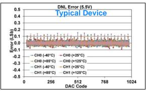
**FIGURE 1-379:** DNL Error vs. DAC Code, and Temperature (Code 25 - 1000) (Dual Channel - **MCP48FXB12**) (10-bit:  $V_{DD} = 5.5V$ ,  $V_{REF} = 1V$ , VRxB:VRxA = '11' ( $V_{RFF}$  Buffered), Gx = '1' (2x)).
