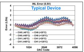
**FIGURE 1-85:** INL Error vs. DAC Code, and Temperature (Code 100 - 4000) (Dual Channel - **MCP48FXB22**) (12-bit:  $V_{DD} = 5.5V$ ,  $V_{REF} = V_{DD}$ ,  $VRxB:VRxA = '10' (V_{RFF} Unbuffered)$ , Gx = '0' (1x)).
