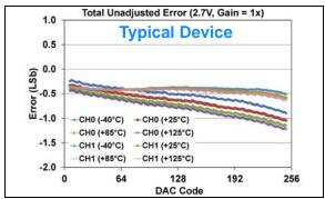
**FIGURE 1-567:** Total Unadjusted Error  $(V_{OUT})$  vs. DAC Code, and Temperature (Dual Channel - **MCP48FXB02**) (8-bit:  $V_{DD} = 2.7V$ ,  $V_{REF} = 2.048V$ ,  $VRxB:VRxA = '11' (V_{REF} Buffered)$ , Gx = '0' (1x)).
