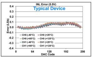
**FIGURE 1-535:** INL Error vs. DAC Code, and Temperature (Code 6 - 250) (Dual Channel - **MCP48FXB02**) (8-bit:  $V_{DD} = 5.5V$ ,  $V_{REF} = 1V$ , VRxB:VRxA = '11' ( $V_{RFF}$  Buffered), Gx = '0' (1x)).
