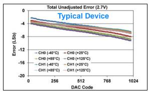
**FIGURE 1-278:** Total Unadjusted Error  $(V_{OUT})$  vs. DAC Code, and Temperature (Dual Channel - **MCP48FXB12**) (10-bit:  $V_{DD} = 2.7V$ ,  $V_{REF} = 1V$ , VRxB:VRxA = '10' ( $V_{RFF}$  Unbuffered), Gx = '0' (1x)).
