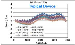
**FIGURE 1-86:** INL Error vs. DAC Code, and Temperature (Code 100 - 4000) (Dual Channel - **MCP48FXB22**) (12-bit:  $V_{DD} = 2.7V$ ,  $V_{REF} = V_{DD}$ , VRxB:VRxA = '10' ( $V_{RFF}$  Unbuffered), Gx = '0' (1x)).
