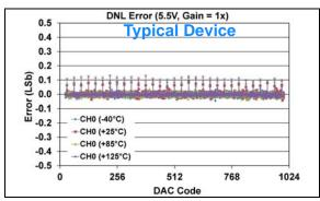
FIGURE 1-323: DNL Error vs. DAC Code, and Temperature (Code 25 - 1000) (Single Channel - MCP48FXB11) (10-bit:  $V_{DD} = 5.5V$ ,  $V_{REF} = 2.048V$ ,  $VRxB:VRxA = '10' (V_{REF} Unbuffered)$ , Gx = '0' (1x)).
