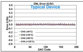
**FIGURE 1-556:** DNL Error vs. DAC Code, and Temperature (Code 6 - 250) (Single Channel - **MCP48FXB01**) (8-bit:  $V_{DD} = 5.5V$ ,  $V_{REF} = 1V$ ,  $V_{RXB}:V_{RXA} = '11'$  ( $V_{REF}$  Buffered),  $G_{X} = '1'$  ( $Z_{X}$ ).
