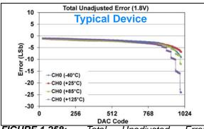
**FIGURE 1-258:** Total Unadjusted Error  $(V_{OUT})$  vs. DAC Code, and Temperature (Single Channel - **MCP48FXB11**)  $(10\text{-bit}: V_{DD} = 1.8V, V_{REF} = V_{DD}, VRXB:VRXA = '10' (V_{REF} Unbuffered), Gx = '0' (1x)), (see$ **Appendix B.2**for additional information).
