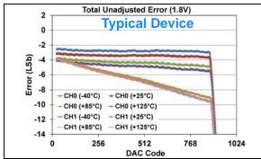
**FIGURE 1-369:** Total Unadjusted Error  $(V_{OUT})$  vs. DAC Code, and Temperature (Dual Channel - **MCP48FXB12**) (10-bit:  $V_{DD} = 1.8V$ ,  $V_{REF} = 1V$ , VRxB:VRxA = '11' ( $V_{REF}$  Buffered), Gx = '1' (2x), (see **Appendix B.5** for additional information).
