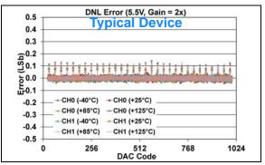
**FIGURE 1-325:** DNL Error vs. DAC Code, and Temperature (Code 25 - 1000) (Dual Channel - **MCP48FXB12**) (10-bit:  $V_{DD} = 5.5V$ ,  $V_{REF} = 2.048V$ ,
