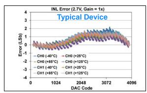
FIGURE 1-69: INL Error vs. DAC Code, and Temperature (Code 100 - 4000) (Dual Channel - MCP48FXB22) (12-bit:  $V_{DD} = 2.7V$ , VRxB:VRxA = '01' (Bandgap), Gx = '0' (1x)).
