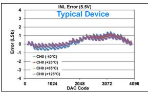
FIGURE 1-154: INL Error vs. DAC Code, and Temperature (Code 100 - 4000) (Single Channel - MCP48FXB21) (12-bit:  $V_{DD} = 5.5V$ ,  $V_{REF} = V_{DD}$ ,  $VRxB:VRxA = '11' (V_{REF} Buffered)$ , Gx = '0' (1x)).
