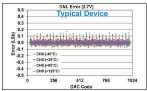
**FIGURE 1-305:** DNL Error vs. DAC Code, and Temperature (Code 25 - 1000) (Single Channel - **MCP48FXB11**) (10-bit:  $V_{DD} = 2.7V$ ,  $V_{REF} = 1V$ ,  $V_{RXB}$ : $V_{RXA} = '10'$  ( $V_{RFF}$  Unbuffered),  $G_{X} = '1'$  (2x)).
