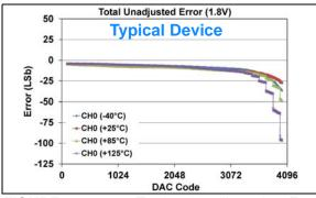
**FIGURE 1-78:** Total Unadjusted Error  $(V_{OUT})$  vs. DAC Code, and Temperature (Single Channel - **MCP48FXB21**) (**12-bit**:  $V_{DD} = 1.8V$ ,  $V_{REF} = V_{DD}$ , VRXB:VRXA = '10' ( $V_{REF}$  Unbuffered), GX = '0' (1x)), (see **Appendix B.2** for additional information).
