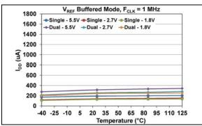
**FIGURE 1-22:** Average Device Supply Current - Active Interface ( $I_{DDA}$ ) ( $F_{SCK} = 1$  MHz) vs. Voltage and Temperature, VRxB:VRxA = '11' ( $V_{RFF}$  Buffered mode).
