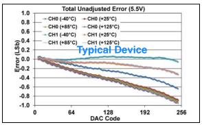
**FIGURE 1-403:** Total Unadjusted Error  $(V_{OUT})$  vs. DAC Code, and Temperature (Dual Channel - **MCP48FXB02**) (8-bit:  $V_{DD} = 5.5V$ ,  $VRxB:VRxA = '00' (V_{DD})$ , Gx = '0' (1x)).
