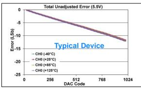
**FIGURE 1-328:** Total Unadjusted Error  $(V_{OUT})$  vs. DAC Code, and Temperature (Single Channel - **MCP48FXB11**)  $(10\text{-bit}: V_{DD} = 5.5\text{V}, V_{REF} = V_{DD}, VRxB:VRxA = '11' (V_{REF} \text{ Buffered}), Gx = '0' (1x)).$
