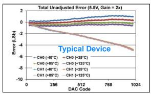
**FIGURE 1-385:** Total Unadjusted Error  $(V_{OUT})$  vs. DAC Code, and Temperature (Dual Channel - **MCP48FXB12**) (10-bit:  $V_{DD} = 5.5V$ ,  $V_{REF} = 2.048V$ ,  $VRxB:VRxA = '11' (V_{RFF} Buffered)$ , Gx = '1' (2x)).
