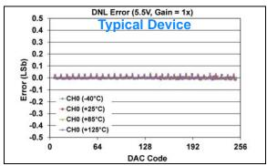
**FIGURE 1-431:** DNL Error vs. DAC Code, and Temperature (Code 6 - 250) (Single Channel - **MCP48FXB01**) (8-bit:  $V_{DD} = 5.5V$ , VRxB:VRxA = '01' (Bandgap), Gx = '0' (1x)).
