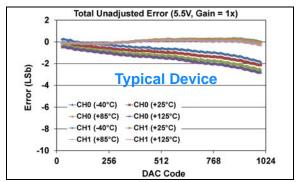
**FIGURE 1-386:** Total Unadjusted Error  $(V_{OUT})$  vs. DAC Code, and Temperature (Dual Channel - **MCP48FXB12**)  $(10\text{-bit}: V_{DD} = 5.5V, V_{REF} = 2.048V, VRxB:VRxA = '11' (V_{REF} Buffered), Gx = '0' (1x)).$
