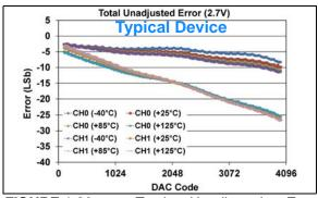
**FIGURE 1-80:** Total Unadjusted Error  $(V_{OUT})$  vs. DAC Code, and Temperature (Dual Channel - **MCP48FXB22**) (12-bit:  $V_{DD} = 2.7V$ ,  $V_{REF} = V_{DD}$ ,  $VRxB:VRxA = '10' (V_{REF} Unbuffered)$ , Gx = '0' (1x)).
