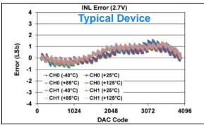
**FIGURE 1-158:** INL Error vs. DAC Code, and Temperature (Code 100 - 4000) (Dual Channel - **MCP48FXB22**) (12-bit:  $V_{DD} = 2.7V$ ,  $V_{REF} = V_{DD}$ ,  $VRxB:VRxA = '11' (V_{REF} Buffered)$ , Gx = '0' (1x)).
