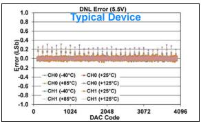
FIGURE 1-91: DNL Error vs. DAC Code, and Temperature (Code 100 - 4000) (Dual Channel - MCP48FXB22) (12-bit:  $V_{DD} = 5.5V$ ,  $V_{REF} = V_{DD}$ ,  $VRxB:VRxA = '10' (V_{RFF} Unbuffered)$ , Gx = '0' (1x)).
