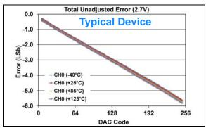
**FIGURE 1-509:** Total Unadjusted Error  $(V_{OUT})$  vs. DAC Code, and Temperature (Single Channel - **MCP48FXB01**) (8-bit:  $V_{DD} = 2.7V$ ,  $V_{REF} = V_{DD}$ ,  $VRxB:VRxA = '11' (V_{REF} Buffered)$ , Gx = '0' (1x)).
