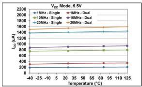
**FIGURE 1-11:** Average Device Supply Current vs.  $F_{SCK}$  Frequency, Voltage and Temperature, VRxB:VRxA = '00' (V<sub>DD</sub> mode).
