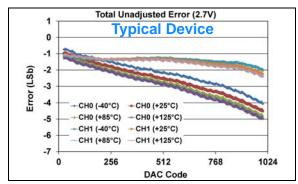
**FIGURE 1-224:** Total Unadjusted Error  $(V_{OUT})$  vs. DAC Code, and Temperature (Dual Channel - **MCP48FXB12**)  $(10\text{-bit}: V_{DD} = 2.7V, VRxB: VRxA = '00' (V_{DD}), Gx = '0' (1x)).$
