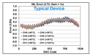
FIGURE 1-393: INL Error vs. DAC Code, and Temperature (Code 25 - 1000) (Dual Channel - MCP48FXB12) (10-bit:  $V_{DD} = 2.7V$ ,  $V_{REF} = 2.048V$ ,  $VRxB:VRxA = '11' (V_{REF} Buffered)$ , Gx = '0' (1x)).
