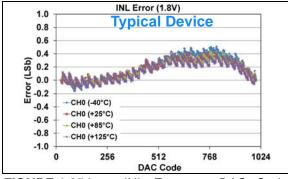
**FIGURE 1-354:** INL Error vs. DAC Code, and Temperature (Code 25 - 1000) (Single Channel - **MCP48FXB11**) (10-bit:  $V_{DD} = 1.8V$ ,  $V_{REF} = 1V$ , VRxB:VRxA = '11' ( $V_{REF}$  Buffered), Gx = '0' (1x)).
