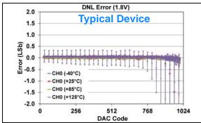
**FIGURE 1-234:** DNL Error vs. DAC Code, and Temperature (Code 25 - 1000) (Single Channel - **MCP48FXB11**) (10-bit:  $V_{DD} = 1.8V$ ,  $VRxB:VRxA = '00' (V_{DD})$ , Gx = '0' (1x)), (see **Appendix B.1** for additional information).
