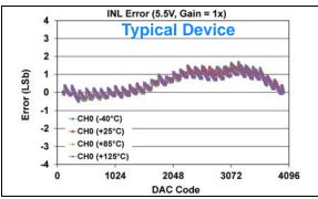
**FIGURE 1-137:** INL Error vs. DAC Code, and Temperature (Code 100 - 4000) (Single Channel - **MCP48FXB21**) (12-bit:  $V_{DD} = 5.5V$ ,  $V_{REF} = 2.048V$ ,  $VRxB:VRxA = '10' (V_{REF} Unbuffered)$ , Gx = '0' (1x)).
