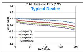
**FIGURE 1-526:** Total Unadjusted Error  $(V_{OUT})$  vs. DAC Code, and Temperature (Single Channel - **MCP48FXB01**) (8-bit:  $V_{DD} = 5.5V$ ,  $V_{REF} = 1V$ , VRxB:VRxA = '11' ( $V_{RFF}$  Buffered), Gx = '0' (1x)).
