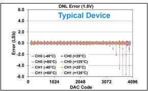
FIGURE 1-93: DNL Error vs. DAC Code, and Temperature (Code 100 - 4000) (Dual Channel - MCP48FXB22) (12-bit:  $V_{DD} = 1.8V$ ,  $V_{REF} = V_{DD}$ , VRxB:VRxA = '10' ( $V_{REF}$  Unbuffered), Gx = '0' (1x)), (see Appendix B.2 for additional information).
