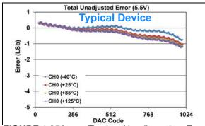
**FIGURE 1-256:** Total Unadjusted Error (V<sub>OUT</sub>) vs. DAC Code, and Temperature (Single Channel - **MCP48FXB11**)
