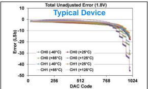
**FIGURE 1-225:** Total Unadjusted Error  $(V_{OUT})$  vs. DAC Code, and Temperature (Dual Channel - **MCP48FXB12**)  $(10\text{-bit}: V_{DD} = 1.8V, VRxB: VRxA = '00' (V_{DD}), Gx = '0' (1x)),$  (see **Appendix B.1** for additional information).
