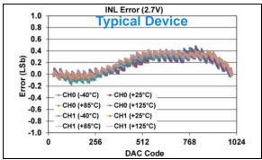
FIGURE 1-230: INL Error vs. DAC Code, and Temperature (Code 25 - 1000) (Dual Channel - MCP48FXB12) (10-bit:  $V_{DD} = 2.7V$ ,  $VRxB:VRxA = '00' (V_{DD})$ , Gx = '0' (1x)).
