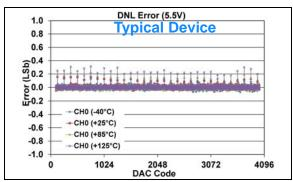
FIGURE 1-88: DNL Error vs. DAC Code, and Temperature (Code 100 - 4000)
