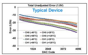
**FIGURE 1-171:** Total Unadjusted Error  $(V_{OUT})$  vs. DAC Code, and Temperature (Dual Channel - **MCP48FXB22**) (12-bit:  $V_{DD} = 1.8V$ ,  $V_{REF} = 1V$ , VRxB:VRxA = '11' ( $V_{REF}$  Buffered), Gx = '0' (1x)).
