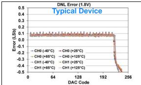
FIGURE 1-489: DNL Error vs. DAC Code, and Temperature (Code 6 - 250) (Dual Channel - MCP48FXB02) (8-bit:  $V_{DD} = 1.8V$ ,  $V_{REF} = 1V$ ,  $V_{RXB}$ :  $V_{RXA} = '10'$  ( $V_{REF}$  Unbuffered),  $G_{X} = '1'$  (2x)), (see Appendix B.3 for additional information).
