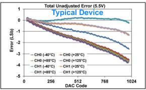
**FIGURE 1-223:** Total Unadjusted Error  $(V_{OUT})$  vs. DAC Code, and Temperature (Dual Channel - **MCP48FXB12**)  $(10\text{-bit}: V_{DD} = 5.5V, VRxB: VRxA = '00' (V_{DD}), Gx = '0' (1x)).$
