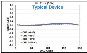
FIGURE 1-406: INL Error vs. DAC Code, and Temperature (Code 6 - 250) (Single Channel - MCP48FXB01) (8-bit:  $V_{DD} = 5.5V$ ,  $V_{RXB}:V_{RXA} = '00' (V_{DD})$ ,  $G_{X} = '0' (1x)$ ).
