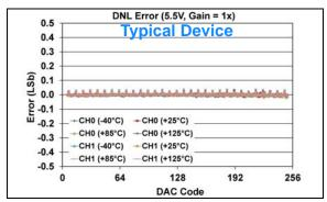
FIGURE 1-434: DNL Error vs. DAC Code, and Temperature (Code 6 - 250) (Dual Channel - MCP48FXB02) (8-bit:  $V_{DD} = 5.5V$ , VRxB:VRxA = '01' (Bandgap), Gx = '0' (1x)).
