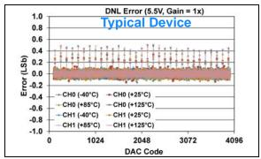
FIGURE 1-146: DNL Error vs. DAC Code, and Temperature (Code 100 - 4000) (Dual Channel - MCP48FXB22) (12-bit:  $V_{DD} = 5.5V$ ,  $V_{REF} = 2.048V$ ,  $VRxB:VRxA = '10' (V_{RFF} Unbuffered)$ , Gx = '0' (1x)).
