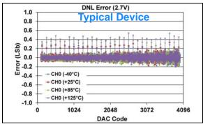
FIGURE 1-161: DNL Error vs. DAC Code, and Temperature (Code 100 - 4000) (Single Channel - MCP48FXB21) (12-bit:  $V_{DD} = 2.7V$ ,  $V_{REF} = V_{DD}$ ,  $VRxB:VRxA = '11' (V_{REF} Buffered)$ , Gx = '0' (1x)).
