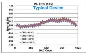
FIGURE 1-352: INL Error vs. DAC Code, and Temperature (Code 25 - 1000) (Single Channel - MCP48FXB11) (10-bit:  $V_{DD} = 5.5V$ ,  $V_{REF} = 1V$ , VRxB:VRxA = '11' ( $V_{RFF}$  Buffered), Gx = '0' (1x)).
