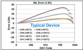
**FIGURE 1-231:** INL Error vs. DAC Code, and Temperature (Code 25 - 1000) (Dual Channel - **MCP48FXB12**) (10-bit:  $V_{DD} = 1.8V$ ,  $VRxB:VRxA = '00' (V_{DD})$ , Gx = '0' (1x)), (see **Appendix B.1** for additional information).
