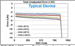
**FIGURE 1-366:** Total Unadjusted Error  $(V_{OUT})$  vs. DAC Code, and Temperature (Single Channel - **MCP48FXB11**)  $(10\text{-bit}: V_{DD} = 1.8V, V_{REF} = 1V, VRxB:VRxA = '11' <math>(V_{REF} \text{ Buffered}), Gx = '1' (2x)),$  (see **Appendix B.5** for additional information).
