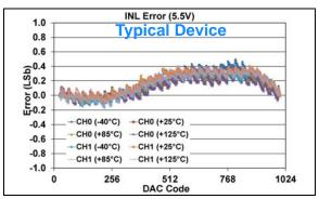
**FIGURE 1-283:** INL Error vs. DAC Code, and Temperature (Code 25 - 1000) (Dual Channel - **MCP48FXB12**) (10-bit:  $V_{DD} = 5.5V$ ,  $V_{REF} = 1V$ , VRxB:VRxA = '10' ( $V_{RFF}$  Unbuffered), Gx = '0' (1x)).
