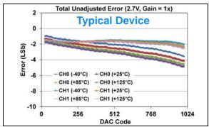
**FIGURE 1-387:** Total Unadjusted Error  $(V_{OUT})$  vs. DAC Code, and Temperature (Dual Channel - **MCP48FXB12**)  $(10\text{-bit}: V_{DD} = 2.7V, V_{REF} = 2.048V, VRxB:VRxA = '11' (V_{REF} Buffered), Gx = '0' (1x)).$
