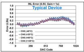
**FIGURE 1-389:** INL Error vs. DAC Code, and Temperature (Code 25 - 1000) (Single Channel - **MCP48FXB11**) (10-bit:  $V_{DD} = 5.5V$ ,  $V_{REF} = 2.048V$ ,  $VRxB:VRxA = '11' (V_{REF} Buffered)$ , Gx = '0' (1x)).
