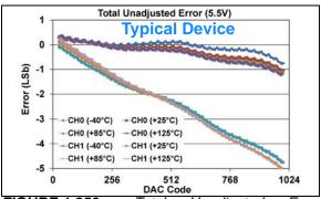
**FIGURE 1-259:** Total Unadjusted Error (V<sub>OUT</sub>) vs. DAC Code, and Temperature (Dual Channel - **MCP48FXB12**)
