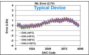
**FIGURE 1-101:** INL Error vs. DAC Code, and Temperature (Code 100 - 4000) (Single Channel - **MCP48FXB21**) (12-bit:  $V_{DD} = 2.7V$ ,  $V_{REF} = 1V$ , VRxB:VRxA = '10' ( $V_{REF}$  Unbuffered), Gx = '0' (1x)).
