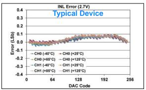
FIGURE 1-464: INL Error vs. DAC Code, and Temperature (Code 6 - 250) (Dual Channel - MCP48FXB02) (8-bit:  $V_{DD} = 2.7V$ ,  $V_{REF} = 1V$ , VRxB:VRxA = '10' ( $V_{RFF}$  Unbuffered), Gx = '0' (1x)).
