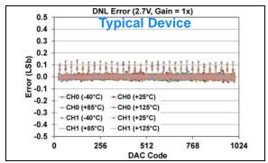
**FIGURE 1-399:** DNL Error vs. DAC Code, and Temperature (Code 25 - 1000) (Dual Channel - **MCP48FXB12**) (10-bit:  $V_{DD} = 2.7V$ ,  $V_{REF} = 2.048V$ ,  $VRxB:VRxA = '11' (V_{REF} Buffered)$ , Gx = '0' (1x)).
