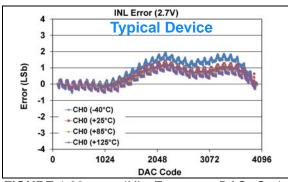
**FIGURE 1-83:** INL Error vs. DAC Code, and Temperature (Code 100 - 4000) (Single Channel - **MCP48FXB21**) (12-bit:  $V_{DD} = 2.7V$ ,  $V_{REF} = V_{DD}$ , VRxB:VRxA = '10' ( $V_{REF}$  Unbuffered), Gx = '0' (1x)).
