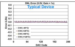
**FIGURE 1-503:** DNL Error vs. DAC Code, and Temperature (Code 6 - 250) (Single Channel - **MCP48FXB01**) (8-bit:  $V_{DD} = 5.5V$ ,  $V_{REF} = 2.048V$ ,  $VRxB:VRxA = '10' (V_{REF} Unbuffered)$ , Gx = '0' (1x)).
