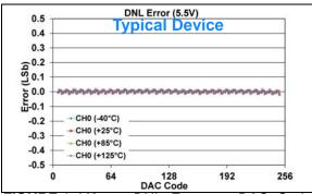
FIGURE 1-448: DNL Error vs. DAC Code, and Temperature (Code 6 - 250) (Single Channel - MCP48FXB01)
