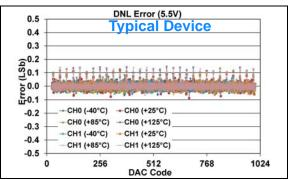
**FIGURE 1-289:** DNL Error vs. DAC Code, and Temperature (Code 25 - 1000) (Dual Channel - **MCP48FXB12**) (10-bit:  $V_{DD} = 5.5V$ ,  $V_{REF} = 1V$ , VRxB:VRxA = '10' ( $V_{RFF}$  Unbuffered), Gx = '0' (1x)).
