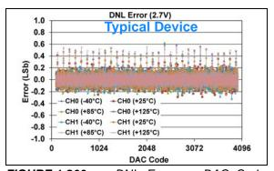
FIGURE 1-200: DNL Error vs. DAC Code, and Temperature (Code 100 - 4000) (Dual Channel - MCP48FXB22) (12-bit:  $V_{DD} = 2.7V$ ,  $V_{REF} = 1V$ , VRxB:VRxA = '11' ( $V_{REF}$  Buffered), Gx = '1' (2x).
