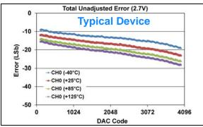
**FIGURE 1-167:** Total Unadjusted Error  $(V_{OUT})$  vs. DAC Code, and Temperature (Single Channel - **MCP48FXB21**) (12-bit:  $V_{DD} = 2.7V$ ,  $V_{REF} = 1V$ ,  $V_{RXB}:V_{RXA} = '11'$  ( $V_{RFF}$  Buffered),  $G_{X} = '0'$  (1x)).
