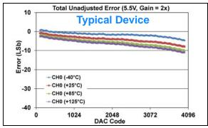
**FIGURE 1-130:** Total Unadjusted Error  $(V_{OUT})$  vs. DAC Code, and Temperature (Single Channel - **MCP48FXB21**) (**12-bit**:  $V_{DD} = 5.5V$ ,  $V_{REF} = 2.048V$ ,  $VRxB:VRxA = '10' (V_{REF} Unbuffered)$ , Gx = '1' (2x)).
