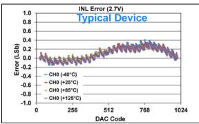
**FIGURE 1-371:** INL Error vs. DAC Code, and Temperature (Code 25 - 1000) (Single Channel - **MCP48FXB11**) (10-bit:  $V_{DD} = 2.7V$ ,  $V_{REF} = 1V$ ,  $V_{RXB}$ : $V_{RXA} = '11'$  ( $V_{REF}$  Buffered),  $G_{X} = '1'$  ( $Z_{X}$ ).
