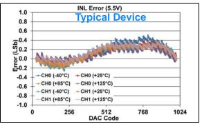
**FIGURE 1-301:** INL Error vs. DAC Code, and Temperature (Code 25 - 1000) (Dual Channel - **MCP48FXB12**) (10-bit:  $V_{DD} = 5.5V$ ,  $V_{REF} = 1V$ , VRxB:VRxA = '10' ( $V_{RFF}$  Unbuffered), Gx = '1' (2x)).
