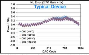
FIGURE 1-318: INL Error vs. DAC Code, and Temperature (Code 25 - 1000) (Single Channel - MCP48FXB11) (10-bit:  $V_{DD} = 2.7V$ ,  $V_{REF} = 2.048V$ ,  $VRxB:VRxA = '10' (V_{REF} Unbuffered)$ , Gx = '0' (1x)).
