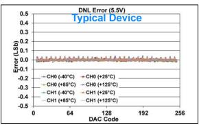
**FIGURE 1-559:** DNL Error vs. DAC Code, and Temperature (Code 6 - 250) (Dual Channel - **MCP48FXB02**) (8-bit:  $V_{DD} = 5.5V$ ,  $V_{REF} = 1V$ ,  $V_{RXB}:V_{RXA} = '11'$  ( $V_{REF}$  Buffered),  $G_{X} = '1'$  ( $Z_{X}$ ).
