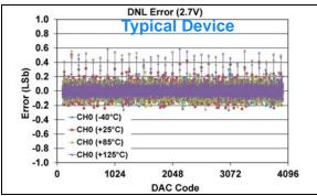
**FIGURE 1-179:** DNL Error vs. DAC Code, and Temperature (Code 100 - 4000) (Single Channel - **MCP48FXB21**) (12-bit:  $V_{DD} = 2.7V$ ,  $V_{REF} = 1V$ ,  $V_{RXB}:V_{RXA} = '11'$  ( $V_{RFF}$  Buffered),  $G_{X} = '0'$  (1x)).
