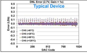
**FIGURE 1-252:** DNL Error vs. DAC Code, and Temperature (Code 25 - 1000) (Single Channel - **MCP48FXB11**) (10-bit:  $V_{DD} = 2.7V$ , VRxB:VRxA = '01' (Bandgap), Gx = '0' (1x)).
