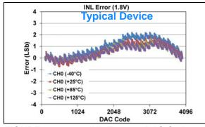
**FIGURE 1-102:** INL Error vs. DAC Code, and Temperature (Code 100 - 4000) (Single Channel - **MCP48FXB21**) (12-bit:  $V_{DD} = 1.8V$ ,  $V_{REF} = 1V$ ,  $V_{RXB}$ :  $V_{RXA} = '10'$  ( $V_{REF}$  Unbuffered),  $G_{X} = '0'$  (1x)).
