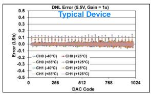
FIGURE 1-254: DNL Error vs. DAC Code, and Temperature (Code 25 - 1000) (Dual Channel - MCP48FXB12) (10-bit:  $V_{DD} = 5.5V$ , VRxB:VRxA = '01' (Bandgap), Gx = '0' (1x)).
