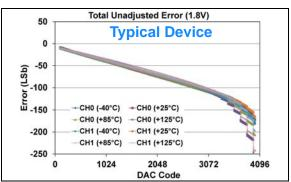
**FIGURE 1-153:** Total Unadjusted Error  $(V_{OUT})$  vs. DAC Code, and Temperature (Dual Channel - **MCP48FXB22**) (12-bit:  $V_{DD} = 1.8V$ ,  $V_{REF} = V_{DD}$ ,  $VRXB:VRXA = '11' (V_{REF} Buffered)$ , Gx = '0' (1x), (see **Appendix B.4** for additional information).
