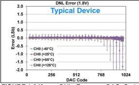
**FIGURE 1-342:** DNL Error vs. DAC Code, and Temperature (Code 25 - 1000) (Single Channel - **MCP48FXB11**) (10-bit:  $V_{DD} = 1.8V$ ,  $V_{REF} = V_{DD}$ , VRxB:VRxA = '11' ( $V_{REF}$  Buffered), Gx = '0' (1x)), (see **Appendix B.4** for additional information).
