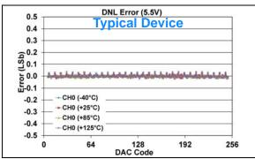
FIGURE 1-484: DNL Error vs. DAC Code, and Temperature (Code 6 - 250) (Single Channel - MCP48FXB01) (8-bit:  $V_{DD} = 5.5V$ ,  $V_{REF} = 1V$ , VRxB:VRxA = '10' ( $V_{REF}$  Unbuffered), Gx = '1' (2x).
