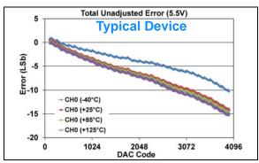
**FIGURE 1-40:** Total Unadjusted Error  $(V_{OUT})$  vs. DAC Code, and Temperature (Single Channel - **MCP48FXB21**) (12-bit:  $V_{DD} = 5.5V$ ,  $VRxB:VRxA = '00' (V_{DD})$ , Gx = '0' (1x)).
