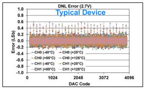
FIGURE 1-182: DNL Error vs. DAC Code, and Temperature (Code 100 - 4000) (Dual Channel - MCP48FXB22) (12-bit:  $V_{DD} = 2.7V$ ,  $V_{REF} = 1V$ , VRxB:VRxA = '11' ( $V_{RFF}$  Buffered), Gx = '0' (1x)).
