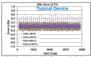
**FIGURE 1-107:** DNL Error vs. DAC Code, and Temperature (Code 100 - 4000) (Single Channel - **MCP48FXB21**) (12-bit:  $V_{DD} = 2.7V$ ,  $V_{REF} = 1V$ , VRXB:VRXA = '10' ( $V_{REF}$  Unbuffered), GX = '0' (1X)).
