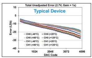
**FIGURE 1-135:** Total Unadjusted Error  $(V_{OUT})$  vs. DAC Code, and Temperature (Dual Channel - **MCP48FXB22**) (12-bit:  $V_{DD} = 2.7V$ ,  $V_{REF} = 2.048V$ ,  $VRxB:VRxA = '10' (V_{REF} Unbuffered)$ , Gx = '0' (1x)).
