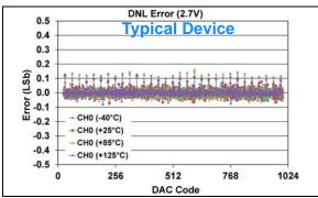
**FIGURE 1-377:** DNL Error vs. DAC Code, and Temperature (Code 25 - 1000) (Single Channel - **MCP48FXB11**) (10-bit:  $V_{DD} = 2.7V$ ,  $V_{REF} = 1V$ ,  $V_{RXB}:V_{RXA} = '11'$  ( $V_{RFF}$  Buffered),  $G_{X} = '1'$  ( $Z_{X}$ ).
