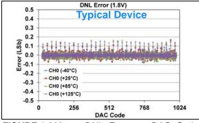
**FIGURE 1-360:** DNL Error vs. DAC Code, and Temperature (Code 25 - 1000) (Single Channel - **MCP48FXB11**) (10-bit:  $V_{DD} = 1.8V$ ,  $V_{REF} = 1V$ ,  $V_{RXB}:V_{RXA} = '11'$  ( $V_{REF}$  Buffered),  $G_{X} = '0'$  (1x)).
