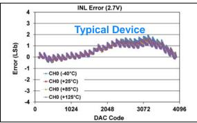
FIGURE 1-47: INL Error vs. DAC Code, and Temperature (Code 100 - 4000) (Single Channel - MCP48FXB21) (12-bit:  $V_{DD} = 2.7V$ ,  $VRxB:VRxA = '00' (V_{DD})$ , Gx = '0' (1x)).
