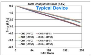
**FIGURE 1-511:** Total Unadjusted Error  $(V_{OUT})$  vs. DAC Code, and Temperature (Dual Channel - **MCP48FXB02**) (8-bit:  $V_{DD} = 5.5V$ ,  $V_{REF} = V_{DD}$ ,  $VRxB:VRxA = '11' (V_{REF} Buffered)$ , Gx = '0' (1x)).
