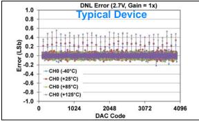
**FIGURE 1-144:** DNL Error vs. DAC Code, and Temperature (Code 100 - 4000) (Single Channel - **MCP48FXB21**) (12-bit:  $V_{DD} = 2.7V$ ,  $V_{REF} = 2.048V$ ,  $VRxB:VRxA = '10' (V_{REF} Unbuffered)$ , Gx = '0' (1x)).
