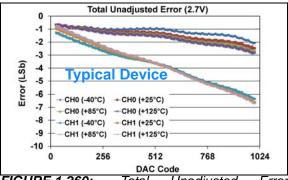
**FIGURE 1-260:** Total Unadjusted Error  $(V_{OUT})$  vs. DAC Code, and Temperature (Dual Channel - **MCP48FXB12**)  $(10\text{-bit}: V_{DD} = 2.7V, V_{REF} = V_{DD},$
