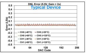
**FIGURE 1-577:** DNL Error vs. DAC Code, and Temperature (Code 6 - 250) (Dual Channel - **MCP48FXB02**) (8-bit:  $V_{DD} = 5.5V$ ,  $V_{REF} = 2.048V$ ,  $VRxB:VRxA = '11' (V_{REF} Buffered)$ , Gx = '1' (2x)).
