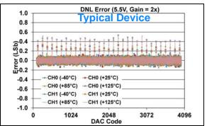
FIGURE 1-145: DNL Error vs. DAC Code, and Temperature (Code 100 - 4000) (Dual Channel - MCP48FXB22) (12-bit:  $V_{DD} = 5.5V$ ,  $V_{REF} = 2.048V$ ,  $VRxB:VRxA = '10' (V_{REF} Unbuffered)$ , Gx = '1' (2x)).
