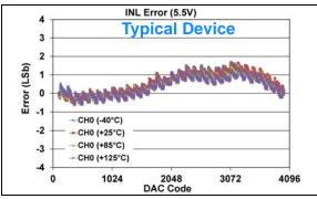
FIGURE 1-172: INL Error vs. DAC Code, and Temperature (Code 100 - 4000) (Single Channel - MCP48FXB21) (12-bit:  $V_{DD} = 5.5V$ ,  $V_{REF} = 1V$ , VRxB:VRxA = '11' ( $V_{REF}$  Buffered), Gx = '0' (1x)).
