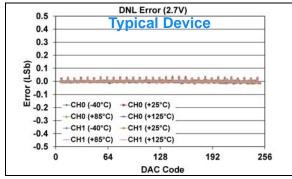
FIGURE 1-416: DNL Error vs. DAC Code, and Temperature (Code 6 - 250) (Dual Channel - MCP48FXB02) (8-bit:  $V_{DD} = 2.7V$ ,  $VRxB:VRxA = '00' (V_{DD})$ , Gx = '0' (1x)).
