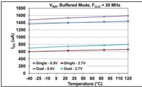
**FIGURE 1-20:** Average Device Supply Current - Active Interface ( $I_{DDA}$ ) ( $F_{SCK} = 20 \text{ MHz}$ ) vs. Voltage and Temperature,
