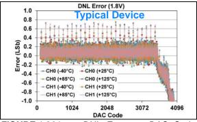
**FIGURE 1-201:** DNL Error vs. DAC Code, and Temperature (Code 100 - 4000) (Dual Channel - **MCP48FXB22**) (12-bit:  $V_{DD} = 1.8V$ ,  $V_{REF} = 1V$ , VRxB:VRxA = '11' ( $V_{REF}$  Buffered), Gx = '1' (2x), (see **Appendix B.5** for additional information).
