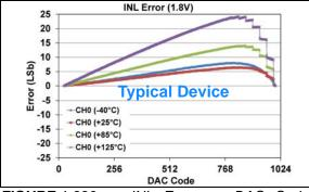
**FIGURE 1-336:** INL Error vs. DAC Code, and Temperature (Code 25 - 1000) (Single Channel - **MCP48FXB11**) (10-bit:  $V_{DD} = 1.8V$ ,  $V_{REF} = V_{DD}$ ,  $VRxB:VRxA = '11' (V_{REF} Buffered)$ , Gx = '0' (1x), (see **Appendix B.4** for additional information).
