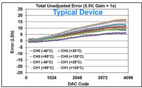
**FIGURE 1-62:** Total Unadjusted Error  $(V_{OUT})$  vs. DAC Code, and Temperature (Dual Channel - **MCP48FXB22**) (12-bit:  $V_{DD} = 5.5V$ , VRxB:VRxA = '01' (Bandgap), Gx = '0' (1x)).
