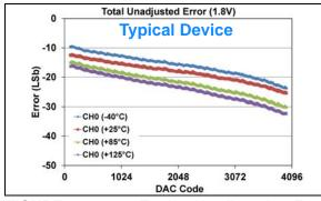
**FIGURE 1-168:** Total Unadjusted Error  $(V_{OUT})$  vs. DAC Code, and Temperature (Single Channel - **MCP48FXB21**) (12-bit:  $V_{DD} = 1.8V$ ,  $V_{REF} = 1V$ ,  $V_{RXB}:V_{RXA} = '11'$  ( $V_{REF}$  Buffered),  $G_{X} = '0'$  ( $I_{X}$ ).
