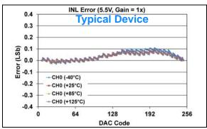
**FIGURE 1-569:** INL Error vs. DAC Code, and Temperature (Code 6 - 250) (Single Channel - **MCP48FXB01**) (8-bit:  $V_{DD} = 5.5V$ ,  $V_{REF} = 2.048V$ ,  $VRxB:VRxA = '11' (V_{REF} Buffered)$ , Gx = '0' (1x)).
