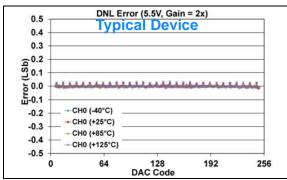
FIGURE 1-502: DNL Error vs. DAC Code, and Temperature (Code 6 - 250) (Single Channel - MCP48FXB01) (8-bit:  $V_{DD} = 5.5V$ ,  $V_{REF} = 2.048V$ ,  $VRxB:VRxA = '10' (V_{REF} Unbuffered)$ , Gx = '1' (2x)).
