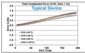
**FIGURE 1-418:** Total Unadjusted Error  $(V_{OUT})$  vs. DAC Code, and Temperature (Single Channel - **MCP48FXB01**) (8-bit:  $V_{DD} = 5.5V$ , VRxB:VRxA = '01' (Bandgap), Gx = '1' (2x)).
