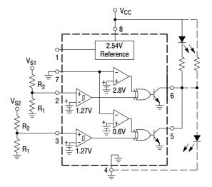
The above figure shows the MC34161 configured as a dual positive undervoltage detector. As the input voltage decreases towards ground, the LED will turn 'ON' when V<sub>S1</sub> or V<sub>S2</sub> falls below V<sub>1</sub>. With the dashed line output connection, the circuit becomes a dual positive overvoltage detector. As the input voltage increases from ground, the LED will turn 'ON' when V<sub>S1</sub> or V<sub>S2</sub> exceeds V<sub>2</sub>.
