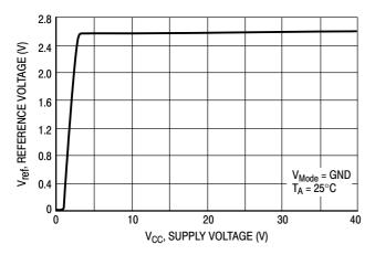
Figure 8. Reference Voltage versus Supply Voltage
