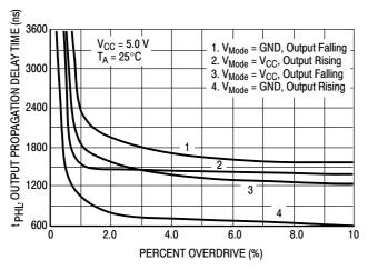
Figure 4. Output Propagation Delay Time versus Percent Overdrive
