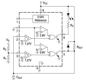
The above figure shows the MC34161 configured as a microprocessor reset with a time delay. Channel 2 monitors input voltage  $V_S$  while channel 1 performs the time delay function. As the input voltage decreases towards ground, the output of channel 2 quickly discharges  $C_{DLY}$  when  $V_S$  falls below  $V_1$ . As the input voltage increases from ground, the output of channel 2 allows  $R_{DLY}$  to charge  $C_{DLY}$  when  $V_S$  exceeds  $V_2$ .
