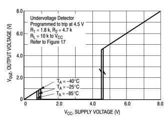
Figure 5. Output Voltage versus Supply Voltage
