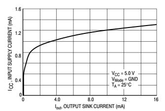
Figure 13. Supply Current versus Output Sink Current
