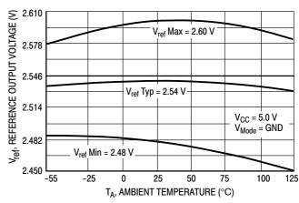
Figure 9. Reference Voltage versus Ambient Temperature
