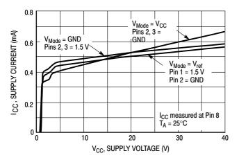
Figure 12. Supply Current versus Supply Voltage
