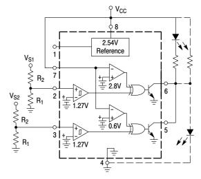
The above figure shows the MC34161 configured as a dual positive overvoltage detector. As the input voltage increases from ground, the LED will turn 'ON' when VS1 or VS2 exceeds V2. With the dashed line output connection, the circuit becomes a dual positive undervoltage detector. As the input voltage decreases from the peak towards ground, the LED will turn 'ON' when V<sub>S1</sub> or V<sub>S2</sub> falls below V<sub>1</sub>.
