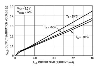
Figure 11. Output Saturation Voltage versus Output Sink Current
