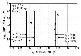
Figure 2. Comparator Input Threshold Voltage
