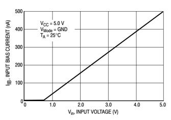
Figure 3. Comparator Input Bias Current versus Input Voltage
