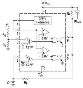
The above figure shows the MC34161 configured as an overvoltage detector with an audio alarm. Channel 1 monitors input voltage  $V_S$  while channel 2 is connected as a simple RC oscillator. As the input voltage increases from ground, the output of channel 1 allows the oscillator to turn 'ON' when  $V_S$  exceeds  $V_2$ .
