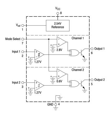
Figure 14. MC34161 Representative Block Diagram
