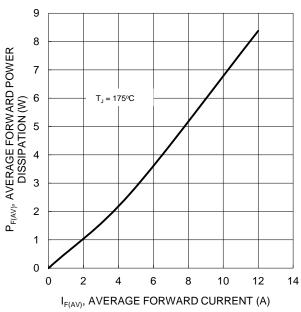
Figure 1 Forward Power Dissipation
