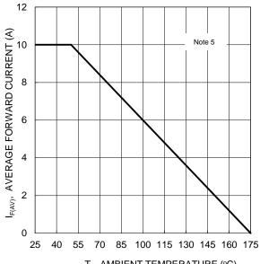
${\rm T_{A}}$ , AMBIENT TEMPERATURE (°C) Figure 4 Forward Current Derating
