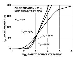
Figure 5. Transfer Characteristics
