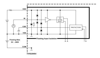
Figure 5: Floating PWM Input Structure
