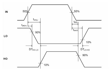
Figure 1: Switching Time Waveform Definitions
