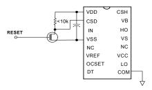
**Figure 10: Latched Protection Configuration**
