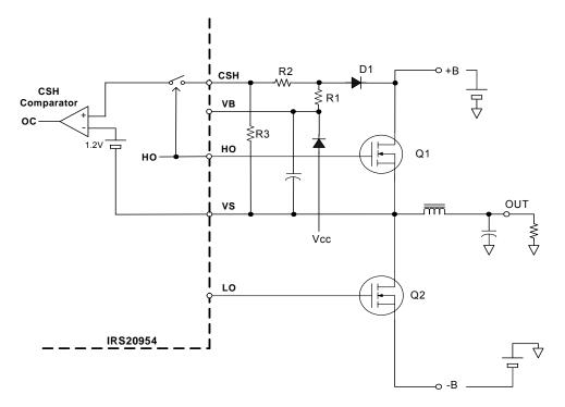
Figure 14: Programming High-side Over-Current Threshold
