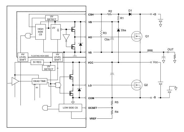
Figure 12: Bi-Directional Over-Current Protection
