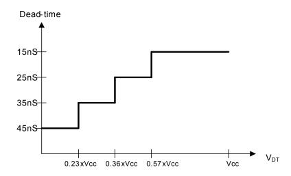
Figure 16: Deadtime Settings vs. V<sub>DT</sub> Voltage
