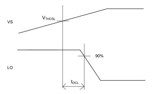
Figure 4:  $V_s > V_{TH,SCL}$  to Shutdown Waveform Definitions
