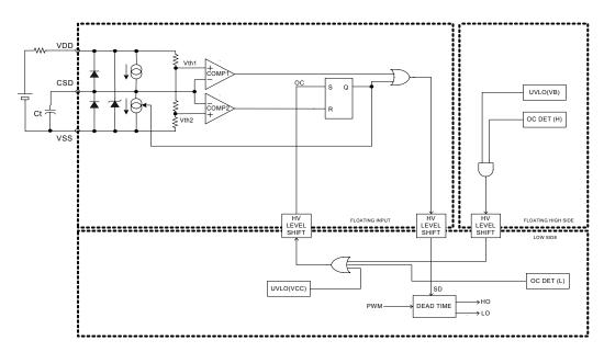
Figure 7: Shutdown Functional Block Diagram
