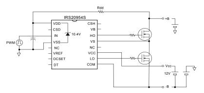
Figure 18: Supplying VDD
