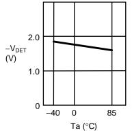
1.32 Low supply voltage release voltage +V<sub>DET</sub> vs. ambient temperature Ta
