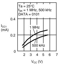
1. 6 Current consumption (READ) I<sub>CC1</sub> vs. Clock frequency f<sub>SK</sub>
