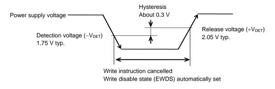
Figure 20 Operation during Low Power Supply Voltage
