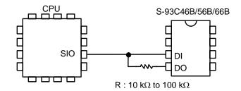
Figure 22 Connection of 3-Wire Interface
