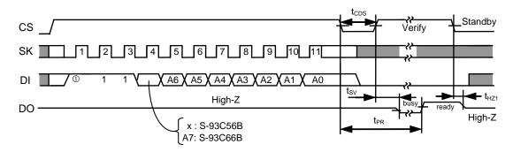
Figure 13 Data Erase Timing (S-93C56B, S-93C66B)
