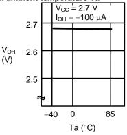
1.19 High-level output voltage V<sub>OH</sub> vs. ambient temperature Ta
