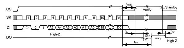
Figure 10 Data Write Timing (S-93C46B)
