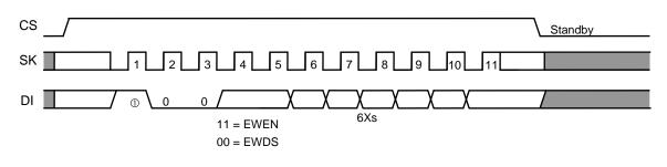
Figure 19 Write Enable / Disable Timing (S-93C56B, S-93C66B)
