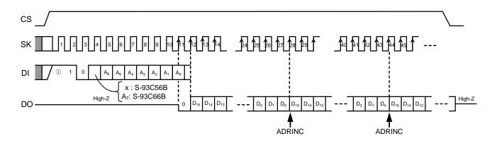
Figure 9 Read Timing (S-93C56B, S-93C66B)
