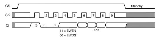
Figure 18 Write Enable / Disable Timing (S-93C46B)
