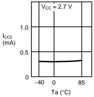
1. 11 Current consumption in standby mode I<sub>SB</sub> vs. ambient temperature Ta
