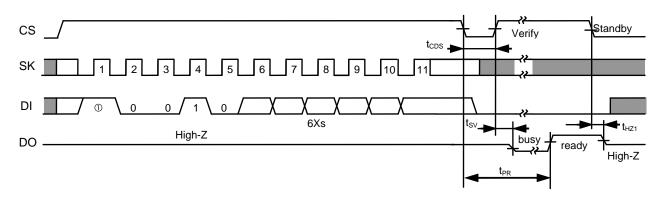
Figure 17 Chip Erase Timing (S-93C56B, S-93C66B)
