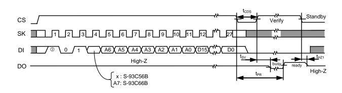
Figure 11 Data Write Timing (S-93C56B, S-93C66B)
