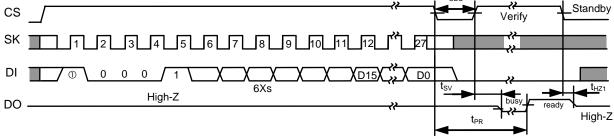
Figure 15 Chip Write Timing (S-93C56B, S-93C66B)
