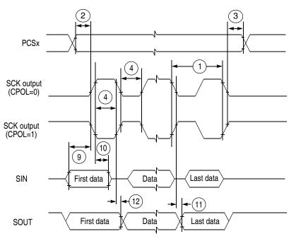
Figure 17. DSPI Classic SPI Timing—Master, CPHA = 0
