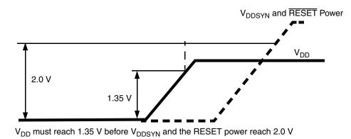
Figure 3. Power-Up Sequence (V<sub>BC33</sub> Grounded)
