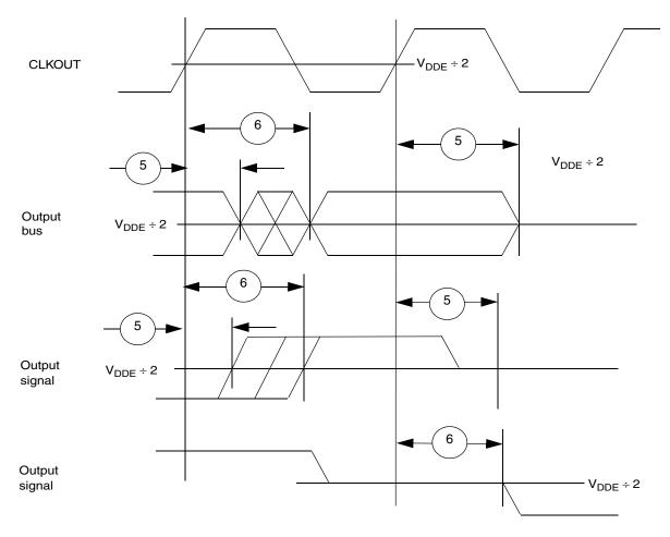
Figure 13. Synchronous Output Timing
