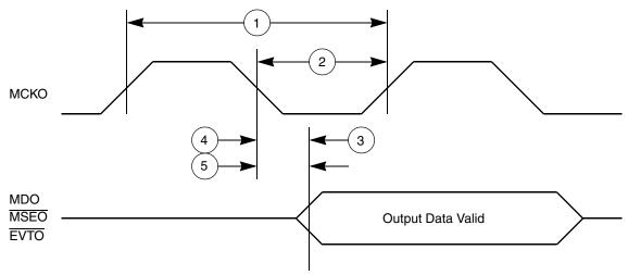
Figure 10. Nexus Output Timing
