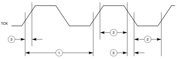
Figure 6. JTAG Test Clock Input Timing
