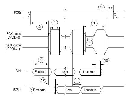
Figure 21. DSPI Modified Transfer Format Timing—Master, CPHA = 0
