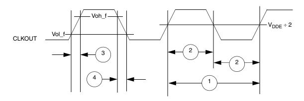
Figure 12. CLKOUT Timing
