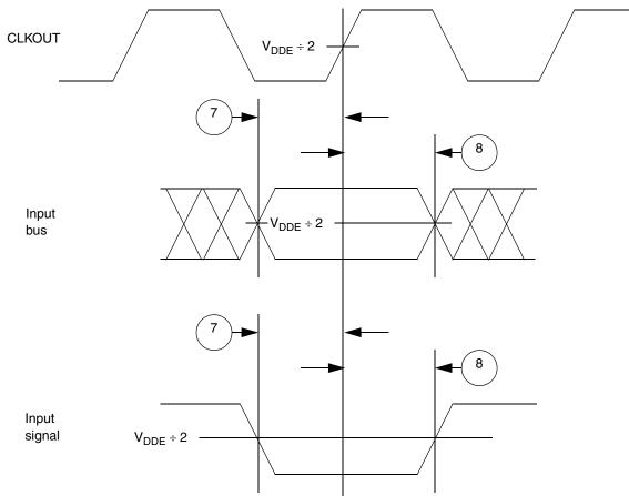
Figure 14. Synchronous Input Timing
