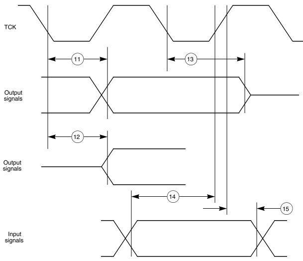
Figure 9. JTAG Boundary Scan Timing
