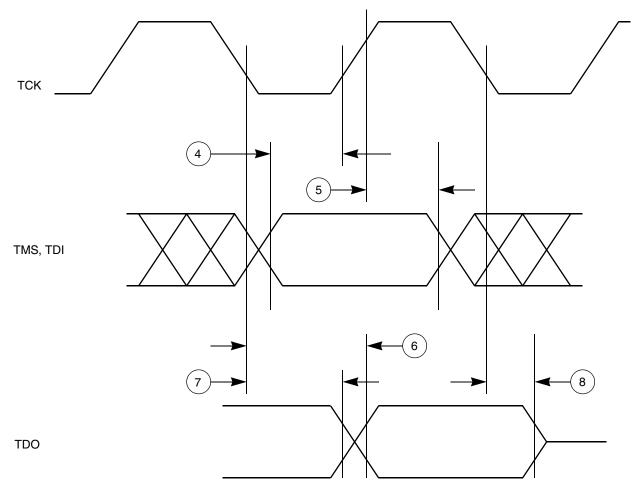
Figure 7. JTAG Test Access Port Timing
