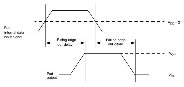
Figure 4. Pad Output Delay
