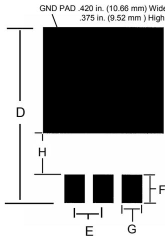
PINS ON .1 in. CENTERS PROVIDE COMPATIBILITY WITH BREADBOARDS AND SOCKETS. TWO PINS ARE PROVIDED FOR EACH DEVICE LEAD FOR GREATER CURRENT CAPACITY.
