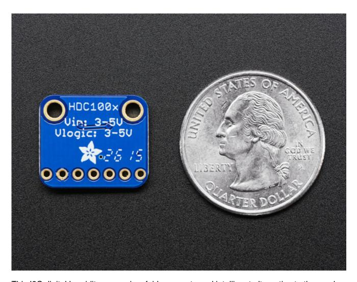
This I2C digital humidity sensor is a fairly accurate and intelligent alternative to the much simpler <a href="Humidity and Temperature Sensor - SHT15 Breakout">Humidity and Temperature Sensor - SHT15 Breakout</a> (http://adafru.it/1638) It has a typical accuracy of ±4% with an operating range that's optimized from 10% to 80% RH. Operation outside this range is still possible - just the accuracy might drop a bit. The temperature output has a typical accuracy of ±0.2°C from -20~85°C.
