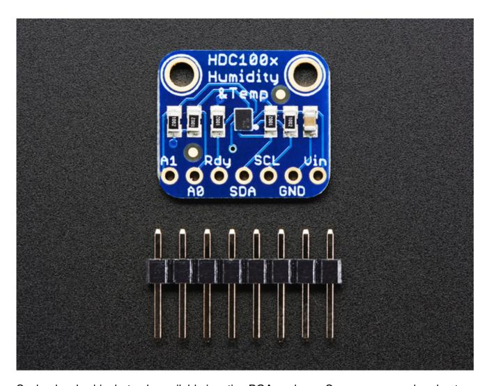
Such a lovely chip, but only available in a tiny BGA package. So we spun up a breakout board with the chip and some extra passive components to make it easy to use. Each order comes with one fully assembled and tested PCB breakout and a small piece of header. You'll need to solder the header onto the PCB but it's fairly easy and takes only a few minutes even for a beginner.
