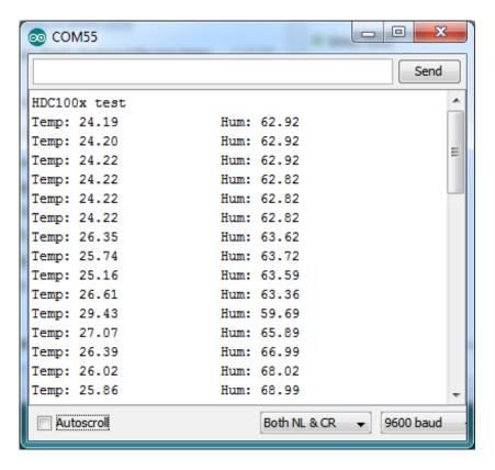
**Please note:** TI has indicated that there's a 'settling' effect for the humidity and that you will need to re-hydrate the sensor once you receive it. To rehydrate it, place it in a location with 85% humidity for 24 hours or 60% humidity for 10 days.
