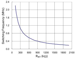
Figure 2. Switching Frequency vs. R<sub>RT</sub>
