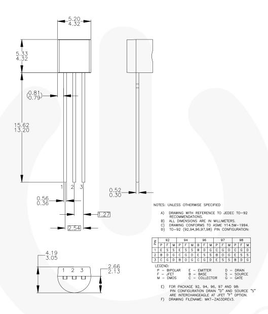
Figure 11. 3-LEAD, TO-92, MOLDED, STD STRAIGHT LD (NO EOL CODE)
