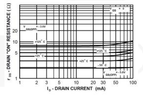
Figure 6. On Resistance vs. Drain Current
