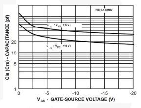
Figure 4. Capacitance vs. Voltage
