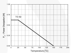
Figure 10. Power Dissipation vs. Ambient Temperature
