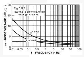
Figure 9. Noise Voltage vs. Frequency
