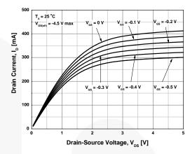
Figure 2. Common Drain-Source Characteristics
