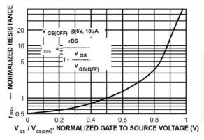
Figure 5. Normalized Drain Resistance vs. Bias Voltage
