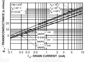
Figure 8. Transconductance vs. Drain Current
