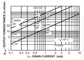
Figure 7. Output Conductance vs. Drain Current
