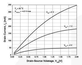
**Figure 1. Common Drain-Source Characteristics**
