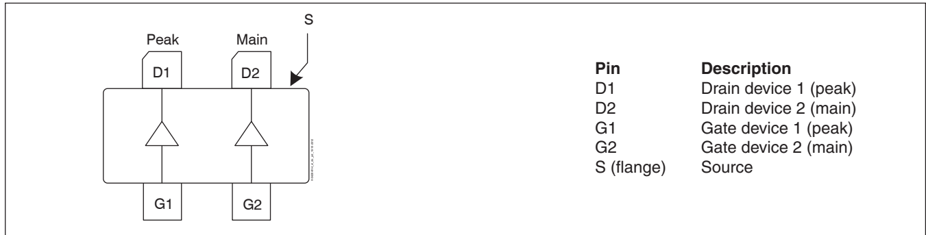
Lead connections for PTAC260302FC
