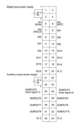
DI1 through DI8 are digital input terminals and SUBOUT3 through SUBOUT10 are digital auxiliary output terminals, both sets of which can be allocated as instructed by the user's software. The terminals without allocation prior to shipping can be freely allocated as required by the user.
