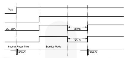
Figure 7. I<sup>2</sup>C Reset Mode Timing
