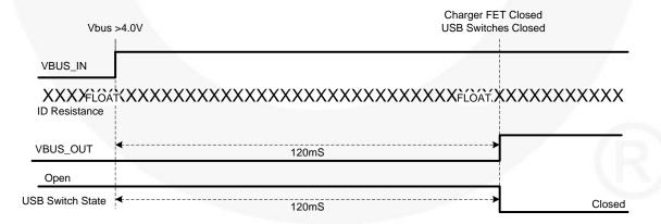
Figure 9. USB Standard Downstream Port Attach Timing<sup>(20)</sup>
