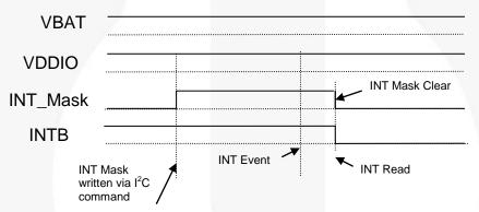
Figure 8. INT Mask to INTB Interrupt Timing Diagram
