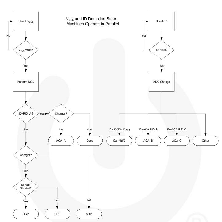
Figure 5. Accessory Discovery State Machine Flow Diagram
