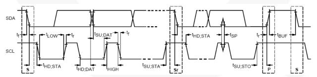
Figure 6. Definition of Timing for Full-Speed Mode Devices on the I<sup>2</sup>C Bus<sup>®</sup>
