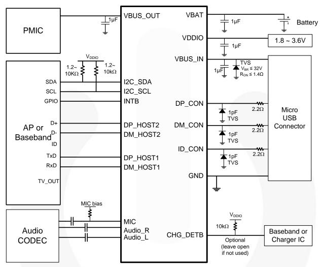
Figure 13. Reference Schematic
