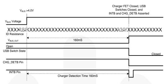
Figure 10. USB Dedicated Charging Port (DCP) or Charging Downstream Port (CDP) Attach Timing (20)
