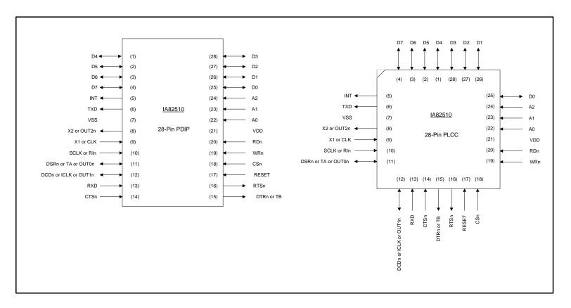
Figure 1. Package Pinout
