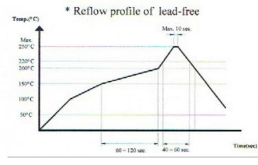
Recommendable wave soldering condition is as follows: Note 1: It is requested that reflow soldering should be executed after heat of product goes down to normal temperature. Note 2: Peak reflow temperature of 250°C maximum of 10 seconds, with a maximum duration of 40-60 seconds between 220°C and 250°C
