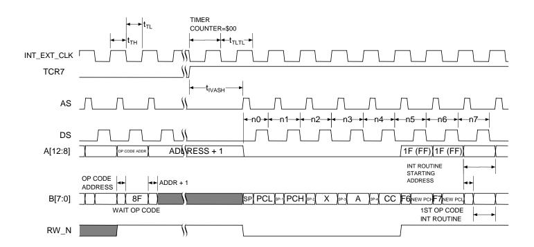
Figure 17. Timer Interrupt After WAIT Instruction Timing
