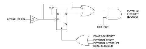
Figure 9. Interrupt Functional Diagram
