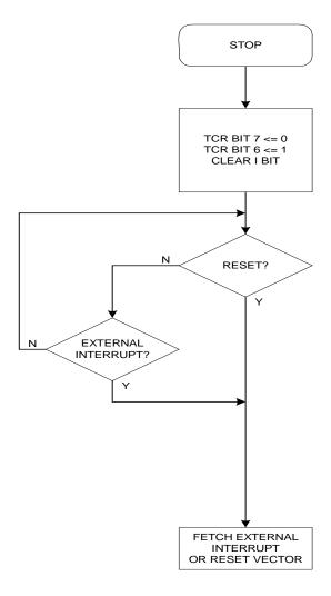
**Figure 11. STOP Function Flowchart**
