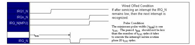
Figure 10. Interrupt Mode Diagram
