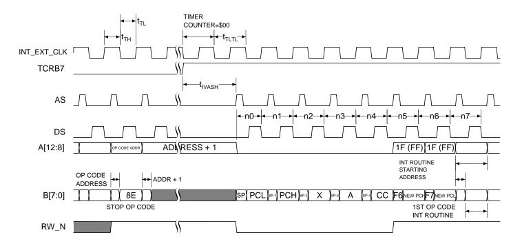
Figure 18. Interrupt Recovery From STOP Instruction Timing
