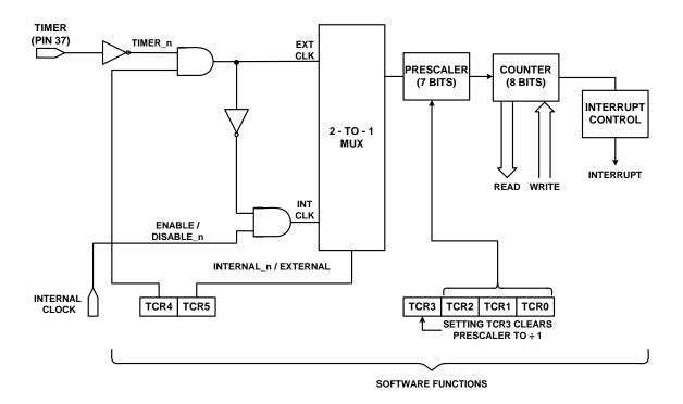
Figure 13. Timer Block Diagram
