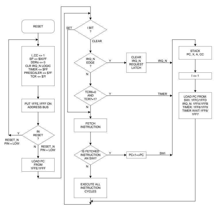
Figure 8. Reset and Interrupt Processing Flowchart
