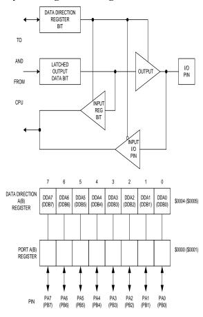
Figure 2. PA0-PA7/PB0-PB7 (Input/Output Lines)
