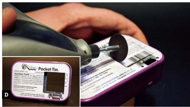
soldering, to insulate all connections from the conductive metal tin. Fig. C: It's a snug fit. Fig. D: Use light pressure when cutting the openings; let the tool do the work. The openings don't have to be perfectly aligned.
