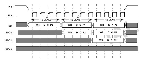
FIGURE 19. DAISY CHAIN WRITE SEQUENCE OF N = 3 DCP
