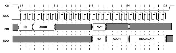
FIGURE 17. FOUR BYTE READ SEQUENCE
