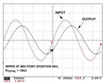
FIGURE 12. FREQUENCY RESPONSE (1MHz)
