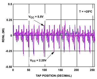
FIGURE 7. DNL vs TAP POSITION IN RHEOSTAT MODE FOR  $10k\Omega$  (W)
