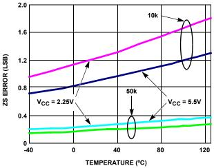
FIGURE 5. ZS ERROR vs TEMPERATURE
