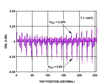
FIGURE 3. DNL vs TAP POSITION IN VOLTAGE DIVIDER MODE FOR 10k $\Omega$  (W)
