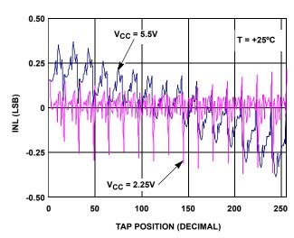
FIGURE 4. INL vs TAP POSITION IN VOLTAGE DIVIDER MODE FOR  $10k\Omega$  (W)
