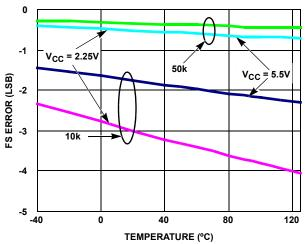
FIGURE 6. FS ERROR vs TEMPERATURE
