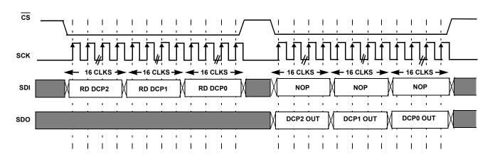
FIGURE 21. DAISY CHAIN READ SEQUENCE OF N = 3 DCP
