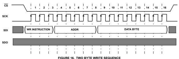
FIGURE 16. TWO BYTE WRITE SEQUENCE
