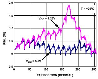
FIGURE 8. INL vs TAP POSITION IN RHEOSTAT MODE FOR  $10k\Omega$  (W)
