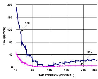
FIGURE 10. TC FOR VOLTAGE DIVIDER MODE IN ppm
