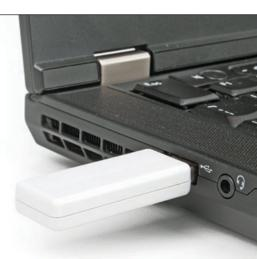
Figure 1-3: USB Dongle plugged into Laptop USB host connector
