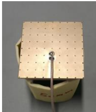
Ground above antenna
