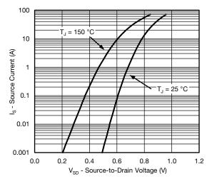
**Source Drain Diode Forward Voltage**
