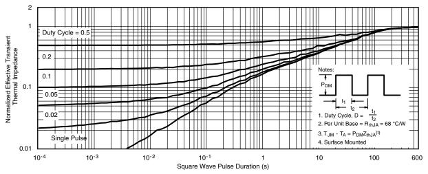
Normalized Thermal Transient Impedance, Junction-to-Ambient
