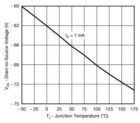
**Drain Source Breakdown vs. Junction Temperature**
