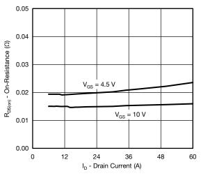
**On-Resistance vs. Drain Current**
