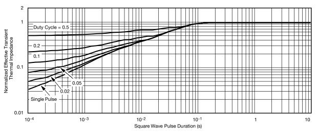
Normalized Thermal Transient Impedance, Junction-to-Case
