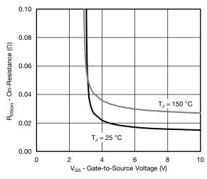
On-Resistance vs. Gate-to-Source Voltage
