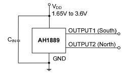
Note: 4. C<sub>IN</sub> is for power stabilization and to strengthen the noise immunity, the recommended capacitance 100nF typical.
