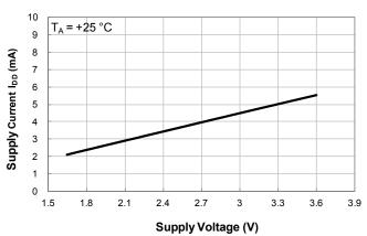
Supply Current vs. Supply Voltage
