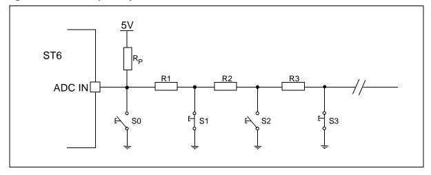
Depending on the identified key, a direct signal activation can be achieved or a selective jump in the program flow can be performed.
