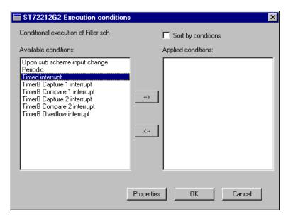
In the example, the microcontroller ST72212G2 has had one of its peripherals, Timer B, enabled. The resulting choice of execution conditions are:
