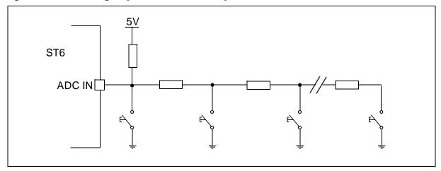
When a key is pressed, the voltage at the ADC input is given by the activated voltage divider, generating a different voltage at the ADC input for each key that is pressed. If the top key is pressed, the voltage measured is zero while the default voltage at the ADC input (if no key is pressed) is Vdd.
