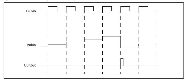
Each Modulo-N block is based on a Counter component provided within the ST-Realizer standard library. This symbol presents the advantage of generating a numeric variable as
