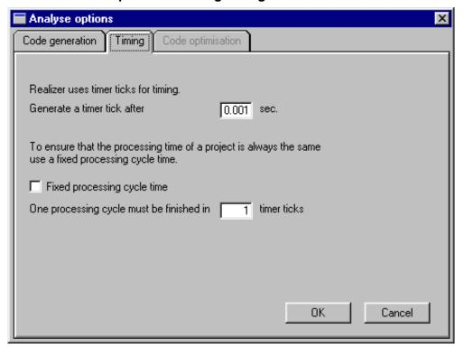
Every ST6 or ST7 microcontroller has a timer, called Timer 1 (ST6) or Timer A (ST7), which (if there are either time-related symbols or events in the application) is used as the base clock to measure out units of time called "timer ticks". Timer ticks are the smallest increment of time that a timer can count. In this dialog box, you may choose the value for the "timer tick" or base clock unit used in the application.
