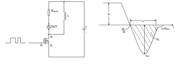
t<sub>RR</sub> Test Circuit
