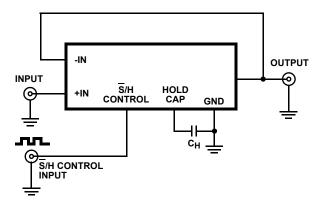
FIGURE 1. HOLD STEP ERROR AND DRIFT CURRENT
