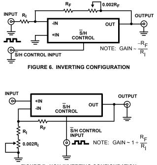
FIGURE 7. NON-INVERTING CONFIGURATION
