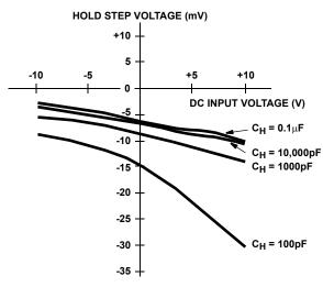
FIGURE 5. HOLD STEP vs INPUT VOLTAGE
