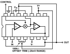
FIGURE 8. BASIC SAMPLE-AND-HOLD (TOP VIEW)
