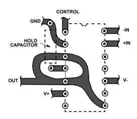
FIGURE 9. GUARD RING LAYOUT (BOTTOM VIEW)
