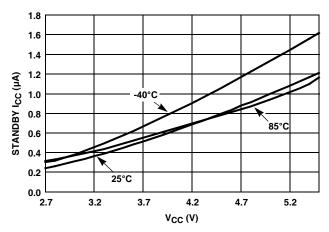
FIGURE 2. STANDBY  $I_{CC}$  vs  $V_{CC}$
