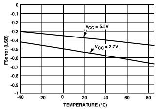
FIGURE 6. FSerror vs TEMPERATURE
