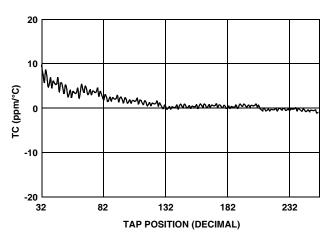
FIGURE 10. TC FOR VOLTAGE DIVIDER MODE IN ppm
