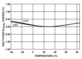
FIGURE 9. END TO END R<sub>TOTAL</sub> % CHANGE vs TEMPERATURE
