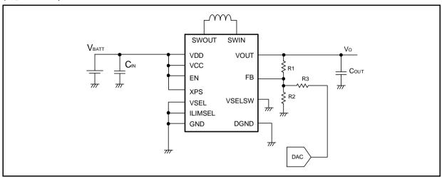
Relationship between DAC and output when setting to R1 = 620 k $\Omega$ , R2 = 110 k $\Omega$  and R3 = 330 k $\Omega$
