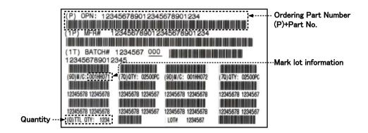
Figure 22-4 Reel label [Dry pack & Reel label (4 x 2.5inch)]
