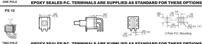
**EPOXY SEALED P.C. TERMINALS ARE SUPPLIED AS STANDARD FOR THESE OPTIONS.**
