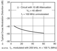
Fig. 3 - Typ. Cross Modulation Distortion vs. Frequency f<sub>2</sub>
