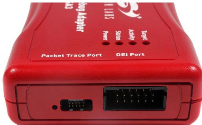
Figure 1. Debug Adapter (ISA3) Front Panel (Packet Trace Port, DEI, Factory Defaults)
