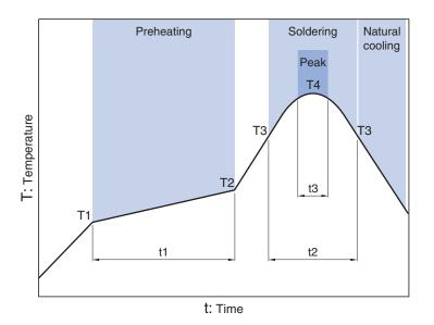
Preheating Soldering Peak Temp. Temp. Time Time Temp. Time T1 T2 **T**4 t1 тз t2 t3 150°C 180°C 90 to 120s 230°C 255°C 10s max. 40s
