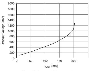
Figure 2. Dropout Voltage vs. I<sub>OUT2</sub>
