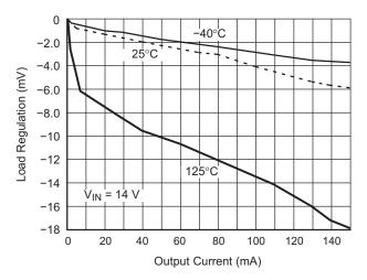
Figure 16. Load Regulation vs. Output Current fo V<sub>OUT2</sub>
