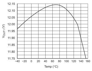
Figure 4. V<sub>OUT1</sub> vs. Temperature
