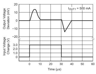
Figure 8. Line Transient Response (VOUT1)
