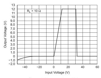
Figure 3. V<sub>OUT1</sub> vs. Input Voltage
