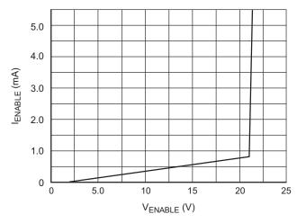
Figure 7. ENABLE Current vs. ENABLE Voltage
