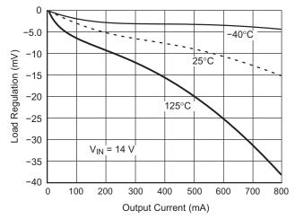
Figure 18. Load Regulation vs. Output Current for V<sub>OUT1</sub>
