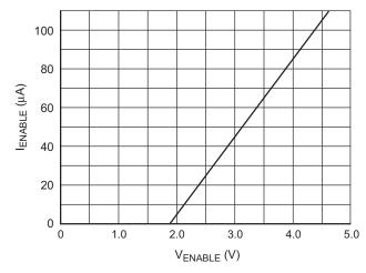
Figure 6. ENABLE Current vs. ENABLE Voltage
