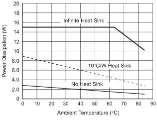
Figure 12. Maximum Power Dissipation (TO-220)
