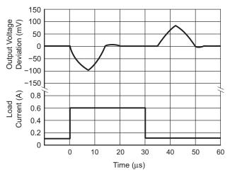
Figure 10. Load Transient Response (V<sub>OUT1</sub>)
