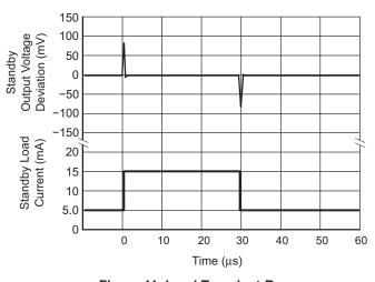
Figure 11. Load Transient Response (V<sub>OUT2</sub>)
