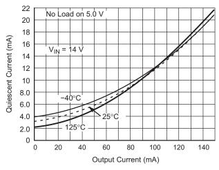
Figure 14. Quiescent Current vs. Output Current for V<sub>OUT1</sub>
