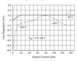
Figure 15. Line Regulation vs. Output Current for V<sub>OUT2</sub>
