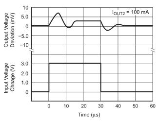
Figure 9. Line Transient Response (V<sub>OUT2</sub>)
