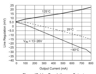
Figure 17. Line Regulation vs. Output Current for V<sub>OUT1</sub>
