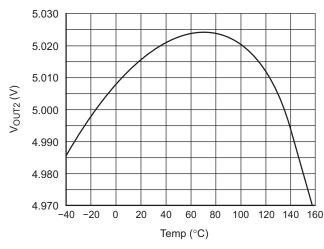
Figure 5. V<sub>OUT2</sub> vs. Temperature
