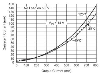
Figure 13. Quiescent Current vs. Output Current for V<sub>OUT2</sub>
