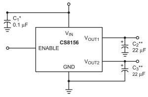
$^{*}$  C<sub>1</sub> is required if the regulator is far from power supply filter.
