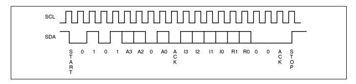
The Increment/Decrement command is different from the other commands. Once the command is issued and the X9428 has responded with an acknowledge, the master can clock the selected wiper up and/or down in one segment steps; thereby, providing a fine tuning capability to the host. For each SCL clock pulse ( $t_{\mbox{HIGH}}$ ) while SDA is HIGH, the selected wiper will
