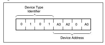
The next four bits of the slave address are the device address. The physical device address is defined by the state of the  $A_0$ ,  $A_2$ ,  $A_3$  inputs. The X9428 compares the serial data stream with the address input state; a successful compare of all four address bits is required for the X9428 to respond with an acknowledge. The  $A_0$ ,  $A_2$ ,  $A_3$  inputs can be actively driven by CMOS input signals or tied to  $V_{CC}$  or  $V_{SS}$ .
