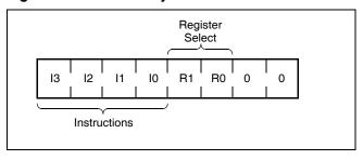
The four high order bits define the instruction. The next two bits (R1 and R0) select one of the four registers that is to be acted upon when a register oriented instruction is issued. Bits 0 and 1 are defined to be 0.
