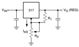
$V_{O}(REG) = 1.25V (1+R_2/R_1)+I_{adj} R_2$
