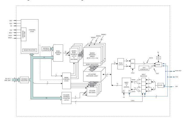
Figure 5: 16 Meg x 16 Functional Block Diagram
