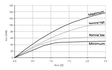
Figure 14: Full Drive Pull-Up Characteristics
