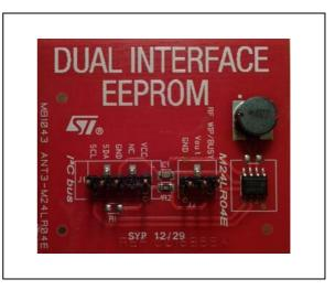
The ANT3-M24LR04E antenna allows system designers to evaluate the M24LR04E-R performance and capabilities, and to get started with their design.
