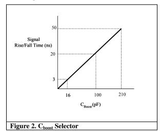
The boost capacitor in parallel with the current-limiting resistor boosts the instantaneous coil current at the signal transition. This ensures switching and reduces propagation delay and reduces pulse-width distortion.
