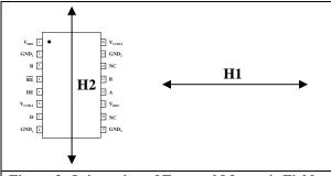
Figure 3. Orientation of External Magnetic Field
