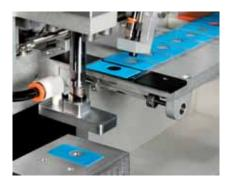
Bergquist Sil-Pad 1500ST (Soft Tack) is a fiberglass reinforced thermal interface material that is naturally tacky on both sides. Sil-Pad 1500ST exhibits superior thermal performance when compared to the competitors' thermal interface materials. Sil-Pad 1500ST is supplied in sheet or roll form for exceptional auto-dispensing and auto-placement in high volume assemblies. Sil-Pad 1500ST is intended for placement between an electronic power device and its heat sink.
