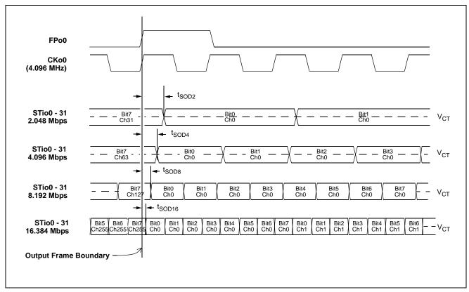
Figure 38 - GCI-Bus Output Timing Diagram when Operated at 2, 4, 8 or 16 Mbps
