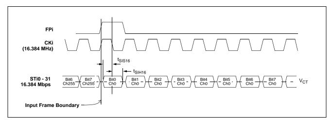
Figure 36 - GCI-Bus Input Timing Diagram when Operated at 16 Mbps
