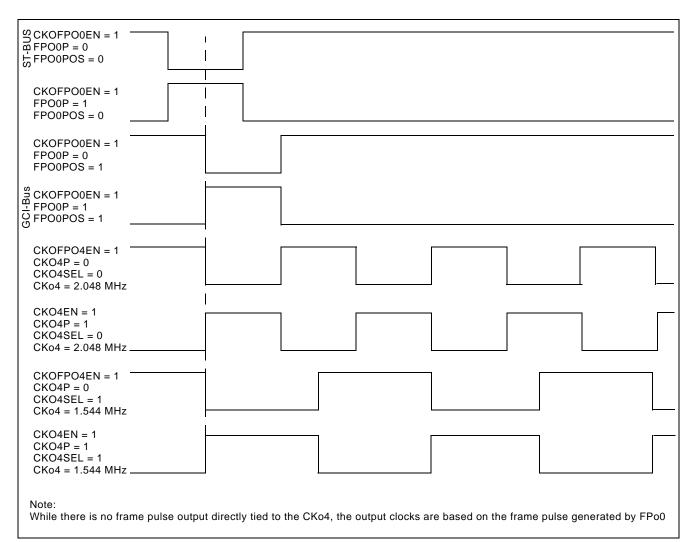
Figure 11 - Output Timing for CKo4
