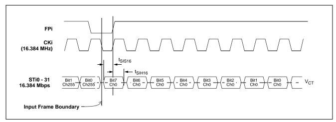
Figure 34 - ST-BUS Input Timing Diagram when Operated at 16 Mbps
