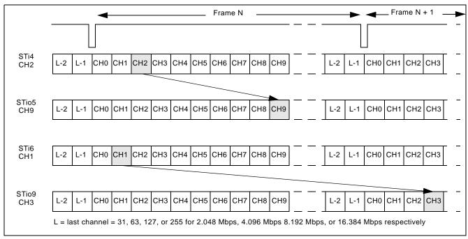
Figure 19 - Data Throughput Delay for Variable Delay
