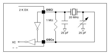
Figure 23 - Crystal Oscillator Circuit
