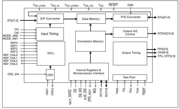
Figure 1 - ZL50019 Functional Block Diagram
