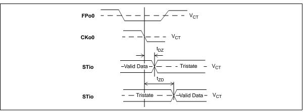
Figure 39 - Serial Output and External Control
