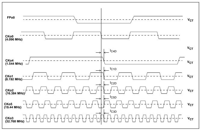
Figure 49 - Output Timing (ST-BUS Format)
