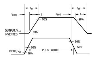
Figure 11. Switching Waveforms
