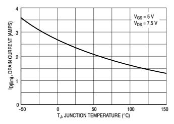
Figure 3. I<sub>D(lim)</sub> Variation With Temperature
