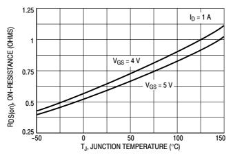
Figure 5. On-Resistance Variation With Temperature
