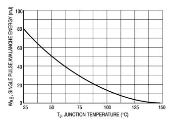
Figure 6. Single Pulse Avalanche Energy versus Junction Temperature
