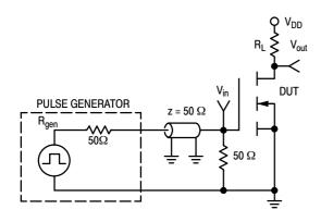
Figure 10. Switching Test Circuit
