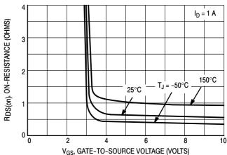
Figure 4. R<sub>DS(on)</sub> Variation With Gate-To-Source Voltage
