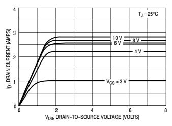
Figure 1. Output Characteristics
