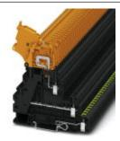
Disconnect terminal block, Connection method: Screw connection, Cross section: 0.14 mm²- 6 mm², AWG: 26 - 10, Nominal current: 28 A, Nominal voltage: 500 V, Width: 6.2 mm, Mounting type: NS 35/7,5, NS 35/15, Color: black
