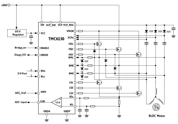
Figure 1.3 Application example for +24V DC
