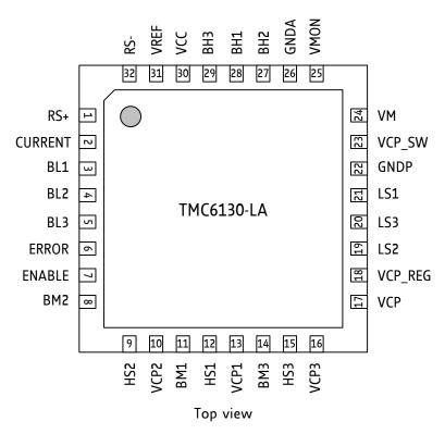
Figure 2.1 TMC6130 pin assignments
