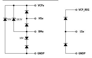
Figure 1.6 Gate driver connections
