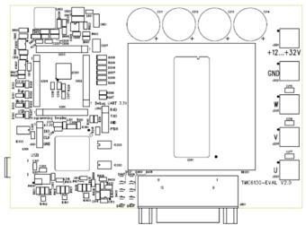
Layout with MOSFET power module (B6-bridge)
