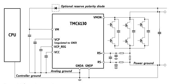
Figure 1.4 Ground connections
