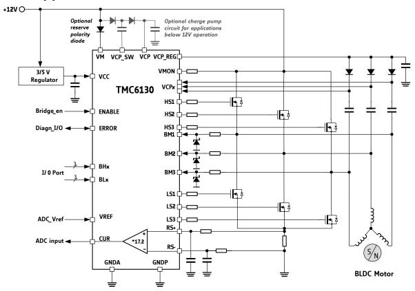
Figure 1.2 Application example for +12V DC
